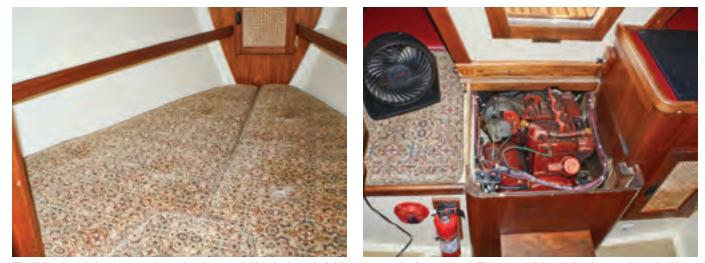
The V-berth, at left, measures just 6 feet long and, like the boat, is fairly narrow at its forward end. The cover of the engine box, at right, doubles as a companionway step and, when removed, provides access to the auxiliary engine, an Atomic 4.
