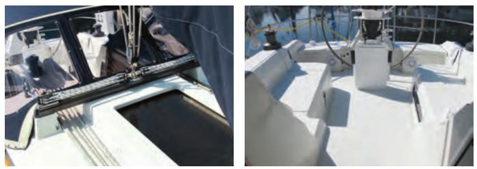
As one would expect on a high-performance boat, there are a lot of lines to tweak, and on *Intuitive* they are all led aft to the cockpit, at left. The C&C 34+ carries its beam well aft to increase offwind speed potential, but a drawback of having the cockpit use all that beam is that the cockpit seats are so far apart that average-size people have difficulty bracing their feet against the leeward seat, at right.
