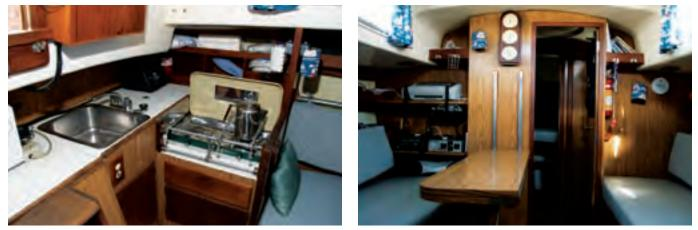
Good old test boat, *Tomfoolery*, has the "traditional" arrangement, in which the compact galley is laid out either side of the companionway, above left. In the saloon, settees facing each other across the dining table make good sea berths, above right. With the table stowed, access forward to the head and stateroom is much improved, below.
