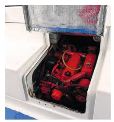
Access to the engine is very good. It's coupled to a retractable and steerable Sonic drive leg.
