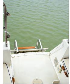
The companionway is protected by a bridge deck and the hatch slide by a sea hood, at left. It's also recessed into the cabin trunk, so it's tucked even farther under a dodger. The swim ladder, center, is attached to a panel in the transom that hinges down to provide easy access from the cockpit to the ladder, at right.
