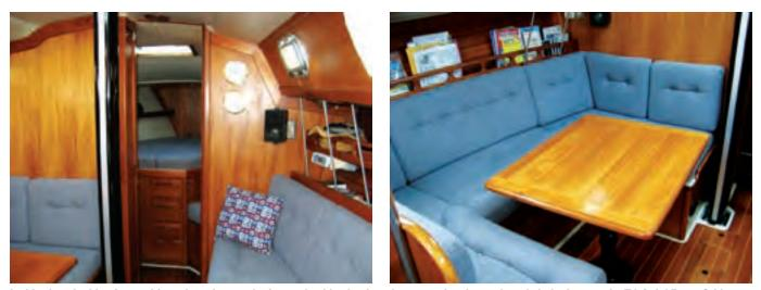
In this view, looking forward from the saloon to the forward cabin, the tie rods connecting the starboard chainplates to the Tri-Axial Force Grid are clearly visible, at left. The dinette table drops to make a 4-foot-wide double berth, at right. The cabin sole is teak-and-holly veneer-faced plywood.
