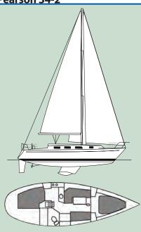
Designer: William Shaw 34 feet 6 inches LOA: LWL 28 feet 2 inches 11 feet 6 inches Beam: Draft: 4 feet 0 inches 11,800 pounds Displacement: 4,950 pounds Ballast: Sail area: 550 square feet Sail area/disp. ratio: 17.0 Disp./LWL ratio: 236 Fuel: 22 gallons Water: 70 gallons Holdina: 20 gallons Engine: 30-hp Yanmar diesel Air draft: 46 feet 8 inches
