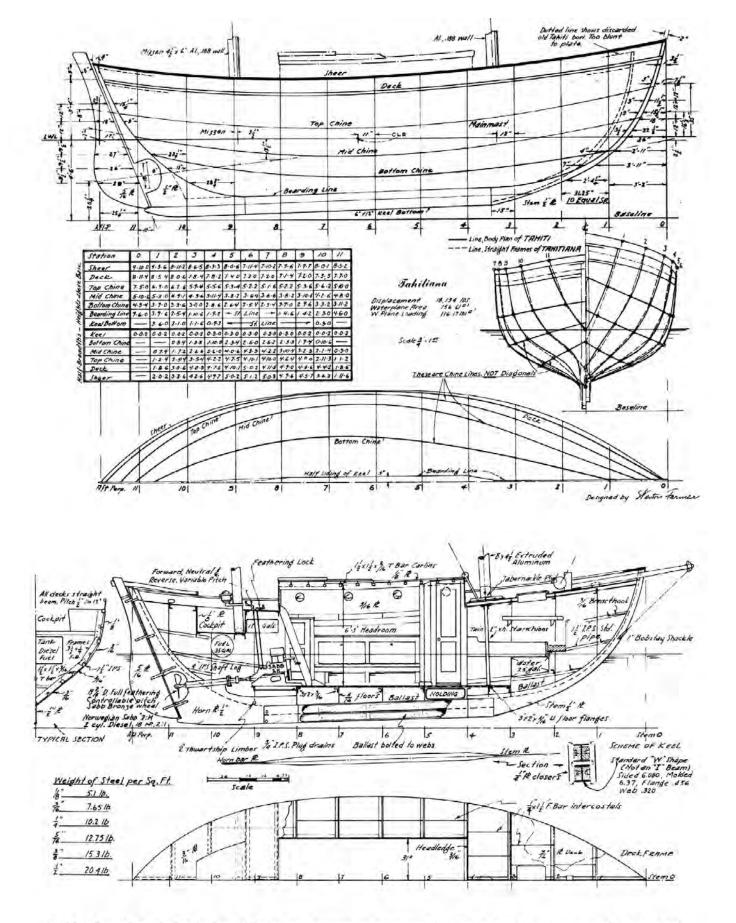
Tahitiana's profile, similar to that of Tahiti but somewhat enlarged, follows in steel the structure of the original, but with steel construction eight to ten times stronger than wood. Modern concessions include the holding tank and the 18-hp Sabb 2-H diesel with its full-feathering, controllable-pitch propeller for close-quarter maneuvering.
