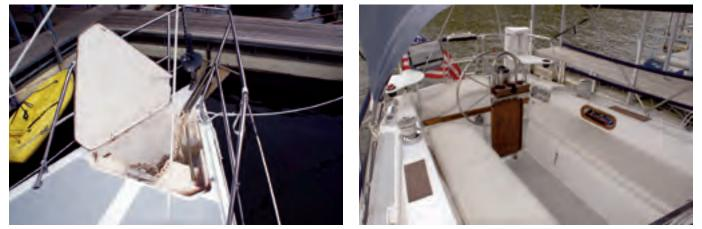
The anchor locker, at left, holds a second anchor and rode but makes fitting a windlass difficult. The T-shaped cockpit, at right, allows easy movement around the pedestal. Note the rudder head under the helm seat where it's accessible if there is a need to fit an emergency tiller.
