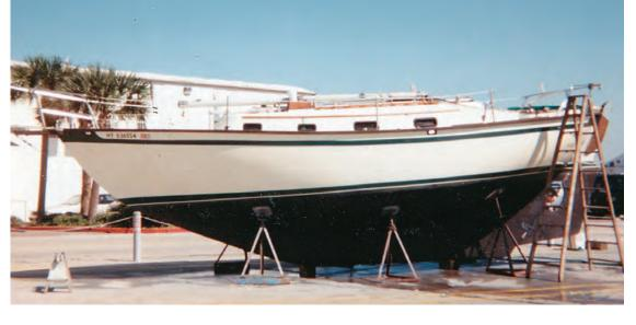
The boat's underwater profile, as we've already seen, is old-fashioned, well tested, and therefore greatly comforting to conservative cruisers. The outboard rudder is efficient and easy to get to if anything goes wrong.
