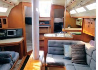
*Intuitive* has a three-burner stove with an oven and an electric refrigerator with a freezer compartment. Various storage compartments for food and cutlery add to the carefully planned and well-detailed cabin. A compact navigation station is opposite the galley and provides a comfortable place for the skipper to work, though the nav table is unsuitable for any but the smallest paper charts. A GPSMAP 4208, VHF, and AM/FM radio are close at hand.
