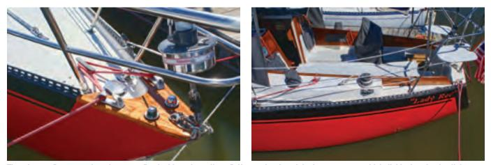
Though many Ranger 33s have been retrofitted with anchor rollers, *Drifter* retains the original arrangement, with individual navigation lights, two chocks, and a single cleat, at left. Teak coamings add a touch of elegance in the cockpit, at right, but do require some work if they are to be kept oiled or varnished. Primary and secondary winches and cleats on the cockpit coamings reflect the boat's age and its racing origins.
