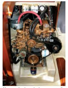
After removing the engine box, access to all sides of the engine is very good. Jerry added sound insulation, which greatly reduced engine noise on deck and below.
