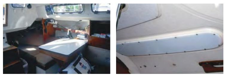
At left above, forward-facing navigation station, and at right, one of the many overhead panels giving access to deck hardware.
