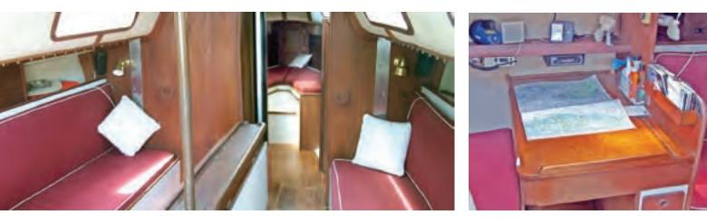
The saloon, at left, is fairly straightforward with opposing settees and a drop-leaf table on centerline. The centerboard pendant runs through the pipe, which also functions as a handhold. Note the massive chainplates through-bolted to the main bulkhead; check underneath for rot, a common problem on older boats. Chart work is done on a dedicated nav table, at right, at the head of the port quarter berth. This is a nice feature that keeps charts, pencils, and rules off the dining table.
