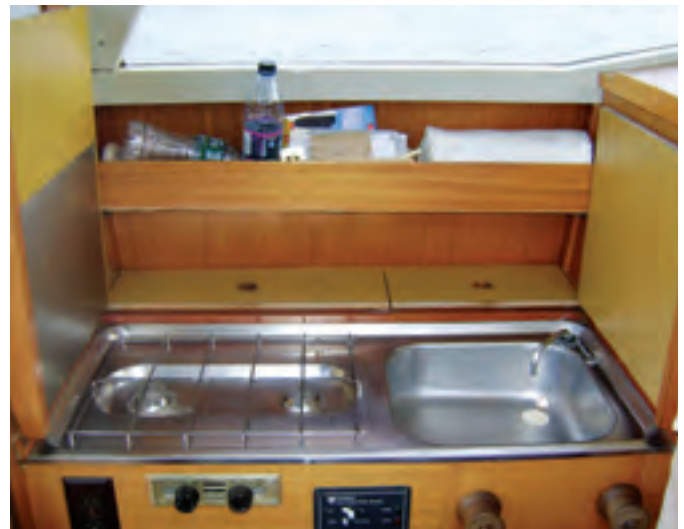
The port side of the pilothouse is both nav station, at left, and galley, at right. When it's the cook's turn to use this space, the leaves of the chart table open to reveal a sink with hot and cold running water and a stove.
