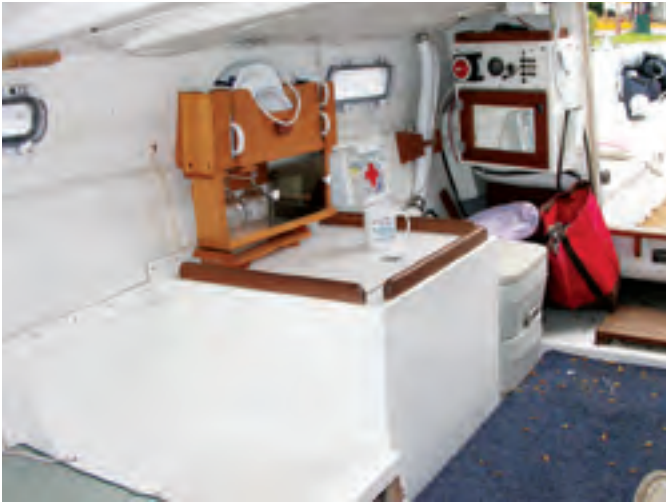
Placing the portable toilet next to the galley is bad feng shui , but that's life aboard a camping cruiser. The molded fiberglass seat forward of the icebox is nicely contoured, at left. The interior is simple and utilitarian, but with the board folded down and the center cushion in place, a sailing couple has a comfy queen-sized berth, at right. Note the platform forward for standing on when handling the jib or ground tackle.
