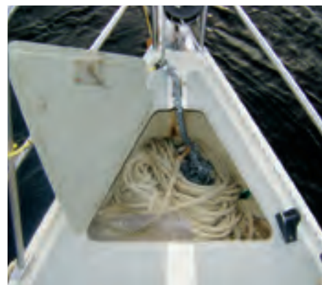
The anchor well is easy to access and keeps the anchor stored out of the way when not in use.
