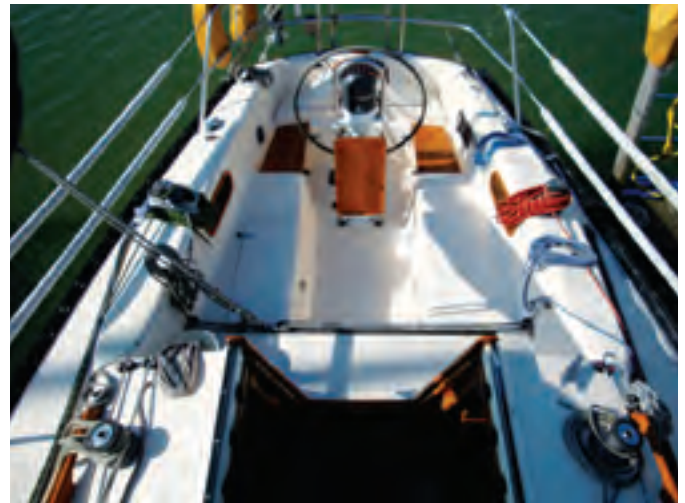
A factory option was to have the shorepower connection, the waste-discharge port, and the water-tank fill fitted in the anchor well, at left above. The short cockpit seats can be extended by inserting boards aft, though this restricts movement around the pedestal, at right above.
