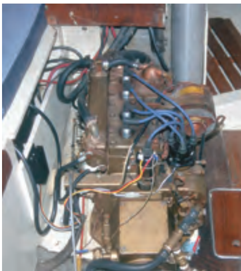
The Atomic 4, at left, has marvelous access in the cabin amidships under the short piece of the L-shaped settee. The Tartan builder's plate, above. The Tartan 30 under sail, below left.
