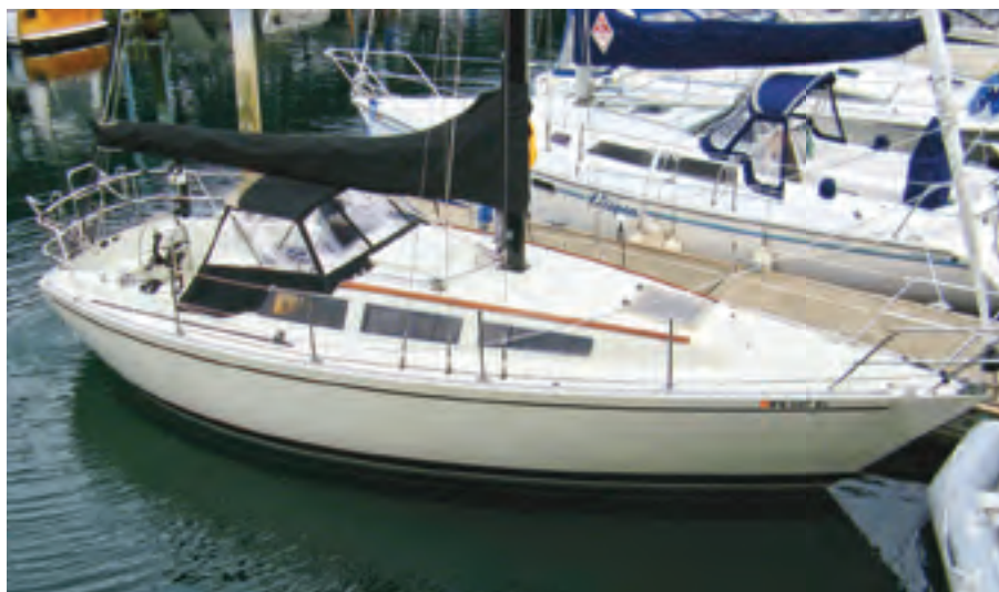
This view of Greg Pearson's well-maintained S2 9.2A, above, shows some of her key deck features. Note the sea hood over the companionway sliding hatch, continuous teak grabrail, narrow foredeck, double lifelines, and double lower shrouds terminating near the rail.
