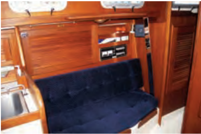
The port-side saloon settee is short, to allow room for the galley. Above the settee, the outboard locker door swings down to become a chart table. The fiddled shelf holds the navigator's tools and John Ollila has installed a VHF radio in the locker. The switch panel is forward of this nav center.
