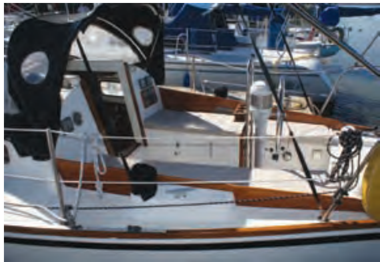
Part of the Bristol 29.9's appeal is its uncluttered deck, at left. The cockpit, above, is conventional, with seats just over 6 feet long and teak coamings that provide decent back support forward.
