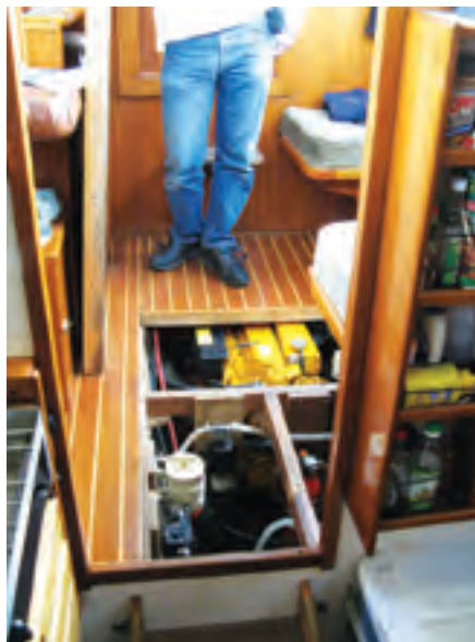
The engine and other systems are under the pilothouse sole and quite accessible.
