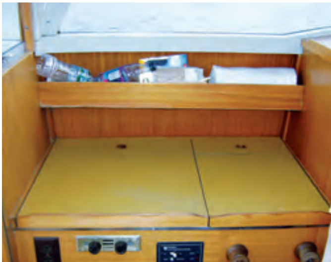
The port side of the pilothouse is both nav station, at left, and galley, at right. When it's the cook's turn to use this space, the leaves of the chart table open to reveal a sink with hot and cold running water and a stove.
