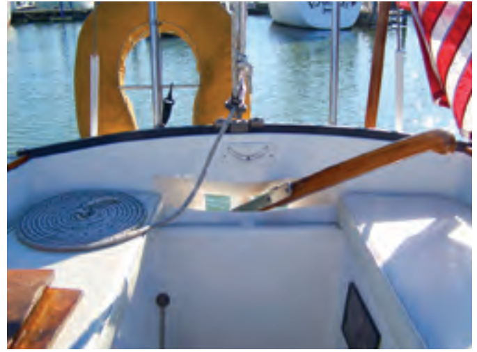
At nearly 7 feet long, the cockpit in the Aloha 8.5 has lots of room for boat handling and relaxing, at left. The tiller passes through the transom, at right, allowing the mainsheet to be attached to a traveler running across the top of the cockpit coaming. The forward hatch is on the foredeck, below, leaving the cabintop clear of obstructions forward of the mast.
