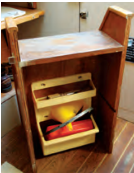
Clever use of the inside of the companionway steps creates useful stowage space, at left above. The step unit can be detached to provide access to the engine, at right above.
