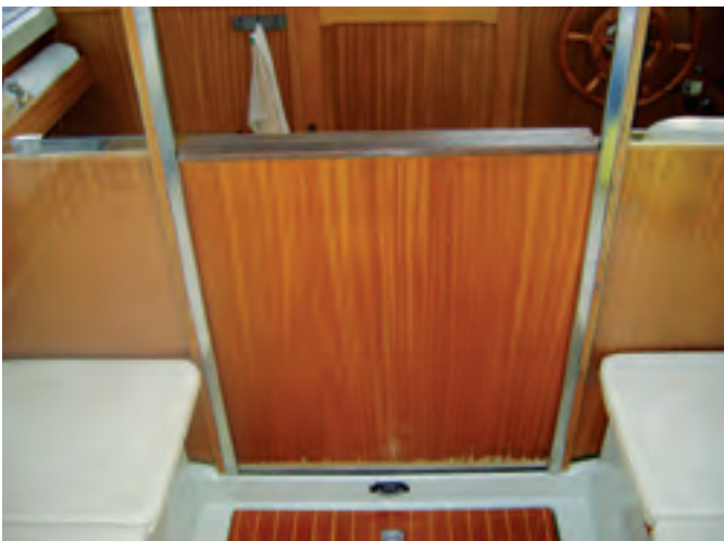
Instead of dropboards, the cockpit is sealed off from the pilothouse by this innovative door that pulls up from a pocket in the bulkhead where it is stowed out of the way, at left. Larry installed extra custom handholds to give him more security when going forward, at right. Note the sliding hatch over the helm seat and the cockpit awning folded away just behind the pilothouse.
