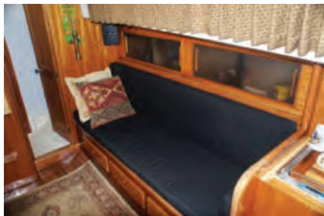
Somewhat unusual in a 30-footer is the dedicated chart table, at left, which uses the head of the quarter berth for a seat. The drawers beneath the starboard settee and the cabinets outboard, at right, are typical of the handsome joiner work found on Bristol yachts.
