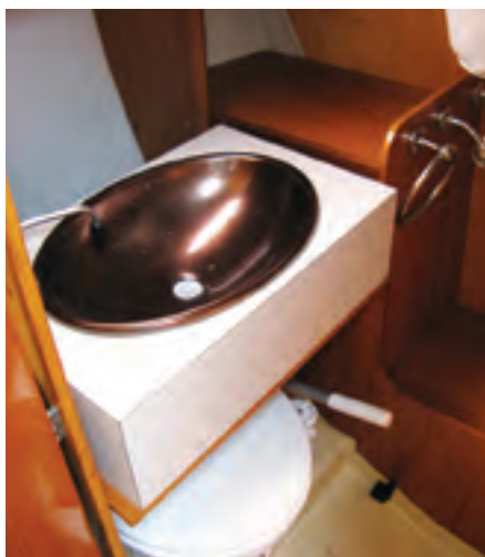
In the head, a hinged sink folds down over the toilet to make the most of a compact space, at left. The engine compartment, under the companionway ladder, is tight, center, but access to most service points is adequate except for the dipstick. To increase space for food preparation, the galley has a hinged counter over the French-made stove, at right. In the 1980s, boats imported into the U.S. weren't "Americanized."
