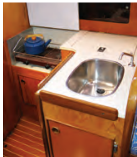
In the head, a hinged sink folds down over the toilet to make the most of a compact space, at left. The engine compartment, under the companionway ladder, is tight, center, but access to most service points is adequate except for the dipstick. To increase space for food preparation, the galley has a hinged counter over the French-made stove, at right. In the 1980s, boats imported into the U.S. weren't "Americanized."
