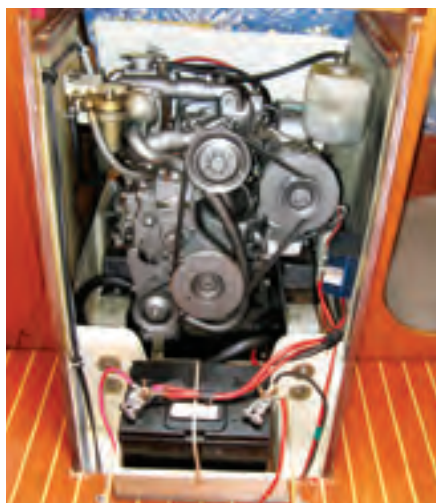
In the head, a hinged sink folds down over the toilet to make the most of a compact space, at left. The engine compartment, under the companionway ladder, is tight, center, but access to most service points is adequate except for the dipstick. To increase space for food preparation, the galley has a hinged counter over the French-made stove, at right. In the 1980s, boats imported into the U.S. weren't "Americanized."
