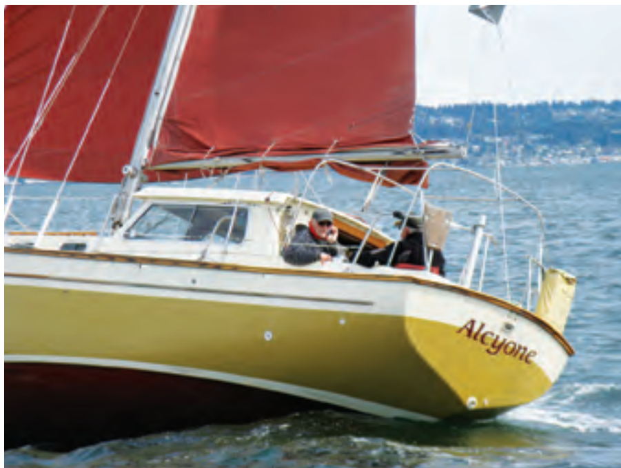
Its high freeboard and relatively narrow beam combine to make the Rawson 30 initially tender. That freeboard and the pilothouse help keep things dry in the cockpit.
