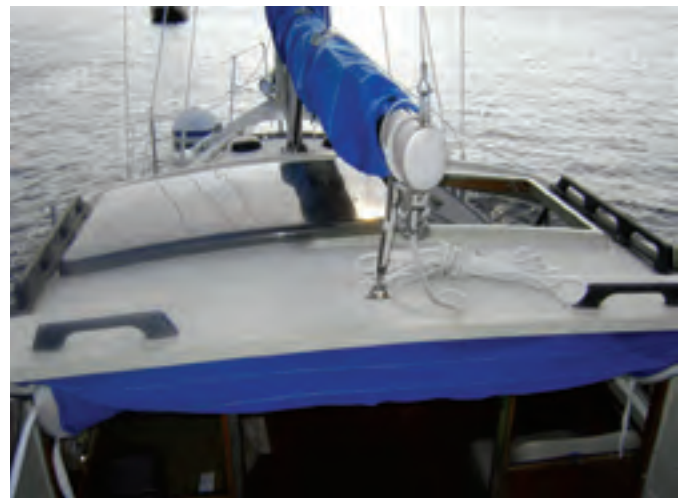
Instead of dropboards, the cockpit is sealed off from the pilothouse by this innovative door that pulls up from a pocket in the bulkhead where it is stowed out of the way, at left. Larry installed extra custom handholds to give him more security when going forward, at right. Note the sliding hatch over the helm seat and the cockpit awning folded away just behind the pilothouse.
