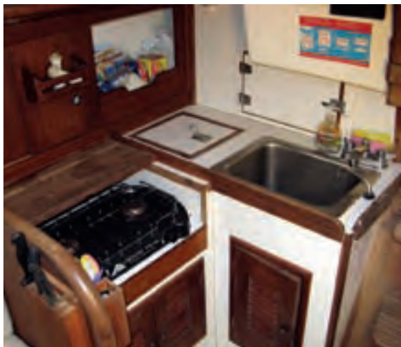
The galley is laid out reasonably well, given the limited space in a 30-foot boat, but the sink is partially tucked under the cockpit, which hampers leaning over it to work.
