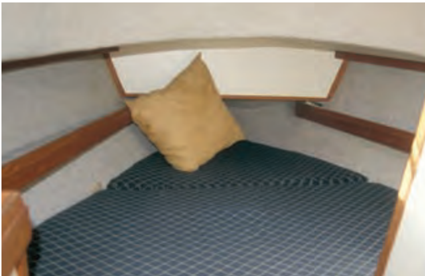
Facing page: The galley is compact, to be sure; the icebox is poorly insulated. A flip-up counter extension increases space for food preparation, at left. The dinette table folds down from the main bulkhead and comfortably seats four, at right. This page: The V-berth cushion is split athwartships for easier access to the locker underneath.
