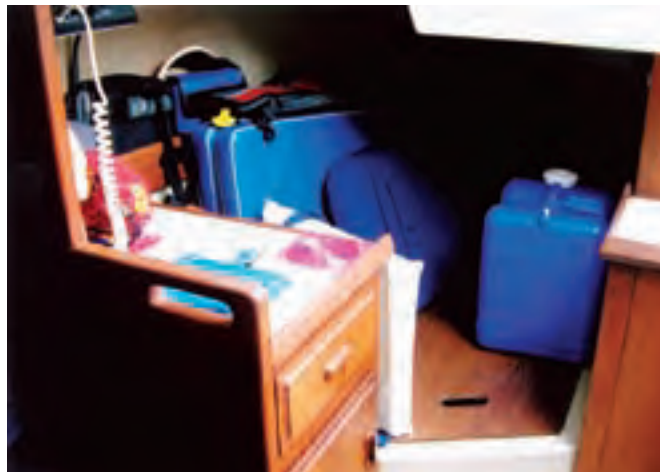
Liza 's quarter berth has been converted by David and Mary Lucas to bulk storage. The cabinet in front has a lift-up leaf that converts it to a small chart table.
