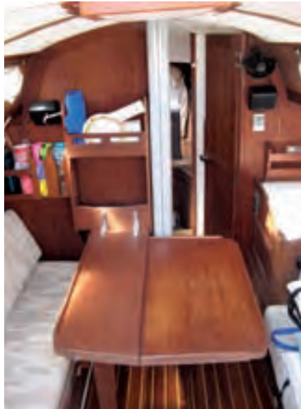
The port settee, at left, extends to make a double berth. Above it is open-shelf and cabinet storage. The 40-gallon water tank is beneath. The navigation station, at right, located in the port quarter area, is well designed and large for a boat this size. The dining table, below, is good sized and folds in half for stowage vertically against the bulkhead when not in use.
