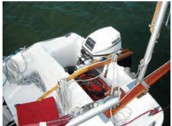
The hatches are intended to eliminate walking on the deck; Gayle Scheuer emerges from the forward hatch, at left, to tend the mooring line at a raft-up. The stern of a Shearwater 28, at right, is a busy place, with outboard, fuel tank, boomkin, mizzen mast, mizzen sheet, main sheet, rudder, and control lines for the rudder's kick-up mechanism.
