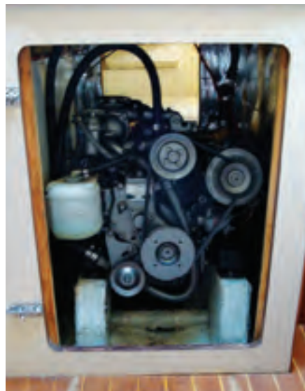
Clever use of the inside of the companionway steps creates useful stowage space, at left above. The step unit can be detached to provide access to the engine, at right above.
