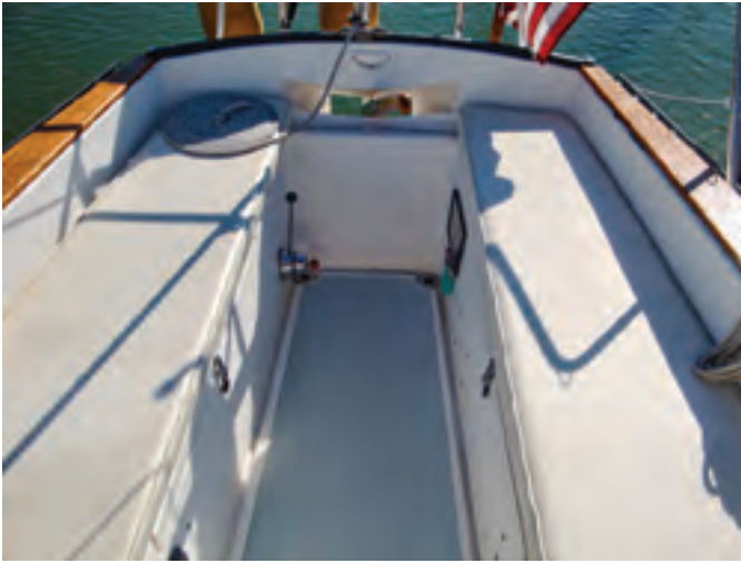
At nearly 7 feet long, the cockpit in the Aloha 8.5 has lots of room for boat handling and relaxing, at left. The tiller passes through the transom, at right, allowing the mainsheet to be attached to a traveler running across the top of the cockpit coaming. The forward hatch is on the foredeck, below, leaving the cabintop clear of obstructions forward of the mast.
