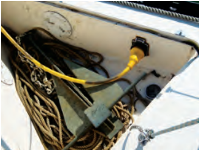
A factory option was to have the shorepower connection, the waste-discharge port, and the water-tank fill fitted in the anchor well, at left above. The short cockpit seats can be extended by inserting boards aft, though this restricts movement around the pedestal, at right above.
