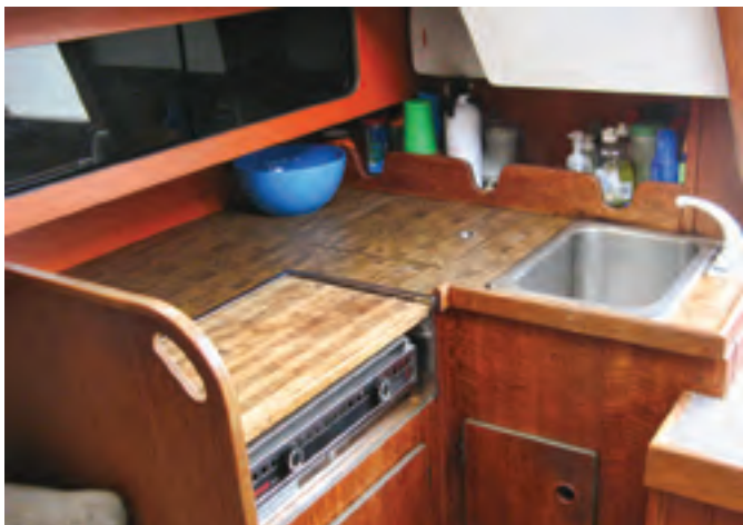
The compact galley, at left, is fitted out with an Origo alcohol stove, a small sink, and an icebox. The nav desk, at right, is cleverly designed to lift up and out for use. It is stowed against the hull and a cushion takes its place when the quarter berth is needed.
