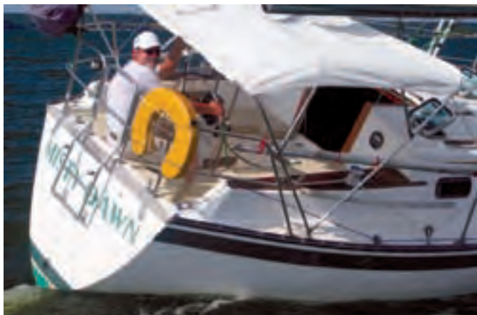
The cockpit of the Caliber 28, at left, feels very secure with its stern rail, high coamings, and bridge deck. The foredeck, at right, is unobstructed, and the hatch to the very large anchor locker takes up most of it.
