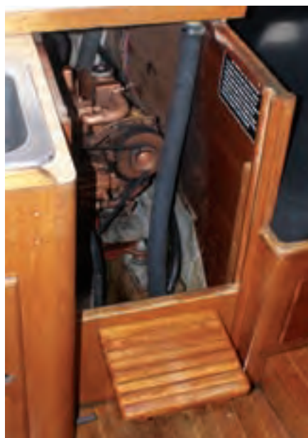
Access to the engine is not very good. Removing the companionway steps reveals the alternator, at left, but the oil dipstick can only be reached through the starboard cockpit locker. As expected on a 30-footer, the head is small, at right, but it is well provided with storage spaces.
