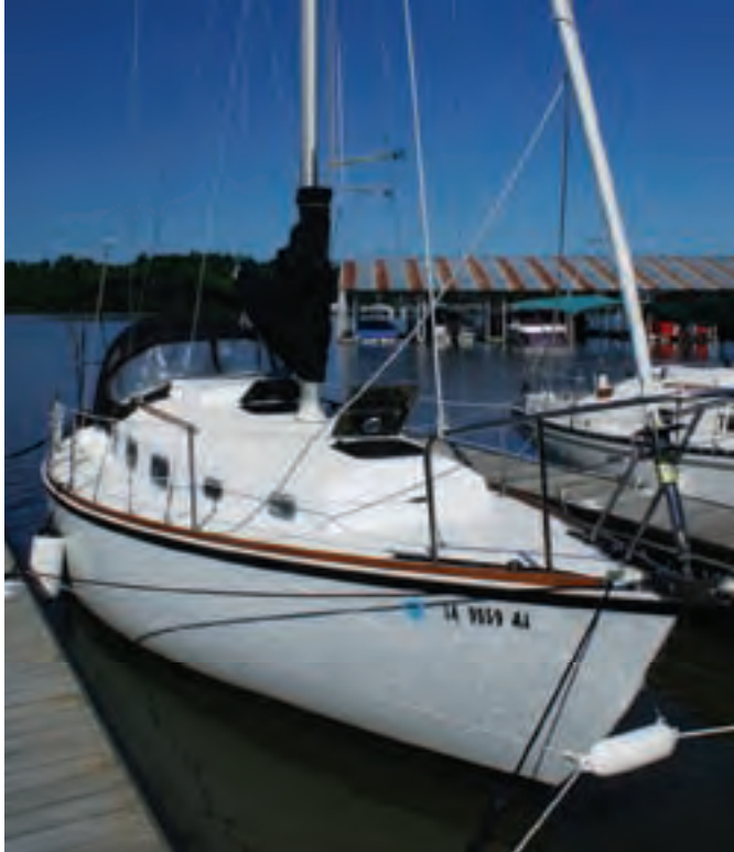
Part of the Bristol 29.9's appeal is its uncluttered deck, at left. The cockpit, above, is conventional, with seats just over 6 feet long and teak coamings that provide decent back support forward.
