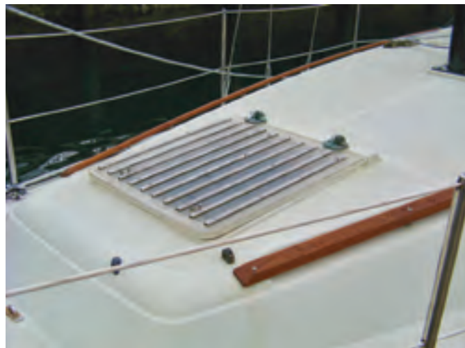
At the bow there is a small anchor locker, two cleats, and a tiny roller for handling ground tackle, at left. The forward hatch, at right, located on the coachroof above the entrance to the forward cabin, is a little too far aft to bring much breeze to crew sleeping on the V-berth.
