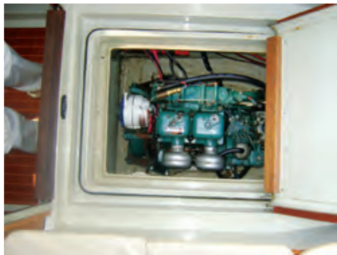
The saloon is a comfortable place to unwind after a long day on the water, at left. Safina's 28-hp Volvo Penta diesel engine is mounted beneath the cockpit sole. The spacious engine room and large hatch allow the engine to be easily inspected and maintained, at right.
