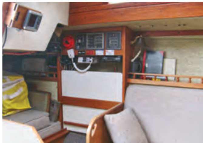
The compact galley, at left, is fitted out with an Origo alcohol stove, a small sink, and an icebox. The nav desk, at right, is cleverly designed to lift up and out for use. It is stowed against the hull and a cushion takes its place when the quarter berth is needed.
