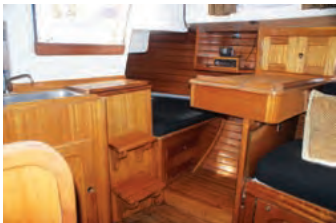
Somewhat unusual in a 30-footer is the dedicated chart table, at left, which uses the head of the quarter berth for a seat. The drawers beneath the starboard settee and the cabinets outboard, at right, are typical of the handsome joiner work found on Bristol yachts.
