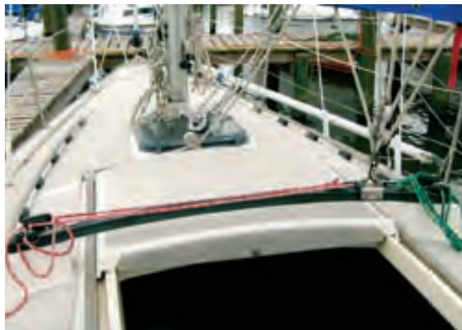
Sunshine's traveler, with line control, makes for easy mainsail shaping when racing.
