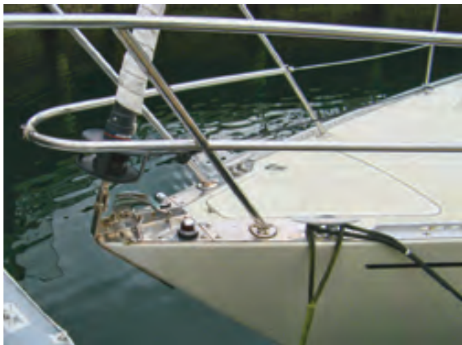
At the bow there is a small anchor locker, two cleats, and a tiny roller for handling ground tackle, at left. The forward hatch, at right, located on the coachroof above the entrance to the forward cabin, is a little too far aft to bring much breeze to crew sleeping on the V-berth.
