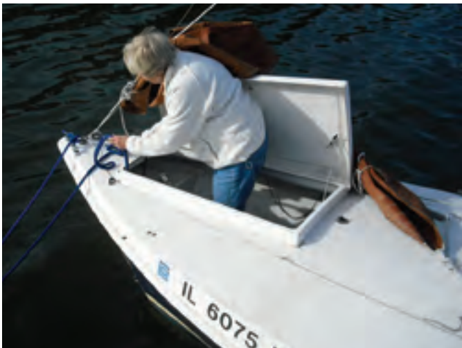
The hatches are intended to eliminate walking on the deck; Gayle Scheuer emerges from the forward hatch, at left, to tend the mooring line at a raft-up. The stern of a Shearwater 28, at right, is a busy place, with outboard, fuel tank, boomkin, mizzen mast, mizzen sheet, main sheet, rudder, and control lines for the rudder's kick-up mechanism.
