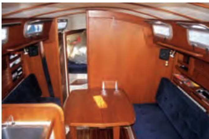
This view from the companionway shows the bulkhead-mounted table set up for use, at left. The U-shaped galley is quite complete for a 28-footer with stovetop, sink, icebox, and more-than-expected stowage, at right. High-quality joinerwork is evident throughout the boat.
