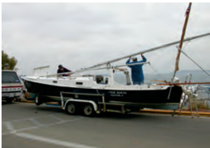
The mast can be lowered under way, to duck under a bridge. The procedure is even easier on land and can be done by one person, but two always helps, at left. True North motoring toward the beach with her dinghy, Due South , near the shore of Kentucky Lake, at right.
