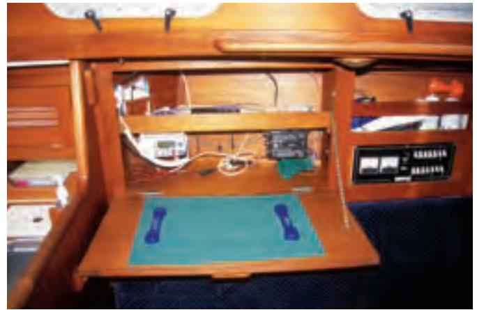
The port-side saloon settee is short, to allow room for the galley. Above the settee, the outboard locker door swings down to become a chart table. The fiddled shelf holds the navigator's tools and John Ollila has installed a VHF radio in the locker. The switch panel is forward of this nav center.
