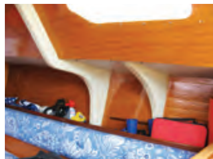
The navigation station, aft of the saloon on the starboard side, is large and very workable for a boat of this size, at left. Beams and knees stiffen the deck and anchor the chainplates, at right.
