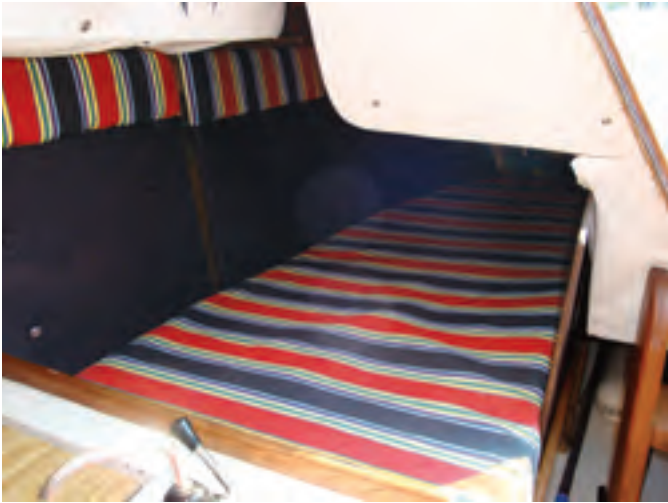
The quarter berths under the cockpit seats, above, are a little wider than the settees in the saloon. By recessing the cabin sole into the keel, Lancer gave this low-profile boat nearly 6 feet of standing headroom, at right. Behind the ladder is a large space for stowing bulky items. The bottom step hinges up to reveal the bilge pump.
