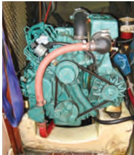
Portions of the hull liners that make up the cabin sole foundation, berth foundations, and hull sides are visible in the forward part of the boat, above. Dufour used extensive and quite intricate internal liners, as a detail of the saloon overhead shows, below right. Papillon was repowered with a 3-cylinder Volvo Penta diesel, below left, and access to it is quite good.
