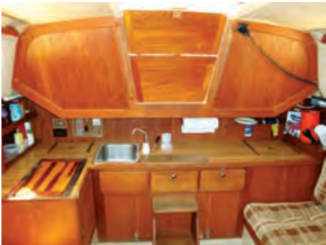
The galley, at left, extends athwartships under the bridge deck, so one of the steps used when entering or leaving the cabin is in the middle of the counter. In spite of this, it's an efficient use of space in a small boat. Most Cal boats have fiberglass pans or inner liners that form the sole and berth flats and include an athwartships beam that supports the mast's compression post. The interior is finished in teak-veneer plywood.
