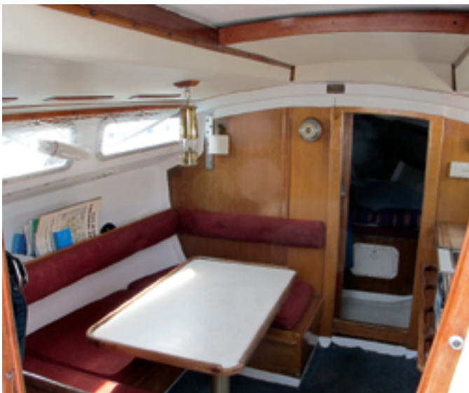
The table drops to make a double berth, at left. Removing the wooden strips in the overhead provides access to the nuts and bolts that secure deck hardware. The starboard-side galley, above, includes a two-burner stovetop, sink, drawers, lockers down low, and outboard stowage for sundry items. A common upgrade for do-it-yourselfers is a swing-out arm for critical instruments like a depth sounder and GPS.
