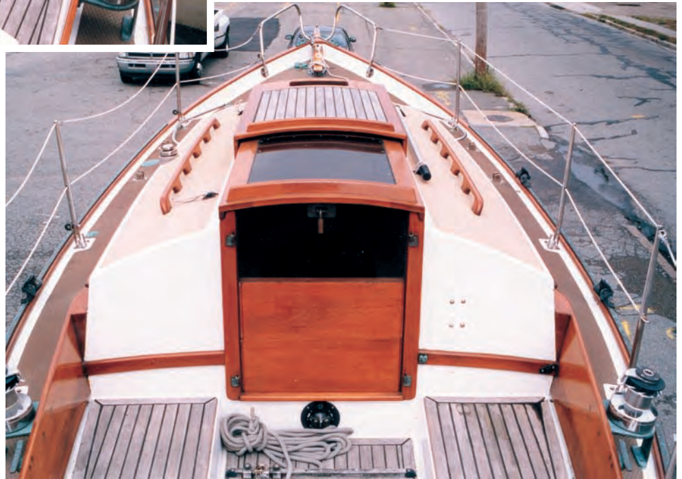
The Ezzells' Blackberry is almost as pretty out of the water as she is in her element. Notice the aft samson post at left, the aft lazarette, and the tiller sweep. The mainsheet attaches to the bridgedeck, center. At bottom, Blackberry , previously known as the Pearla B , shows off her Chuck Paine lines.
