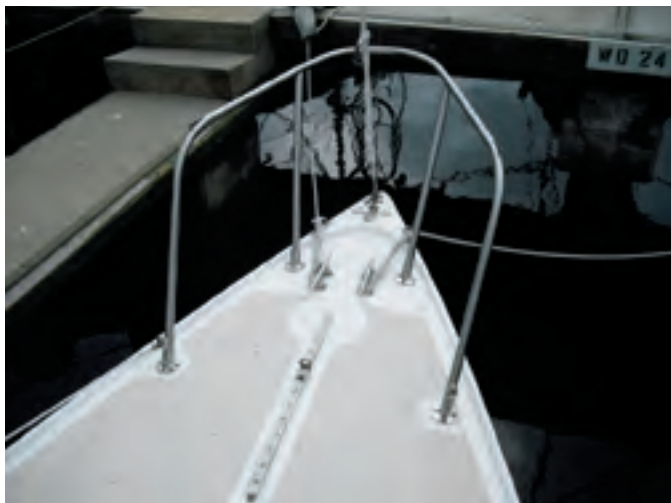
The foredeck of the Morgan 25 is uncluttered and the lifelines terminate low on the pulpit so the foot of the genoa can clear them, at left. The 8-foot cockpit can seat a crowd and the coamings provide plenty of back support, at right.
