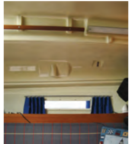
Portions of the hull liners that make up the cabin sole foundation, berth foundations, and hull sides are visible in the forward part of the boat, above. Dufour used extensive and quite intricate internal liners, as a detail of the saloon overhead shows, below right. Papillon was repowered with a 3-cylinder Volvo Penta diesel, below left, and access to it is quite good.
