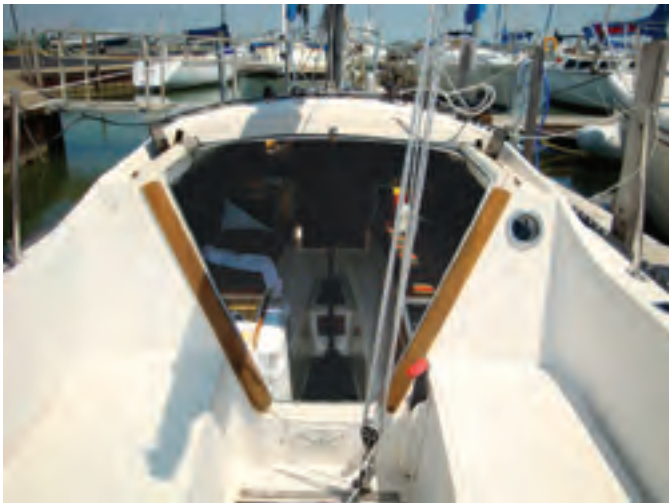
The wide companionway makes for easy egress, but you have to get by the mainsheet tackle first, at left. The cockpit coamings are sufficiently high to provide decent back support. The gas tank for the outboard motor is in the lazarette aft of the tiller, at right.
