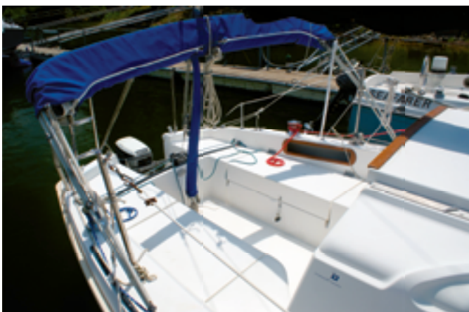
The roomy cockpit, at left, comfortably seats four. Seat lockers and coaming cubbies provide plenty of stowage. The foredeck, at right, has few obstructions while providing the basic necessary hardware: chocks, cleats, and running lights.
