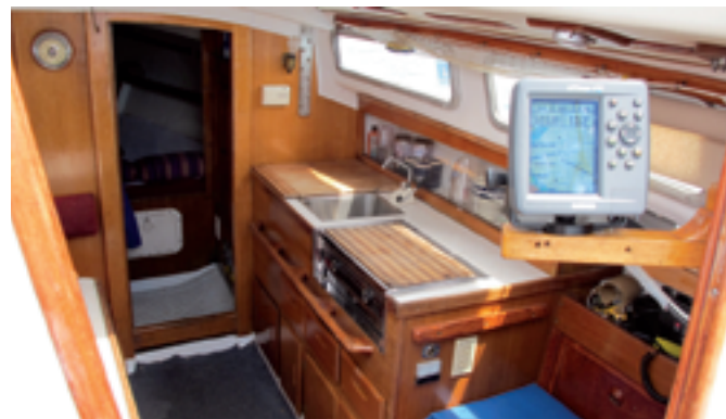
The table drops to make a double berth, at left. Removing the wooden strips in the overhead provides access to the nuts and bolts that secure deck hardware. The starboard-side galley, above, includes a two-burner stovetop, sink, drawers, lockers down low, and outboard stowage for sundry items. A common upgrade for do-it-yourselfers is a swing-out arm for critical instruments like a depth sounder and GPS.
