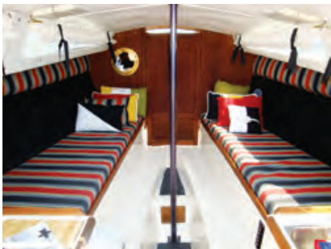
Bump-A-Noggin has a bright interior thanks to reupholstered settee cushions. The compression post for the mast is dead center, at left. Forward, the head compartment has vanities port and starboard, with the sink in the starboard one, and a portable toilet is normally between them, at right.
