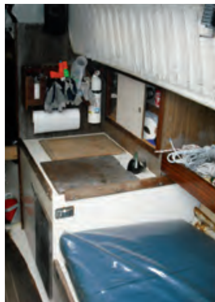
Amanda has the standard layout for a Morgan 24. A V-berth (here filled with sails) occupies the bow, at left. The galley is forward in the saloon and the settees extend under the cockpit as quarter berths, at right.
