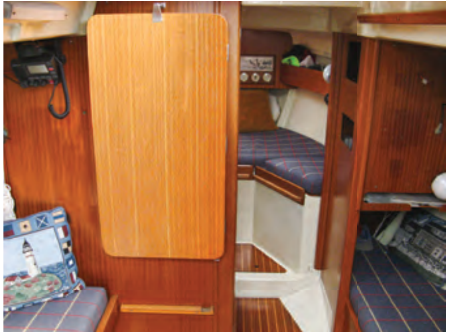
Portions of the hull liners that make up the cabin sole foundation, berth foundations, and hull sides are visible in the forward part of the boat, above. Dufour used extensive and quite intricate internal liners, as a detail of the saloon overhead shows, below right. Papillon was repowered with a 3-cylinder Volvo Penta diesel, below left, and access to it is quite good.
