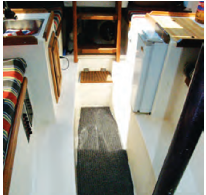
The quarter berths under the cockpit seats, above, are a little wider than the settees in the saloon. By recessing the cabin sole into the keel, Lancer gave this low-profile boat nearly 6 feet of standing headroom, at right. Behind the ladder is a large space for stowing bulky items. The bottom step hinges up to reveal the bilge pump.
