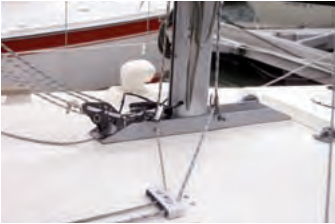
The mast is stepped on a shoe. By tightening and loosening the forestay and backstay, the mast's rake can be adjusted slightly forward or aft to correct weather or lee helm.
