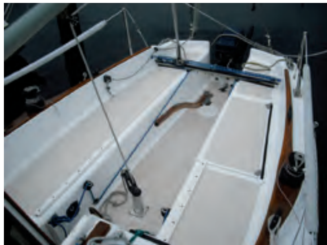
The foredeck of the Morgan 25 is uncluttered and the lifelines terminate low on the pulpit so the foot of the genoa can clear them, at left. The 8-foot cockpit can seat a crowd and the coamings provide plenty of back support, at right.
