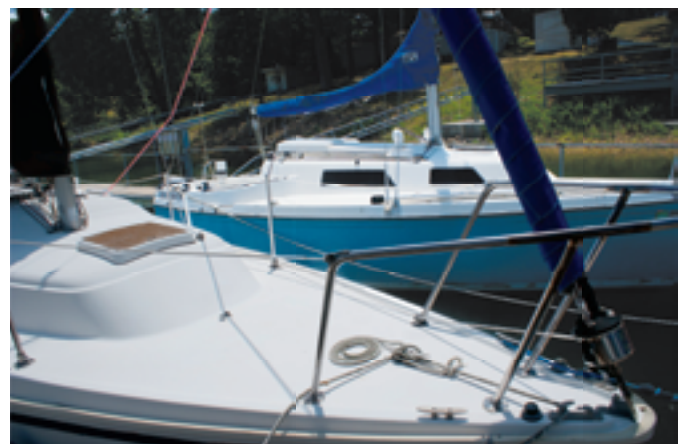
The roomy cockpit, at left, comfortably seats four. Seat lockers and coaming cubbies provide plenty of stowage. The foredeck, at right, has few obstructions while providing the basic necessary hardware: chocks, cleats, and running lights.
