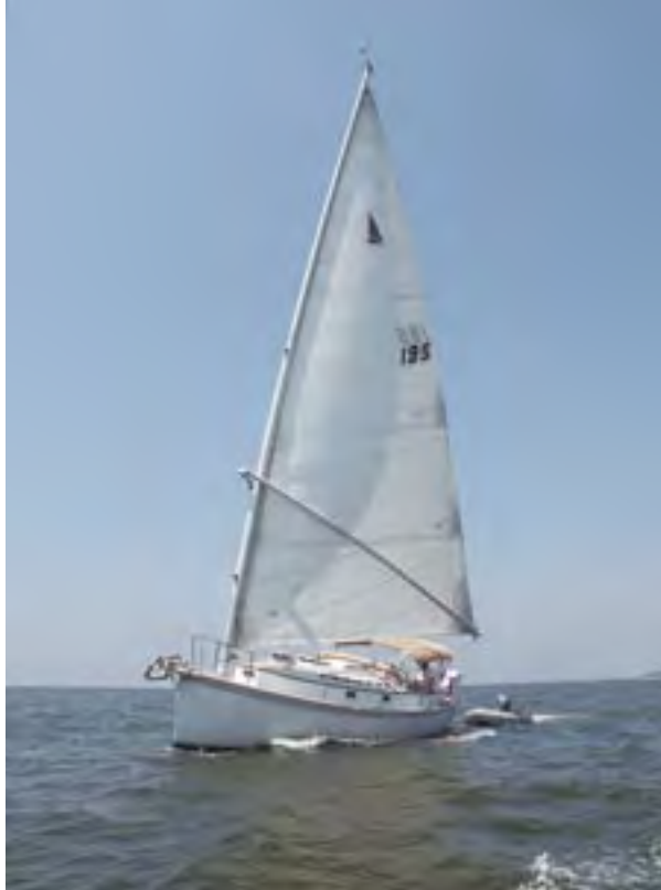
Pelican's unstayed mast, above, is very flexible, bending to leeward in the puffs spilling wind from the sail. An overview of the Classic Nonsuch layout, below.
