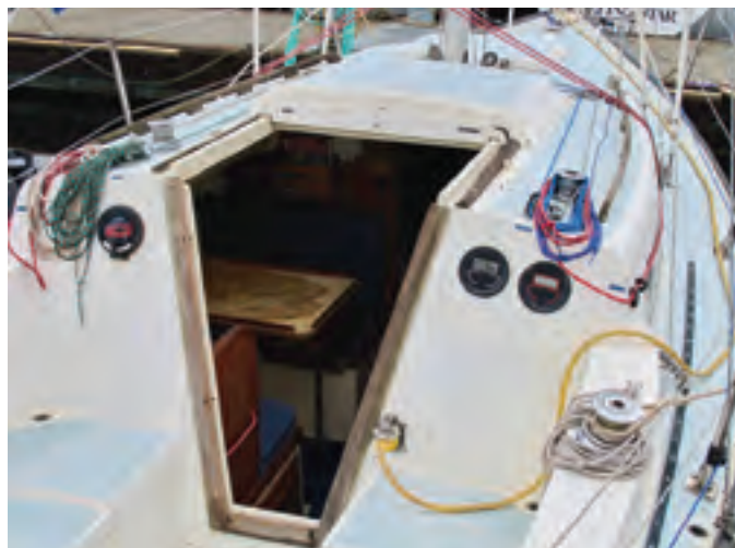
The companionway has a low sill for easy ingress and egress, at left, but in rough conditions the bottom weather board should be locked in place. The red lines running along the cabin sides are part of Dave Gow's boom vang/preventer system. The cockpit has high coamings for comfortable backrests, at right. Dave says the 8-hp outboard has always been more than adequate power, even against Puget Sound's notorious currents.
