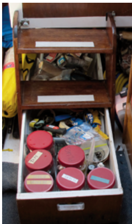
A very, very long storage drawer is fitted under the companionway ladder and cockpit.
