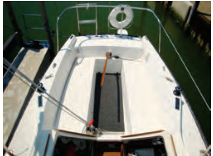
The wide companionway makes for easy egress, but you have to get by the mainsheet tackle first, at left. The cockpit coamings are sufficiently high to provide decent back support. The gas tank for the outboard motor is in the lazarette aft of the tiller, at right.
