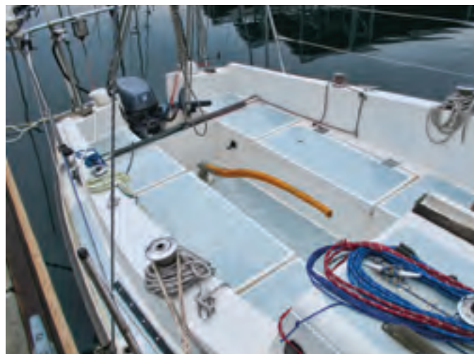
The companionway has a low sill for easy ingress and egress, at left, but in rough conditions the bottom weather board should be locked in place. The red lines running along the cabin sides are part of Dave Gow's boom vang/preventer system. The cockpit has high coamings for comfortable backrests, at right. Dave says the 8-hp outboard has always been more than adequate power, even against Puget Sound's notorious currents.
