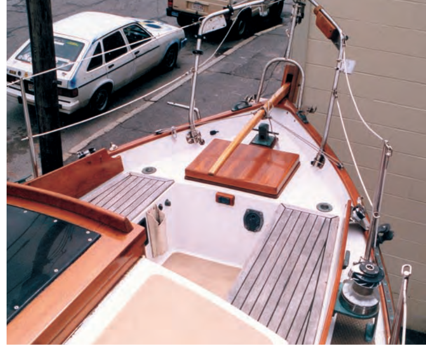
The Ezzells' Blackberry is almost as pretty out of the water as she is in her element. Notice the aft samson post at left, the aft lazarette, and the tiller sweep. The mainsheet attaches to the bridgedeck, center. At bottom, Blackberry , previously known as the Pearla B , shows off her Chuck Paine lines.
