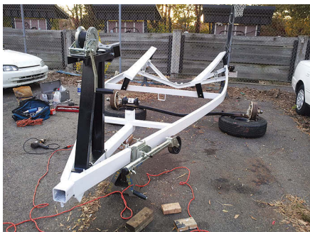
As the restoration progressed, the trailer began to sport new paint and sprout new parts, at left. The new Titan 10- by 2¼-inch free-backing drum-brake assemblies await the new rims and tires, center. Complete with bunk carpeting, the trailer is ready for hauling duty at the marina, at right.
