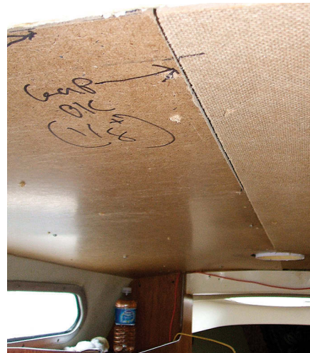
Ken used scrap lumber to hold pieces of the old overhead liner in place while the adhesive set, at left. Using tick stick marks and a flexible batten, he drew the shapes of the new overhead liner on hardboard, center, then screwed the hardboard patterns in place and marked them for trimming, at right.
