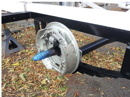
As the restoration progressed, the trailer began to sport new paint and sprout new parts, at left. The new Titan 10- by 2¼-inch free-backing drum-brake assemblies await the new rims and tires, center. Complete with bunk carpeting, the trailer is ready for hauling duty at the marina, at right.
