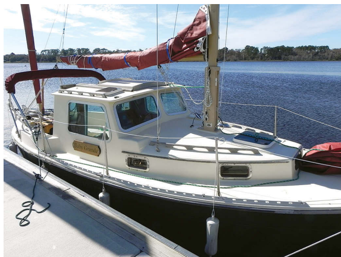
On the Nimble Arctic 25, the mast is stepped in a tabernacle, which allows it to be lowered fairly easily, even to duck under bridges.
