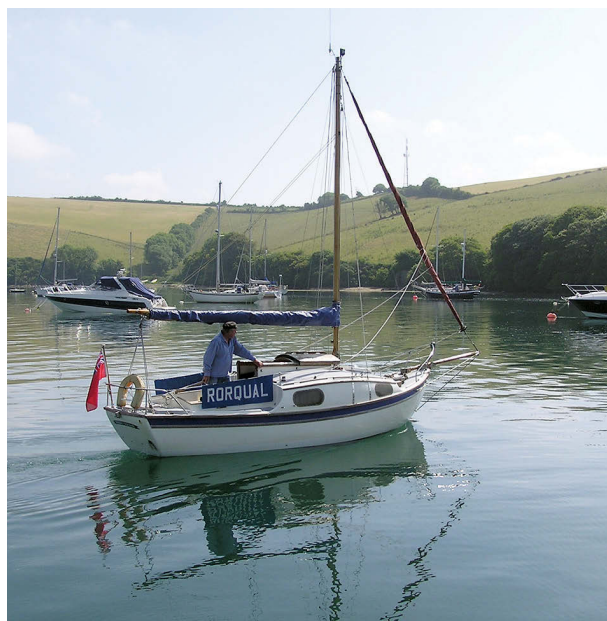
One of Denys Rayner's earliest designs in fiberglass was the Westerly 22, at left, which had a gunter rig, for easy singlehanded, and generous headroom. The Laurent Giles-designed Westerly Centaur, above and facing page, has the bilge keels that allow so many Westerlys to take the ground in tidal estuaries.
