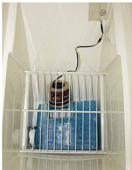
Clarence solved the problem of ice melt in his icebox by making a special cold-melting ice in plastic containers, at left. This also solved the problem of losing “cold energy” when the melted ice drained away. A portable fan housed in a plastic tub circulates the cold air.
