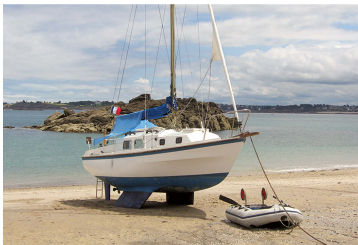
One of Denys Rayner's earliest designs in fiberglass was the Westerly 22, at left, which had a gunter rig, for easy singlehanded, and generous headroom. The Laurent Giles-designed Westerly Centaur, above and facing page, has the bilge keels that allow so many Westerlys to take the ground in tidal estuaries.
