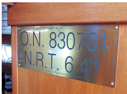
Del Viento , a U.S. documented vessel, upper right, has her official number secured to the interior structure, at right. A similar requirement applies to a Canadian vessel, at left.
