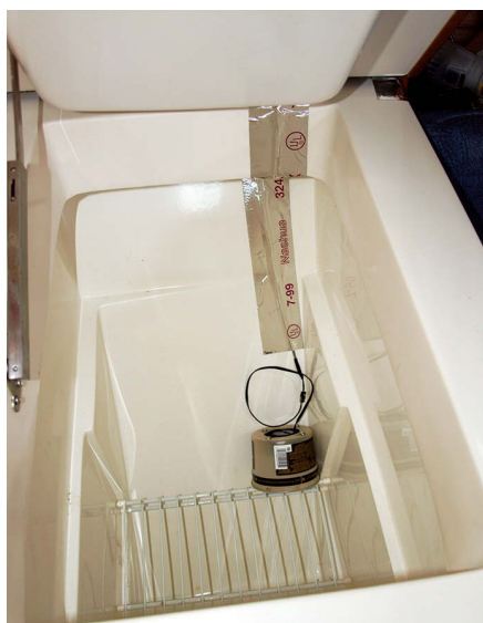
Clarence solved the problem of ice melt in his icebox by making a special cold-melting ice in plastic containers, at left. This also solved the problem of losing “cold energy” when the melted ice drained away. A portable fan housed in a plastic tub circulates the cold air.
