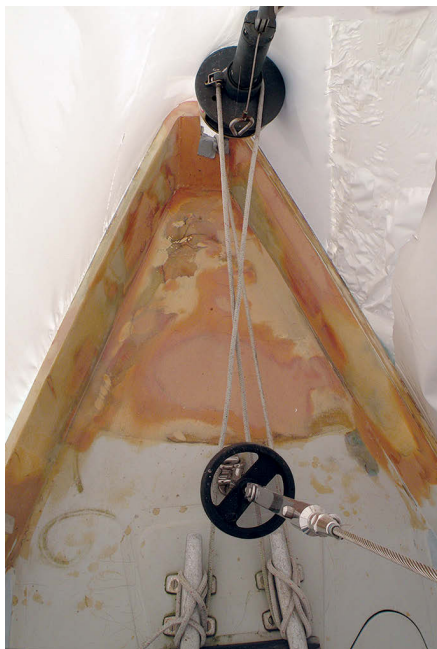
Under the winter cover, a new section of bulwark and deck core are in place and ready for finishing, at left. The bow section has been re-cored and faired and is ready for primer, center. The first area where the repair was completed was at the bow, at right.
