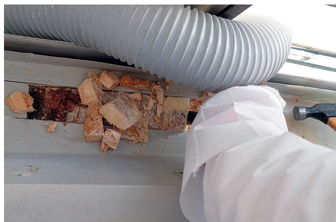
Because of the way the deck was joined to the hull, Steve had to cut into the bulwark, at left. The deck skin also had to be cut out to expose the saturated balsa core. Mary removed the rotten core with hammer and chisel, at right. The white hose is part of the dust collection system.
