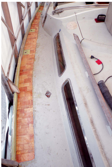
Under the winter cover, a new section of bulwark and deck core are in place and ready for finishing, at left. The bow section has been re-cored and faired and is ready for primer, center. The first area where the repair was completed was at the bow, at right.
