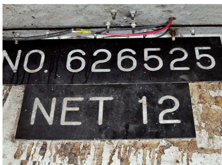
Del Viento , a U.S. documented vessel, upper right, has her official number secured to the interior structure, at right. A similar requirement applies to a Canadian vessel, at left.
