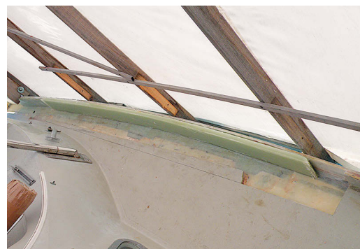
Steve removed the inner bulwark skin and rotten deck core in sections, at top, and rebuilt the bulwark piece by piece out of fiberglass cloth and epoxy resin in specially built molds, center. A section of the new bulwark is ready for installation, above.
