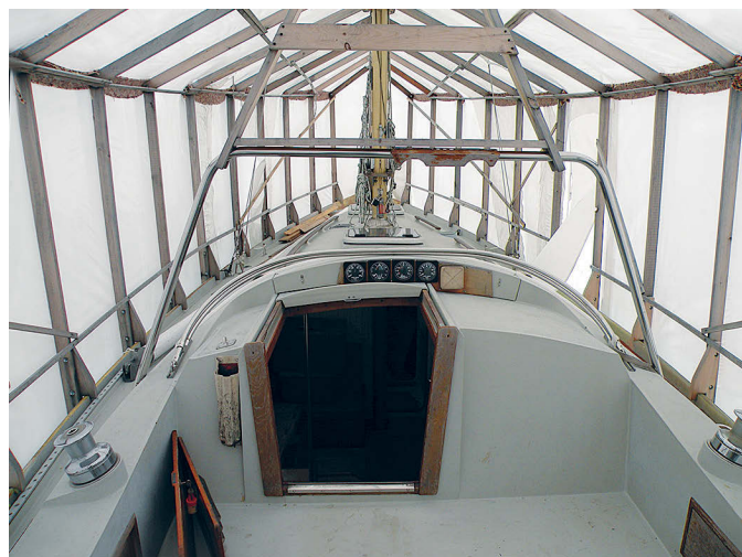
Levity lies at her mooring before the repair to her hull-to-deck joint, at left. Once ashore, Levity became a workshop, at right. The shrinkwrap cover over a custom frame admitted lots of light and allowed Mary and Steve to continue with the repair work throughout the winter months.
