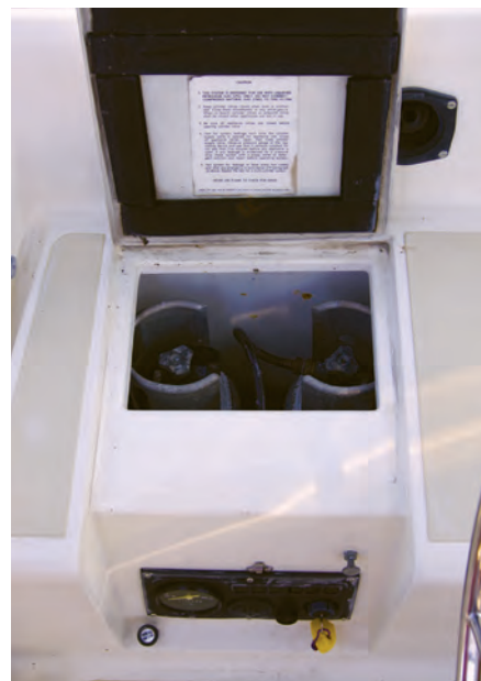
Two 11-pound propane tanks are neatly stowed in a dedicated cockpit locker that drains overboard. The engine control panel is recessed into the seat front.
