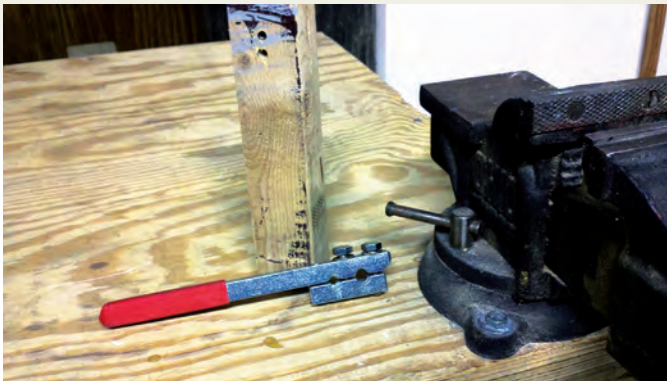
A wooden block with a hole and a kerf makes an excellent jig for sawing stainless-steel cable with an ordinary hacksaw, and the red-handled crimping tool is essential for stainless-steel terminals, at left. The crimping tool must be held securely in a vise, at right, while the bolts are tightened little by little on alternate sides of the terminal. The signal to stop tightening is when the jaws of the tool touch on both sides. (Fittings, such as the pelican hook in the picture, do not need to be attached while crimping.)
