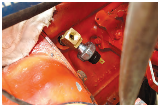
John's engine instrument panel had an oil-pressure gauge but John wanted to add an oil-pressure warning light. He took off the pressure sensor, at left, and inserted into the oil line a brass tee fitting into which he screwed the switch for the warning light, at right.
