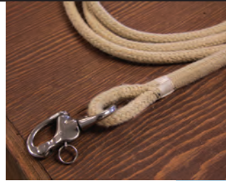
A snap shackle spliced into New England's Sta-Set Vintage.
