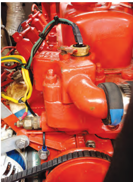
John was able to use a pre-tapped hole in the thermostat housing to fit the sensor for the temperature warning light (green and black wires), at left. The ammeter and the tachometer are wired to the alternator, at right.
