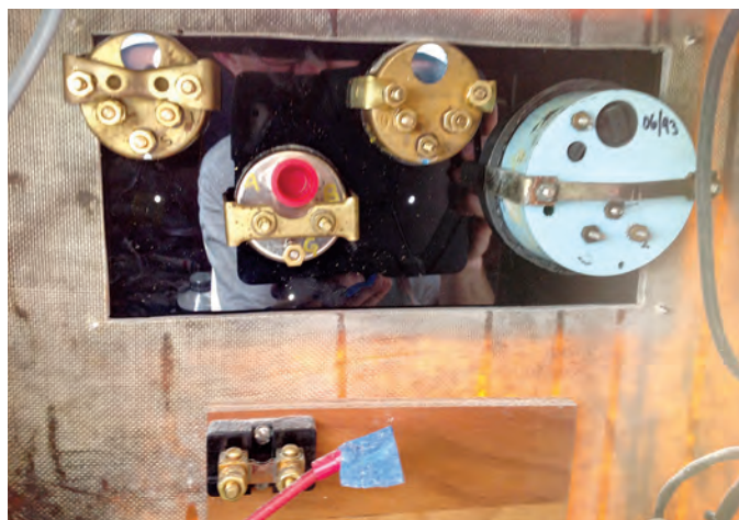
John made a pattern for the layout of his new engine panel, top right, then transferred the centers of the components to a sheet of black acrylic. He assembled the gauges and lamps onto the acrylic and installed the panel, at left, then connected, labeled, and tidied up the wiring, at right.
