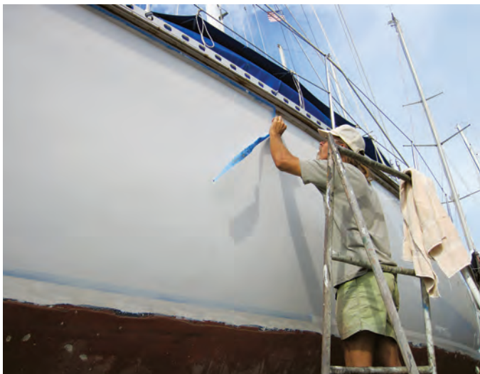
Chris used a straight-edge razor blade to pry up a corner of the masking tape, at left, then carefully removed the tape. By investing their own time and labor, Chris and Anne gave Mr. Mac a gleaming hull, at right, for a fraction of the time and cost of a professional spray job.
