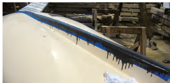
Ganymede's dinghy gets dragged up all manner of beaches and its skeg was showing wear. At a boatbuilder's suggestion, Ben applied a mixture of carborundum in epoxy as a protective layer, above.
