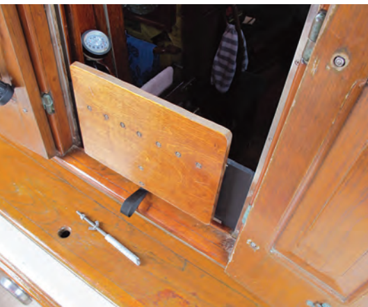
With the support strut released, the seat folds down for quick stowage, at left. Grinding the groove in the support rod takes patience, center, and safety glasses are essential. A Dremel tool and sanding drums can be used instead of a router to trim the edges of the hatchboard, at right.
