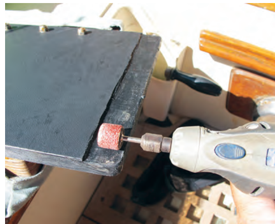
With the support strut released, the seat folds down for quick stowage, at left. Grinding the groove in the support rod takes patience, center, and safety glasses are essential. A Dremel tool and sanding drums can be used instead of a router to trim the edges of the hatchboard, at right.
