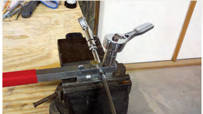
A wooden block with a hole and a kerf makes an excellent jig for sawing stainless-steel cable with an ordinary hacksaw, and the red-handled crimping tool is essential for stainless-steel terminals, at left. The crimping tool must be held securely in a vise, at right, while the bolts are tightened little by little on alternate sides of the terminal. The signal to stop tightening is when the jaws of the tool touch on both sides. (Fittings, such as the pelican hook in the picture, do not need to be attached while crimping.)
