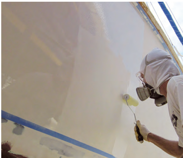
Chris applied the Awlgrip topcoat in 3-foot sections, overlapping with the wet edge of the previous section, at left. Note the difference in texture between the current section, with lots of air bubbles, and the previous section, which has already smoothed out. Once the paint was applied to a section, Chris used full top-to-bottom strokes to spread it evenly and minimize the air bubbles, at right.
