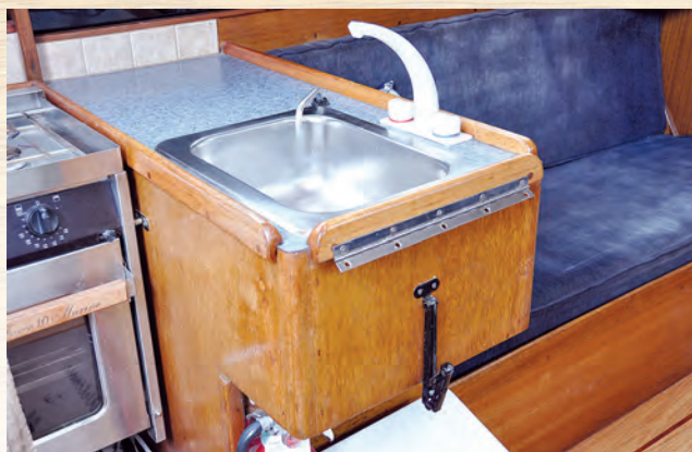
The board is attached by a hinge to the counter's fiddle rail, which provides the needed offset for the drop-leaf support bracket.
