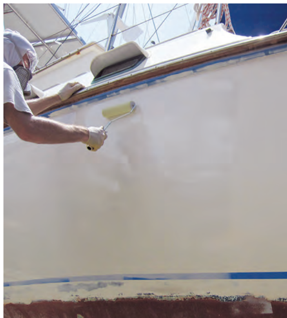
Chris applied the Awlgrip topcoat in 3-foot sections, overlapping with the wet edge of the previous section, at left. Note the difference in texture between the current section, with lots of air bubbles, and the previous section, which has already smoothed out. Once the paint was applied to a section, Chris used full top-to-bottom strokes to spread it evenly and minimize the air bubbles, at right.
