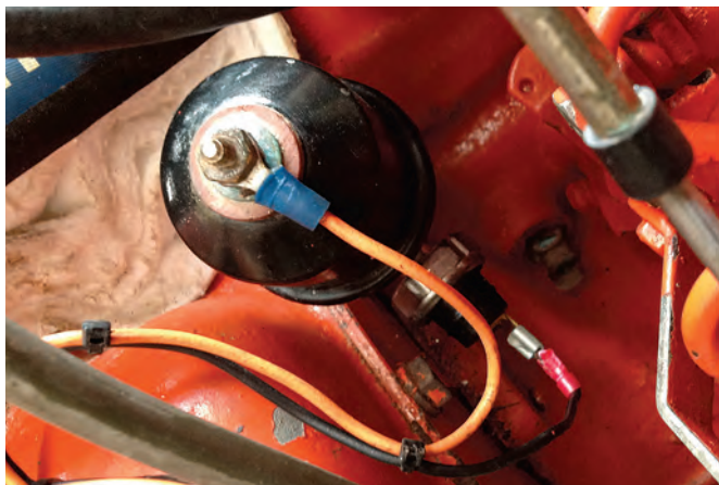
John's engine instrument panel had an oil-pressure gauge but John wanted to add an oil-pressure warning light. He took off the pressure sensor, at left, and inserted into the oil line a brass tee fitting into which he screwed the switch for the warning light, at right.
