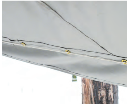
The opening in the after end of the enclosure is there to reduce pressure buildup in strong winds, at left. Richard and Terry settled on a lashing system, center, where a line passes through grommets and around the lifeline, but it's a work in progress. A "door" built into the cover allows easy ingress and egress, at right. Richard now has a sheltered cockpit with full headroom, below, where he can work or entertain his marina mates, David Ladd, left, and Jerry Riggs, right.
