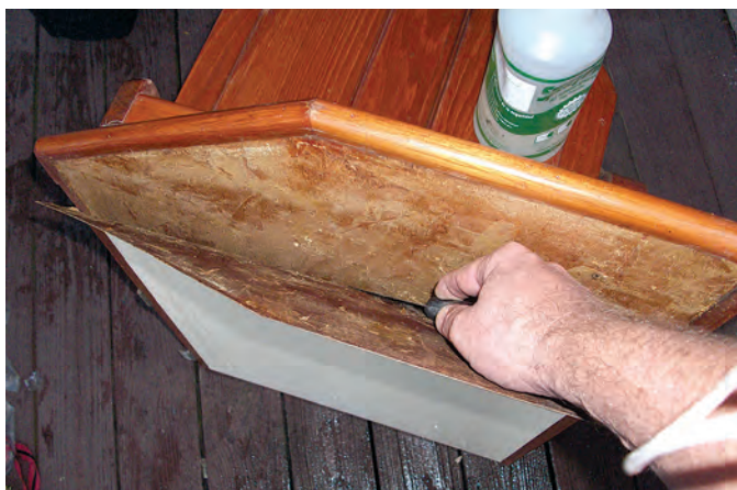
Removing the Formica was a delicate process that required lots of lacquer thinner, putty knives, and patience, at left. To get at the Formica, Scott removed the fiddles from the table's edges. After fitting the copper, he reinstalled the fiddles and coated them with epoxy, at right. While he was at it, he fitted new hinges.
