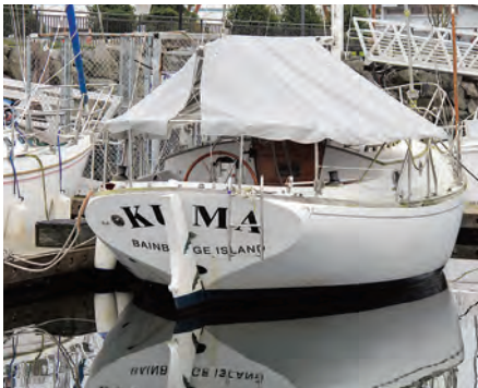
The opening in the after end of the enclosure is there to reduce pressure buildup in strong winds, at left. Richard and Terry settled on a lashing system, center, where a line passes through grommets and around the lifeline, but it's a work in progress. A "door" built into the cover allows easy ingress and egress, at right. Richard now has a sheltered cockpit with full headroom, below, where he can work or entertain his marina mates, David Ladd, left, and Jerry Riggs, right.
