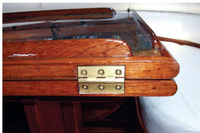
Removing the Formica was a delicate process that required lots of lacquer thinner, putty knives, and patience, at left. To get at the Formica, Scott removed the fiddles from the table's edges. After fitting the copper, he reinstalled the fiddles and coated them with epoxy, at right. While he was at it, he fitted new hinges.
