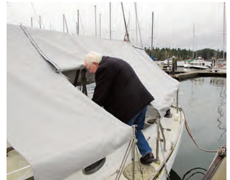
The opening in the after end of the enclosure is there to reduce pressure buildup in strong winds, at left. Richard and Terry settled on a lashing system, center, where a line passes through grommets and around the lifeline, but it's a work in progress. A "door" built into the cover allows easy ingress and egress, at right. Richard now has a sheltered cockpit with full headroom, below, where he can work or entertain his marina mates, David Ladd, left, and Jerry Riggs, right.
