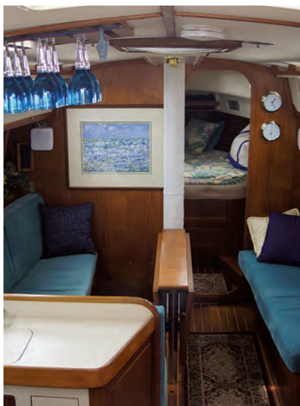
While the saloon has a classic arrangement and proportions, at left, the forward cabin has an island double berth. The top of the icebox doubles as the chart table, center. Aft, the head compartment is on the starboard side and a quarter berth, with lots of room and little privacy, occupies the port side, at right.
