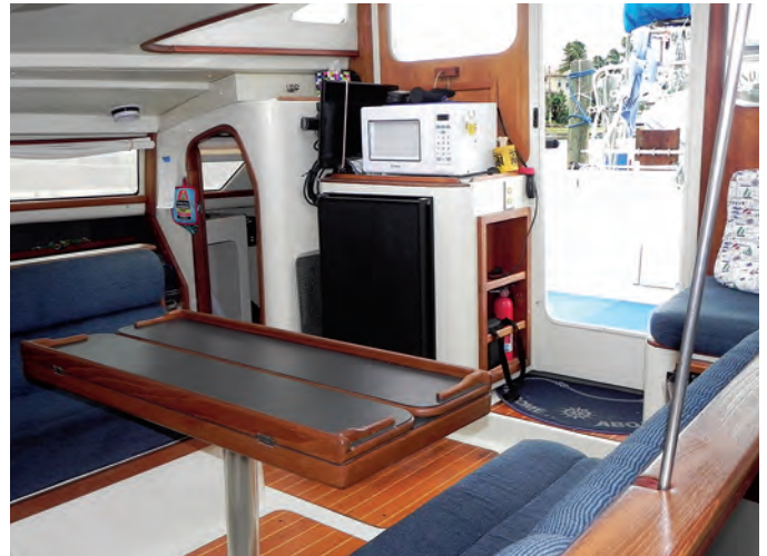
Spanning the width of the bridge deck, the saloon is generously roomy for any 32-foot boat, at left, and the sense of space is further enhanced by the open areas in the hulls abreast of the saloon. The bridge deck also has room next to the companionway for the three-way refrigerator and microwave, at right.
