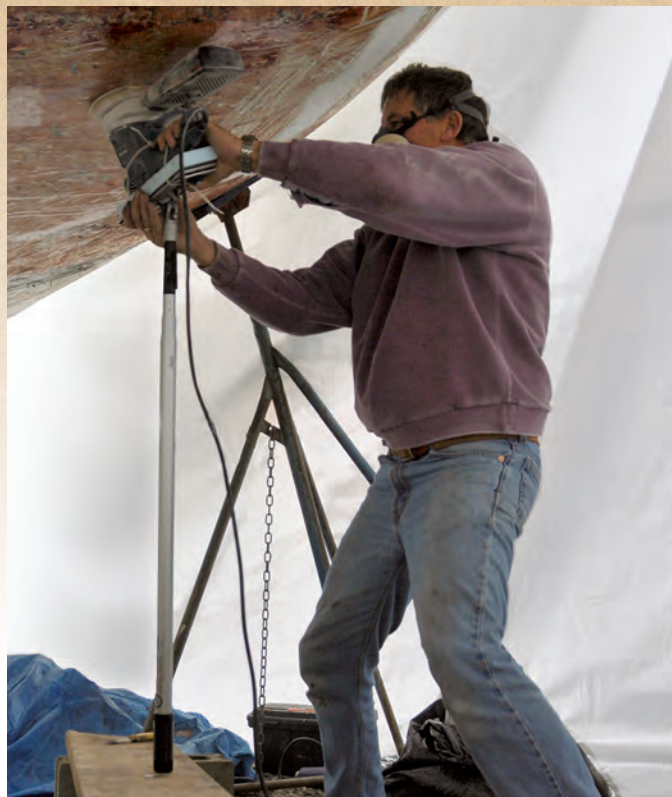
The adjustable boathook allowed Bert to sand the bottom, whatever height it was. A board laid across cinder blocks added flexibility to the arrangement.
