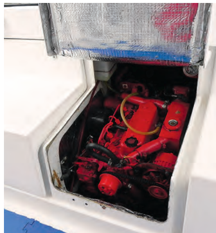
Access to the engine is very good. It's coupled to a retractable and steerable Sonic drive leg.
