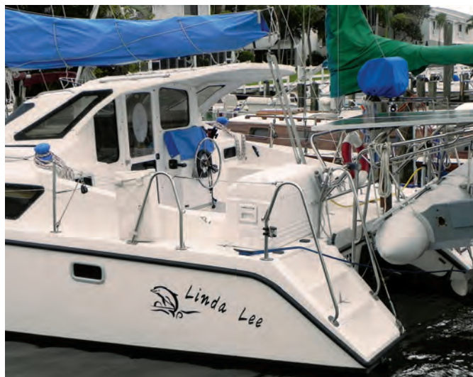
The stern of Linda Lee is a busy place, with an inflatable in davits, a solar panel, a barbecue grill, and lines for handling the retractable rudders.
