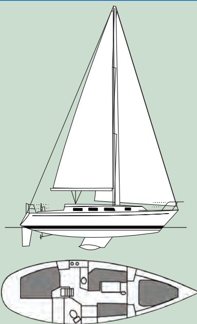
While the saloon has a classic arrangement and proportions, at left, the forward cabin has an island double berth. The top of the icebox doubles as the chart table, center. Aft, the head compartment is on the starboard side and a quarter berth, with lots of room and little privacy, occupies the port side, at right.
