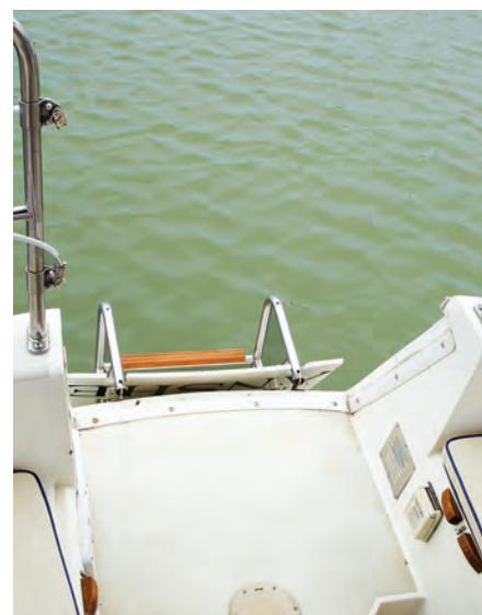
The companionway is protected by a bridge deck and the hatch slide by a sea hood, at left. It's also recessed into the cabin trunk, so it's tucked even farther under a dodger. The swim ladder, center, is attached to a panel in the transom that hinges down to provide easy access from the cockpit to the ladder, at right.
