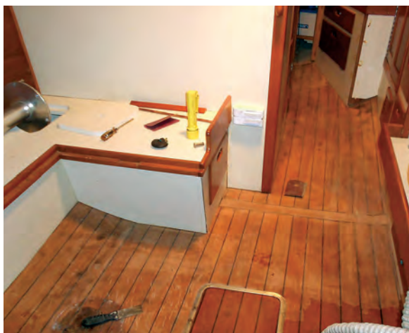
To prepare the sole for its new vinyl coverup, Art stripped the old varnish, faired the surface, and undercut the trim to allow a tidy fit.
