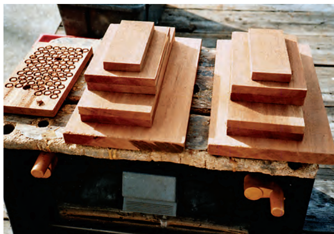
After determining the dimensions for the Dorade boxes, Richard cut out all the pieces of wood, at left. A job like this one also requires a spare length from which to cut bungs to cover countersunk screws. The baffle in the middle of the box, at right, knocks down rain and spray that enters through the vent's cowl.
