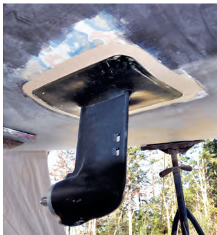
The new engine bed was a tight fit in the space, at left, and Bert had to jiggle the drive unit to fit it with the limited height available. A rubber fairing surrounds the drive leg, at center, and is glued to the hull. A Gori folding propeller, at right drives the boat well and creates little drag when the boat is sailing.
