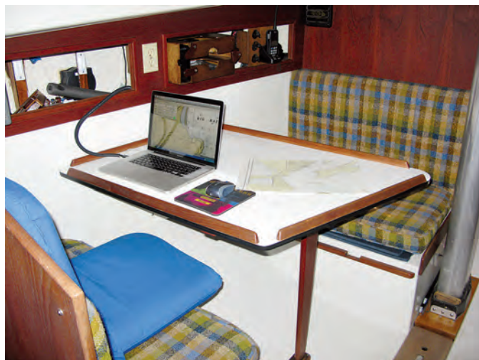
The convertible dinette seats four in a pinch, at left, but it's more comfortable for two. Note the cubbies outboard and, at lower right, the troublesome mast step. The chainplate is bolted to a plywood knee under the sidedeck, at right. Water leaking past old sealant around the deck fitting can weaken the knee and the chainplate. The starboard settee is fitted with a lee cloth and pulls out to make a good sea berth. Easy-to-rig net hammocks are ideal for stowing veggies.
