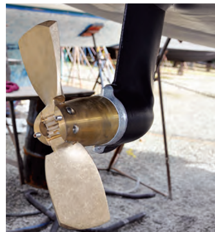
The new engine bed was a tight fit in the space, at left, and Bert had to jiggle the drive unit to fit it with the limited height available. A rubber fairing surrounds the drive leg, at center, and is glued to the hull. A Gori folding propeller, at right drives the boat well and creates little drag when the boat is sailing.
