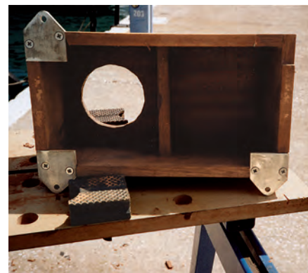
The yet-to-be-plugged screw holes are visible on the unfinished boxes, at left. After trimming the finished boxes to fit the deck camber, Richard plugged the screw holes and sanded the boxes in preparation for varnishing, center. The carpentry work done, he fitted the feet, cut from stainless-steel flat bar, at right.
