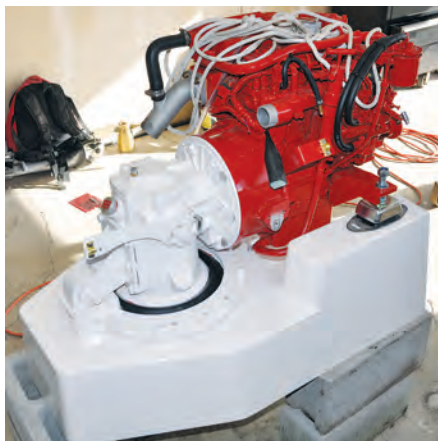
Bert assembled the engine/drive unit to its base, at left, to drill and tap holes for the mounting bolts, center. Cutting the hole in the hull was daunting, at right.
