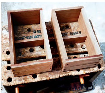
The yet-to-be-plugged screw holes are visible on the unfinished boxes, at left. After trimming the finished boxes to fit the deck camber, Richard plugged the screw holes and sanded the boxes in preparation for varnishing, center. The carpentry work done, he fitted the feet, cut from stainless-steel flat bar, at right.
