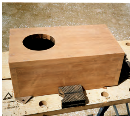
The yet-to-be-plugged screw holes are visible on the unfinished boxes, at left. After trimming the finished boxes to fit the deck camber, Richard plugged the screw holes and sanded the boxes in preparation for varnishing, center. The carpentry work done, he fitted the feet, cut from stainless-steel flat bar, at right.
