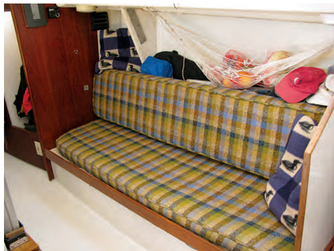
The convertible dinette seats four in a pinch, at left, but it's more comfortable for two. Note the cubbies outboard and, at lower right, the troublesome mast step. The chainplate is bolted to a plywood knee under the sidedeck, at right. Water leaking past old sealant around the deck fitting can weaken the knee and the chainplate. The starboard settee is fitted with a lee cloth and pulls out to make a good sea berth. Easy-to-rig net hammocks are ideal for stowing veggies.
