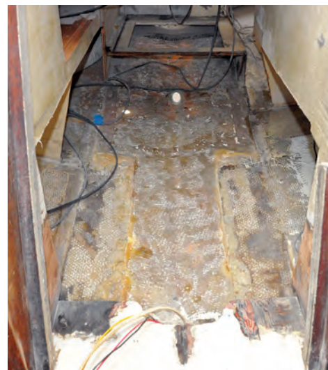
Bert cut away the old engine beds and prepared the space to receive the bed for the saildrive combination.
