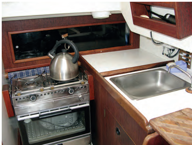
A gimbaled two-burner stove/oven, a sink, and a small countertop make up the starboard side of the compact galley. An icebox and counter are to port. Jerry built a cutting board that slips over the top companionway step.
