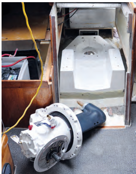
The new engine bed was a tight fit in the space, at left, and Bert had to jiggle the drive unit to fit it with the limited height available. A rubber fairing surrounds the drive leg, at center, and is glued to the hull. A Gori folding propeller, at right drives the boat well and creates little drag when the boat is sailing.
