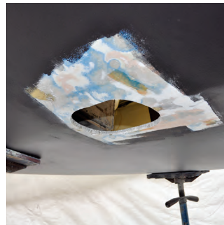
Bert assembled the engine/drive unit to its base, at left, to drill and tap holes for the mounting bolts, center. Cutting the hole in the hull was daunting, at right.
