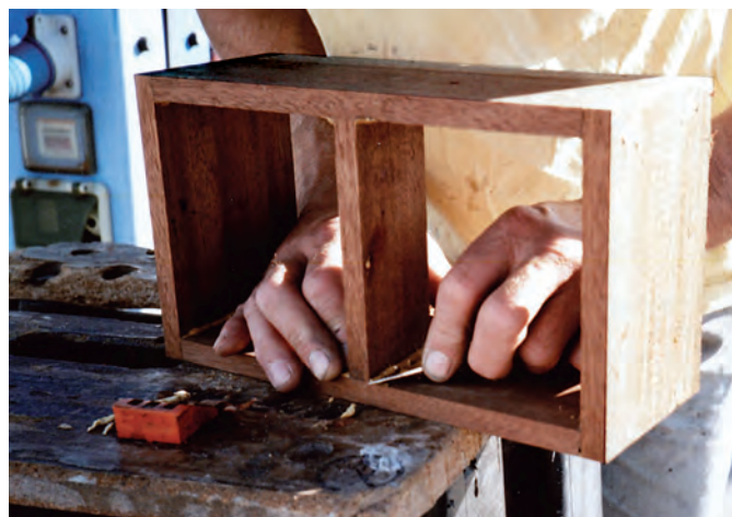
After determining the dimensions for the Dorade boxes, Richard cut out all the pieces of wood, at left. A job like this one also requires a spare length from which to cut bungs to cover countersunk screws. The baffle in the middle of the box, at right, knocks down rain and spray that enters through the vent's cowl.
