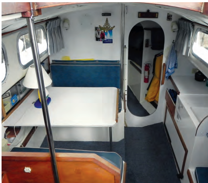
The dinette is raised, putting the cabin windows at eye level for diners, at left. A counter extension expands the galley with its molded sink. A shippy detail is the oval cutout in the main bulkhead that allows easy passage while maintaining its strength. The vertiginous companionway ladder, at right, is well provided with handholds.
