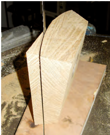
Jim cut out the new block for the lower bearing on his band saw, at left, and epoxied studs into it to receive the bearing, above. The bronze bearing and shaft-seal assembly, at right, is a readily available stock item.
