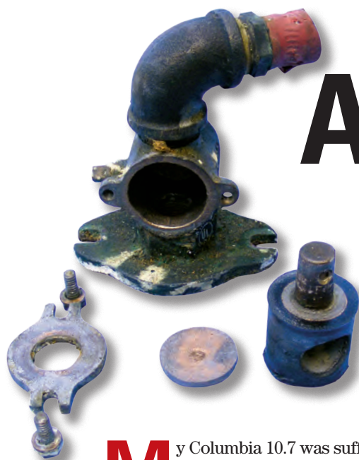
The cylindrical rubber plug in the old Groco SV-type seacock had seized solid.
