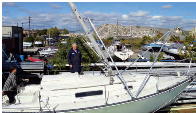
The pivot point of the A-frames is not level with that of the mast, but the apex of the after A-frame, attached to the spinnaker-pole car, accommodates the offset by rising up the mast as the mast is being raised.
