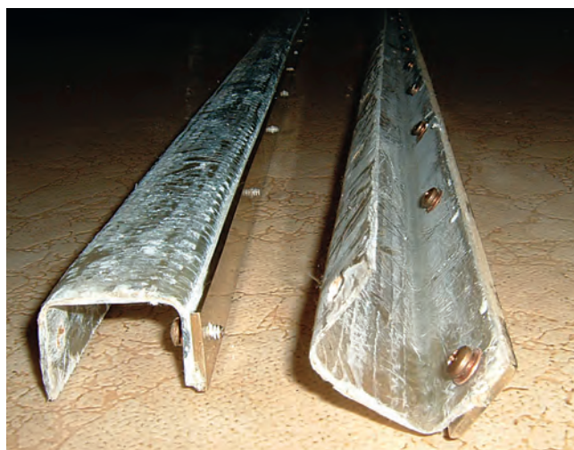
Ben made his fiberglass companionway-hatch slides in one piece using a 2 x 4 as a mandrel, then cut them apart with a table saw.
