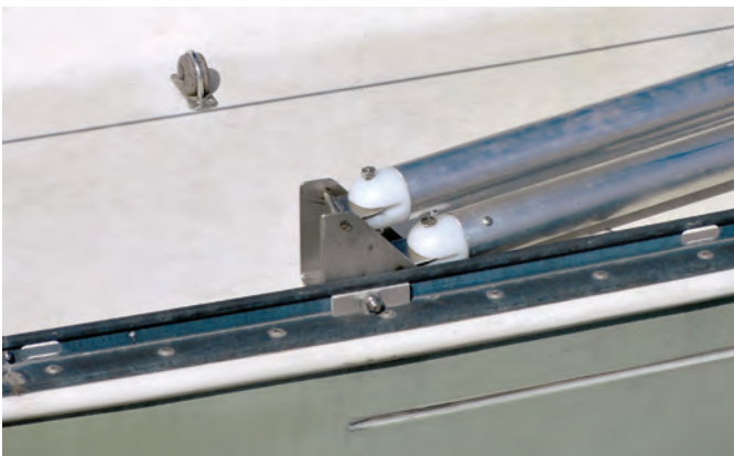
The deck pivot is designed to allow the A-frames to stow one on top of the other when folded down. The toggle connections allow freedom of movement. The bracket is bolted to the toerail so it can be easily removed when not needed.
