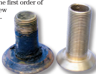
The old through-hull (on the left in both photos) has a much larger base than the new one (on the right). Had Paul used the new one, he would have had to cut it to length.
