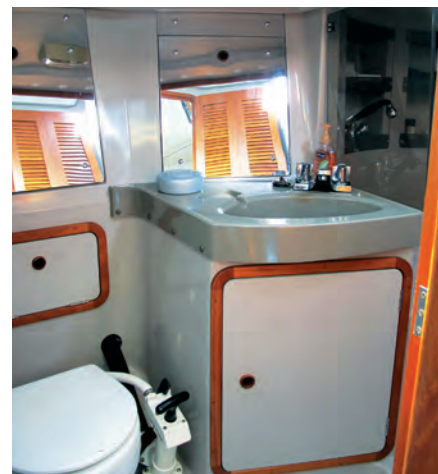
Removing the companionway ladder reveals the front of the engine, at left, but the back and sides are harder to get at. Molded fiberglass inner liners are well suited to the head, at right, where the inevitable moisture from the shower, sink, and toilet can damage wooden components.
