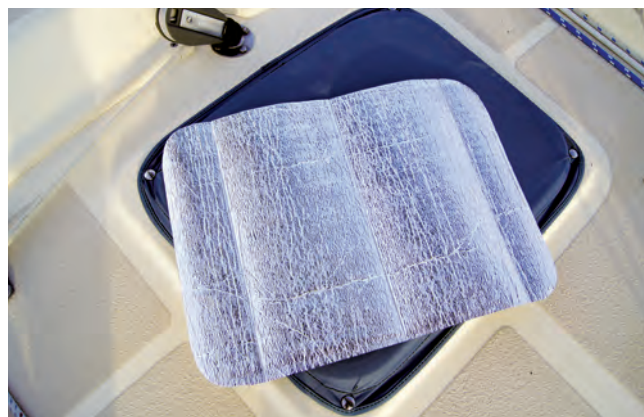
Deck hatches let in daylight but also let in unwelcome UV and heat. Gregg’s Sunbrella covers protect the boat’s interior from both, at left. Gregg further cut down the heat entering the boat by fitting reflective panels he cut from an automobile windshield sun screen, at right.
