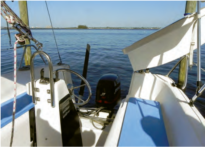
The aft end of the cockpit, which incorporates the helmsman's seat, lifts up on a hinge to provide access to the outboard motor and swim platform, at left. Unusual for a general-purpose boat like the MacGregor are its twin rudders, at right, that are retractable and linked together in the steering system. All 26X models have pedestal steering with a small, powerboat-style wheel, below. Long turns at the helm can be tiring.
