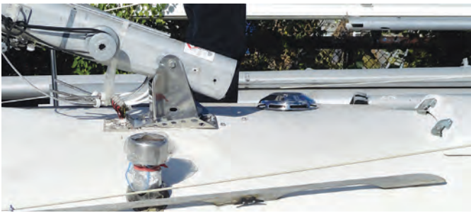
A custom-made stainless-steel tabernacle allows the mast to pivot and also serves as the mast step.
