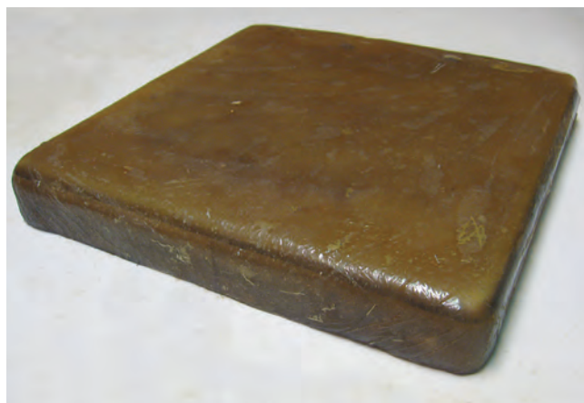
Ben's plastic-bag technique over a male mold results in tight outside corners. The layout doesn't lift or form bubbles and fairs easily.
