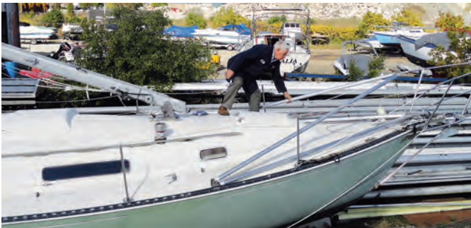
After the mast has been lowered and the after A-frame disconnected from the mast, both frames can be rotated forward so they can be stowed on deck or removed. Once disconnected from the deck, the A-frames “scissor” together for ease of storage.
