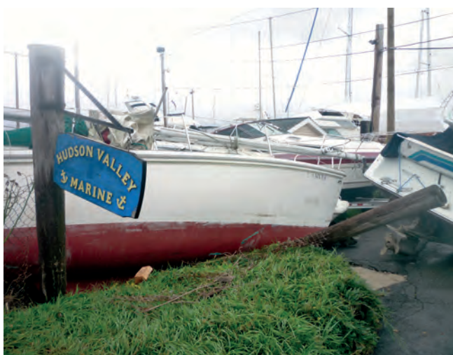
In the Viking yard, above, several powerboats and smaller sailboats floated off their cradles and jack stands and came to rest where the wind blew them — unfortunately, on top of their rudders and propellers. The yard next door presented a similar picture, below.
