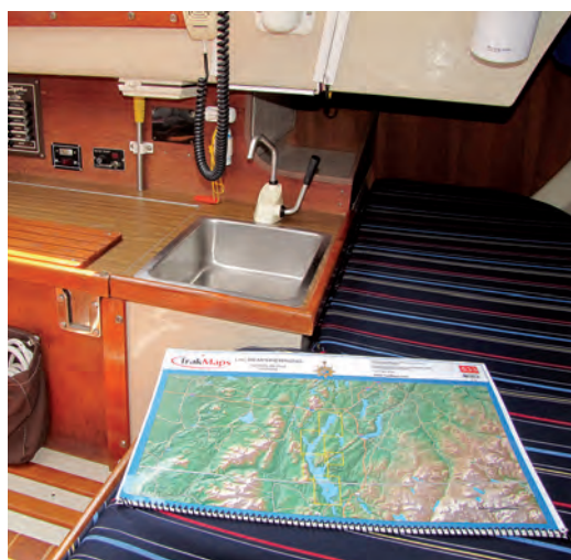
The compact galley is under the bridge deck, at left, and the saloon settees extend under the cockpit. A portable toilet fits under a fold-down lid at the aft end of the V-berth, at right.
