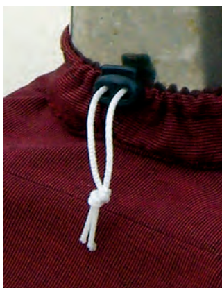
The cord lock on the drawstring holds the collar snugly around the Dorade vent.
