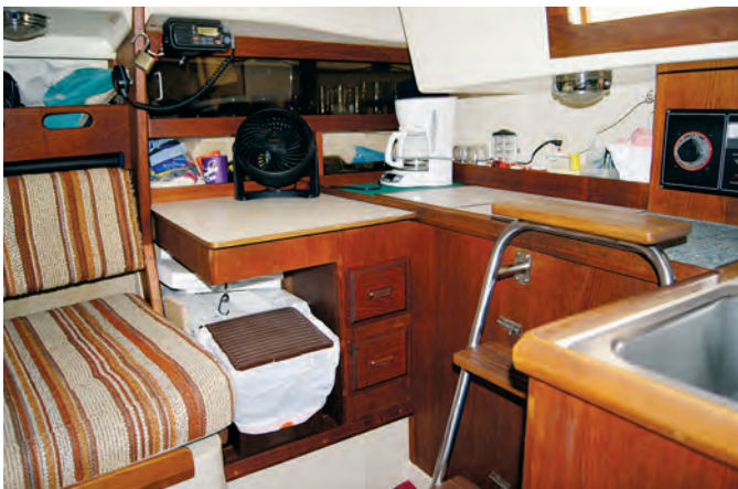
The navigation station, at left, is essentially a small hinged countertop with storage underneath. The defining feature of the O'Day 37 is its aft cabin, at right. It has its own entrance from the cockpit and contains an athwartships double berth and a private head compartment.
