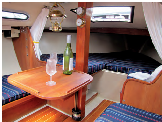
Although the Capri 25 does not have standing headroom, the 9-foot 2-inch beam makes for a spacious saloon, at left. The compression post for the mast provides a sturdy support for a small table in the saloon, at right, and a curtain allows some privacy between the saloon and the V-berth.
