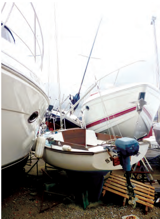
In the Viking yard, above, several powerboats and smaller sailboats floated off their cradles and jack stands and came to rest where the wind blew them — unfortunately, on top of their rudders and propellers. The yard next door presented a similar picture, below.
