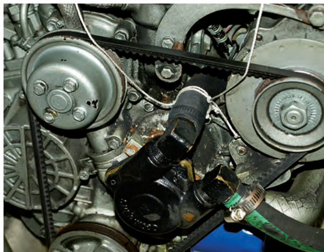
Two lengths of nylon twine tied around the hose gave Clarence the purchase needed to pull the hose onto the barb.
