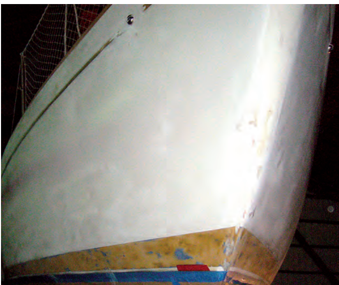
Nobody liked the "blah" off-white hull color so, over their first winter with the boat, E-J and Tim stripped the bootstripe and spent 80 hours sanding the hull, at left. The deep blue and the red bootstripe certainly banished the blahs, at right.
