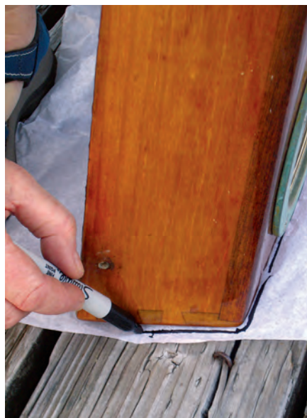
Judy decided to protect Cetacean 's Dorade boxes, which Ron had freshly varnished, at left, by making Sunbrella covers for them. She started by unscrewing the starboard aft box and drawing around it for a pattern, at right.
