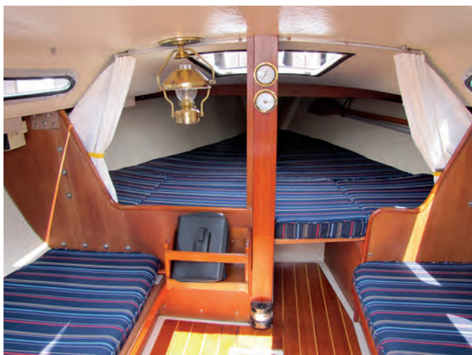
Although the Capri 25 does not have standing headroom, the 9-foot 2-inch beam makes for a spacious saloon, at left. The compression post for the mast provides a sturdy support for a small table in the saloon, at right, and a curtain allows some privacy between the saloon and the V-berth.
