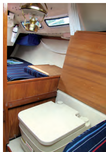
The compact galley is under the bridge deck, at left, and the saloon settees extend under the cockpit. A portable toilet fits under a fold-down lid at the aft end of the V-berth, at right.
