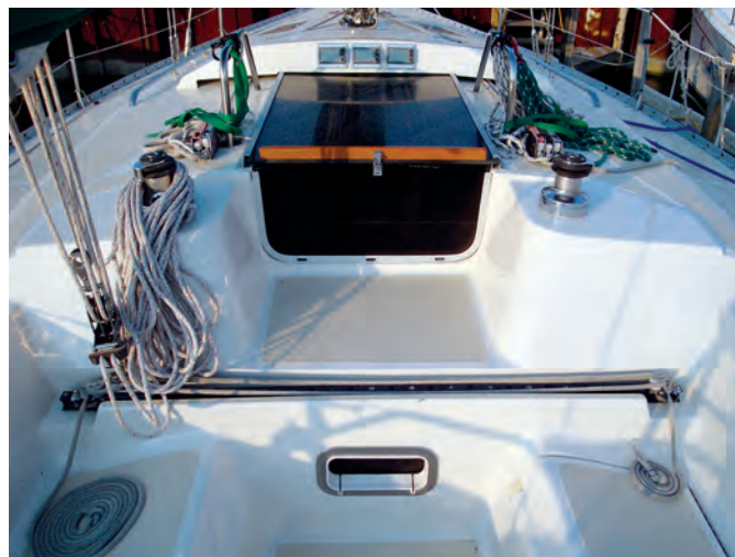
The T-shaped cockpit allows easy access around the helm, at left, and the coamings give decent back support. Great care went into the deck tooling here, too, to create the sculpted seating surfaces. The bridge deck, at right, provides stooping headroom in the aft cabin.
