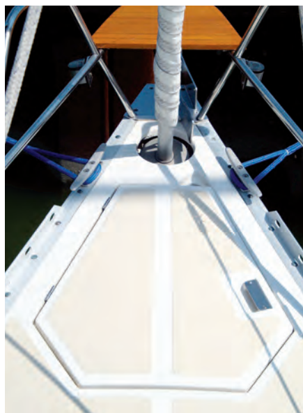
The furler drum is cleverly recessed under the deck just forward of the anchor locker.
