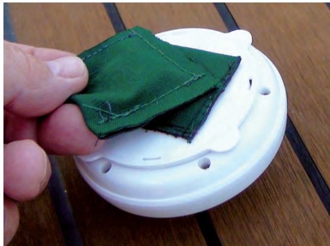
Stephen sewed washers into Sunbrella sleeves and bolted them to the spotlight bases, at left. Magnets sewn into similar sleeves, at right, and placed on the outside of the canvas hold the lights on the inside of the Bimini or dodger.
