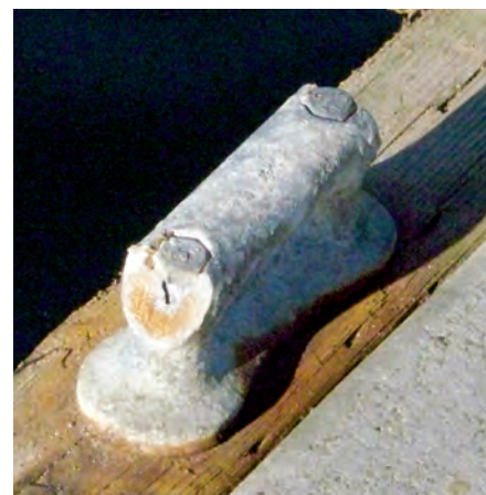
The explosion split the boat's hull down the stem, above, and blew off the deck with enough force to shear the ears off a dock cleat, at right.
