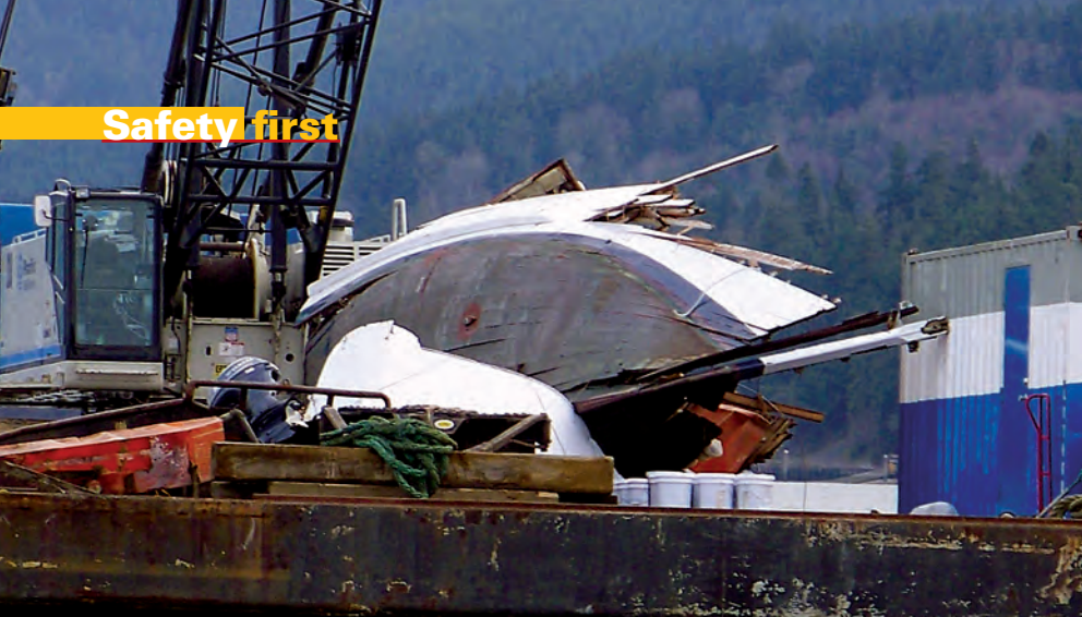
The explosion split the boat's hull down the stem, above, and blew off the deck with enough force to shear the ears off a dock cleat, at right.
