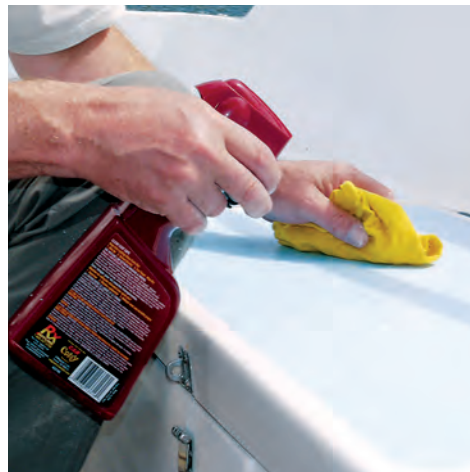
A wool pad, at left, is best for applying and working with rubbing compounds and polishes, and using a variable-speed rotary polishing machine almost goes without saying. After the compounding and polishing stage, wiping the surface with a cloth dampened with detailing spray, above center, removes residue. Wax should be applied sparingly, and a waffle-finish foam pad works well for applying it, above right. Peter's toil begins to show results, below.
