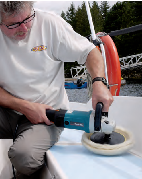
A wool pad, at left, is best for applying and working with rubbing compounds and polishes, and using a variable-speed rotary polishing machine almost goes without saying. After the compounding and polishing stage, wiping the surface with a cloth dampened with detailing spray, above center, removes residue. Wax should be applied sparingly, and a waffle-finish foam pad works well for applying it, above right. Peter's toil begins to show results, below.
