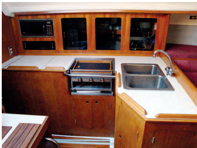
There's enough counter space in the L-shaped galley, above, for reasonably convenient food preparation. The two-burner CNG cooktop has a broiler and a microwave does duty as an oven when shore-power is available.
