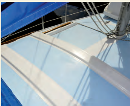
The port side of the hatch slide seems to have better withstood six months of weathering, at right.
