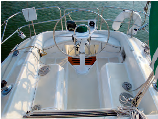
The T-shaped cockpit allows easy access around the helm, at left, and the coamings give decent back support. Great care went into the deck tooling here, too, to create the sculpted seating surfaces. The bridge deck, at right, provides stooping headroom in the aft cabin.
