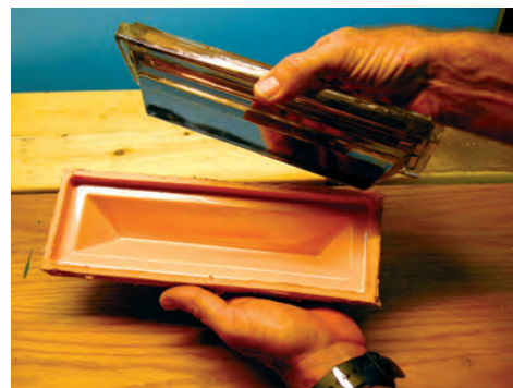
The illustration, at top, shows the principle of the master mold. To reduce the amount of compound needed to surround the master prism, David built the box in layers, at left. He set the prism on the base, clamped the mold box down, and poured the compound, above. Prism and mold separated easily, above right.
