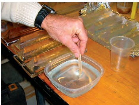
After experimenting with resin/catalyst ratios, David mixed the resin carefully to avoid introducing bubbles, above left. He leveled the mold, then gently filled it with resin, above right. The cured prism released easily from the mold, at right, and is remarkably clear.
