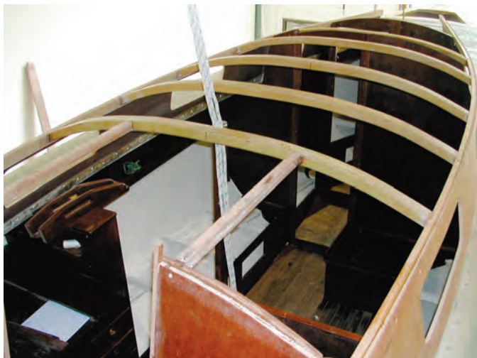
The Mistral was built with a wooden trunk cabin, and Stephen rebuilt it, at left. He kept the original beams to use as patterns for the new ones. Stephen also refinished the joiner work, at right, and made new parts as needed. His mother was his inspiration, so he named the boat for her, below.
