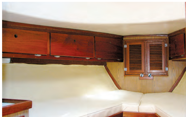
The Alberg 35 was offered with a choice between two arrangements. Finesse has the "California" galley and dinette, at left. Another of Richard's projects was to install real storage lockers in the V-berth cabin, at right . . . not to mention renew the upholstery.
