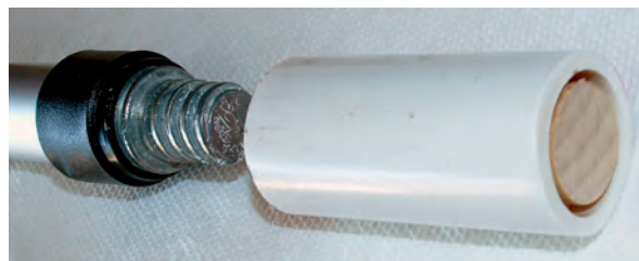
The coupler and dowel fit neatly inside the PVC pipe.
