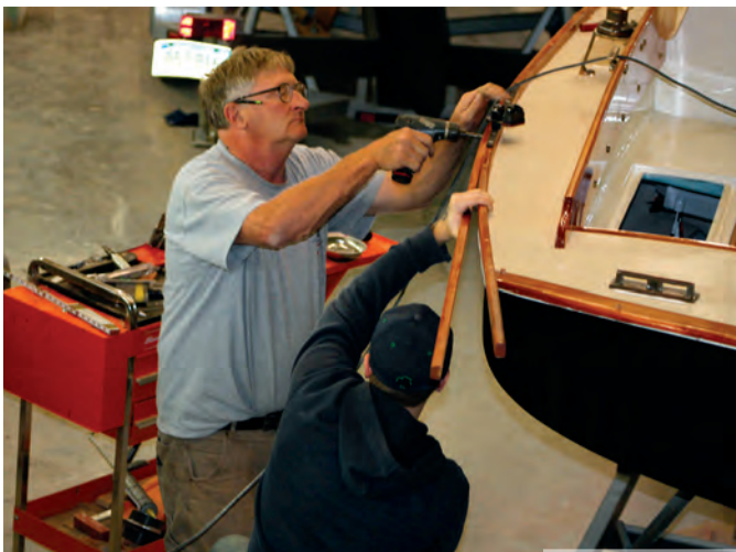
Bob, who is the woodworking specialist at the shop, attaches a toerail to a Cape Dory Typhoon, at left, as a finishing touch to a full restoration. A restored Typhoon Weekender sits on her trailer, at right, awaiting transportation to new cruising grounds in her new life.
