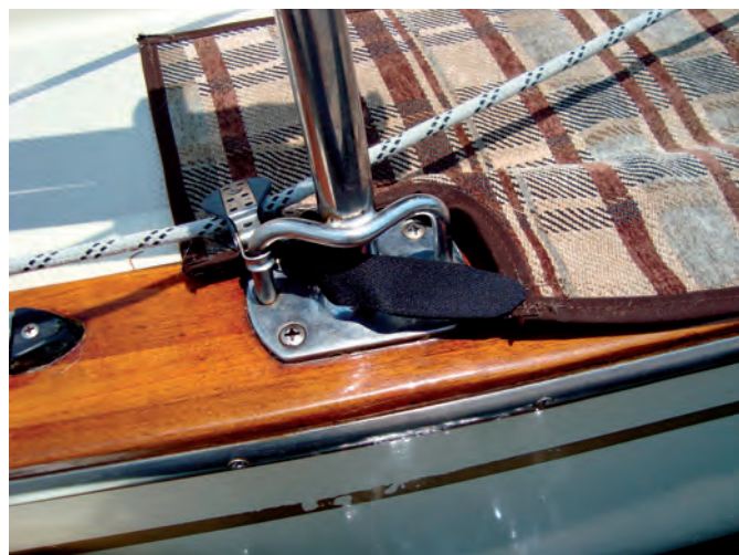
One mat protects the varnished cap rail and gives the dogs traction on the sidedeck. Velcro straps secure it to the stanchion bases.
