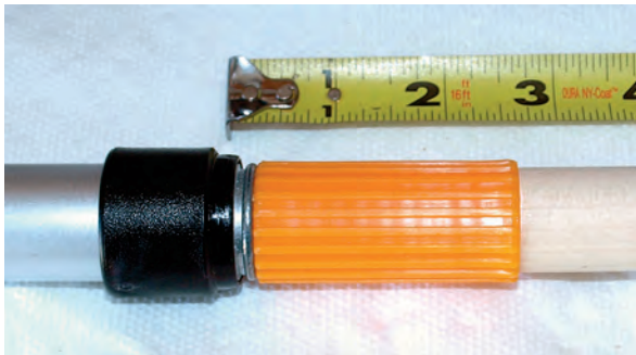
Clarence measured from where the PVC pipe seated on the pole to the end of the coupler and added ¼ inch.
