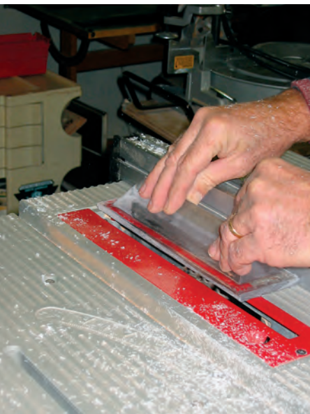
David used a table saw to cut the rabbet for the bezel.
