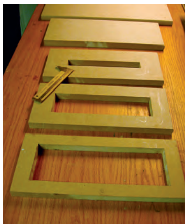
The illustration, at top, shows the principle of the master mold. To reduce the amount of compound needed to surround the master prism, David built the box in layers, at left. He set the prism on the base, clamped the mold box down, and poured the compound, above. Prism and mold separated easily, above right.
