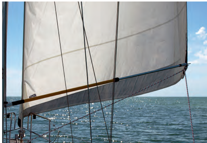
Clarence's light-duty, low-cost whisker pole is just the ticket for holding out the genoa when running in light winds.
