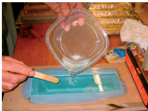
After experimenting with resin/catalyst ratios, David mixed the resin carefully to avoid introducing bubbles, above left. He leveled the mold, then gently filled it with resin, above right. The cured prism released easily from the mold, at right, and is remarkably clear.
