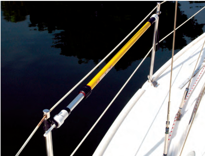
Clarence stows the whisker pole between two stanchions. The spike fits in an eye on one and the snap clips into a shackle strapped to the other.
