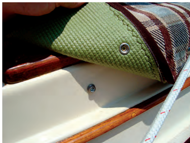
Stephen used the existing Bimini-strap snaps to attach the upper mat to the coaming. The binding tape is a tidy finishing touch.
