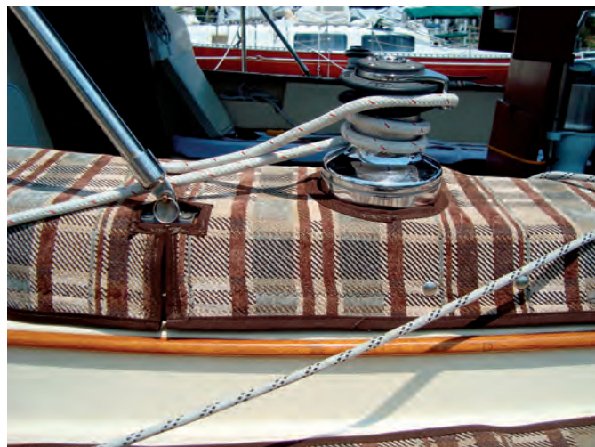
The upper mat protects the cockpit coaming cap. Stephen made cutouts to go around the winch and other hardware.
