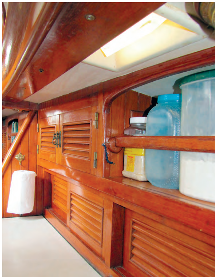
Aboard Nine of Cups , prisms direct daylight into places, like this corner of the galley, that might otherwise be in shadow.
