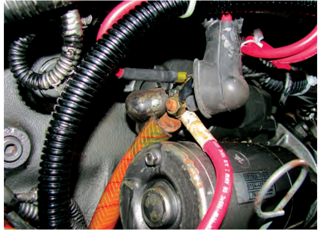
Harry ran the new wires from the key switch to the starter solenoid alongside the wiring harness and secured them to it with cable ties, at left. The starter solenoid sits atop the starter, above right. The new wires are the solid red pair at the upper right.
