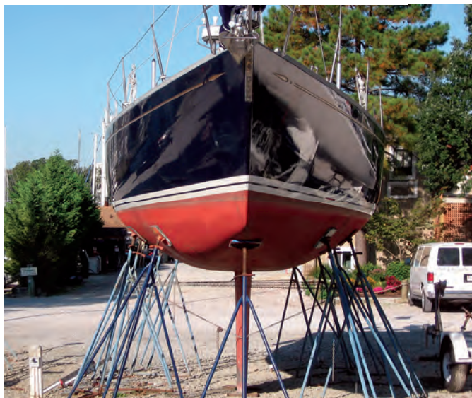
This Swan from about 1980 shows the effect of the IOR depth measurements, above. The hull turns sharply at the CMD point and the bottom is flat. IOR sterns were often pinched right at the rudder, below.
