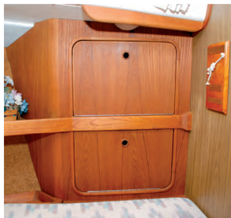
To open up the saloon, Ron cut back the leeboards on the pilot berths, at left. In the forward cabin, he fitted cabinets, at right, that provide useful storage space without impinging on the V-berth.
