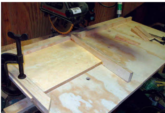
To produce uniform scarf cuts, the jig must first be clamped firmly to the work table, at left. The wedges lying on the far side of the table are the offcuts. With the piece to be cut clamped to the fence, at right, advancing the saw slowly will produce a clean cut.
