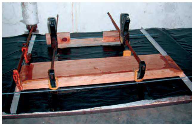
With his combination of clamps, Dave was able to put the squeeze on three edges of the table leaf, above. The finished mitered joints in the table's border pieces justified Dave's efforts, at right.
