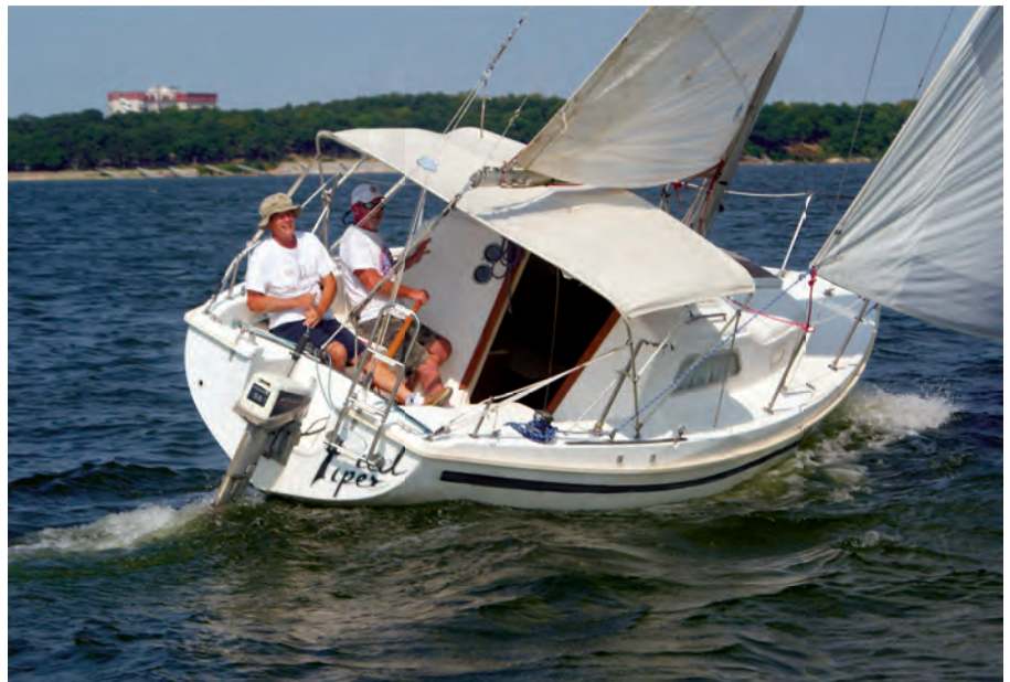
The centerline motor well makes it easy to operate and turn the outboard, including kicking it up. The offset companionway goes with the dinette arrangement in the interior.
