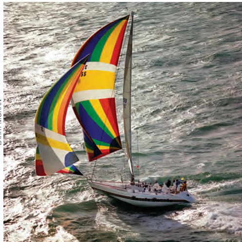
In a typical scene from 1983, Razzle Dazzle is flying a spinnaker and a blooper. Note the big hole in the water amidships . . . into which the boat can easily roll.
