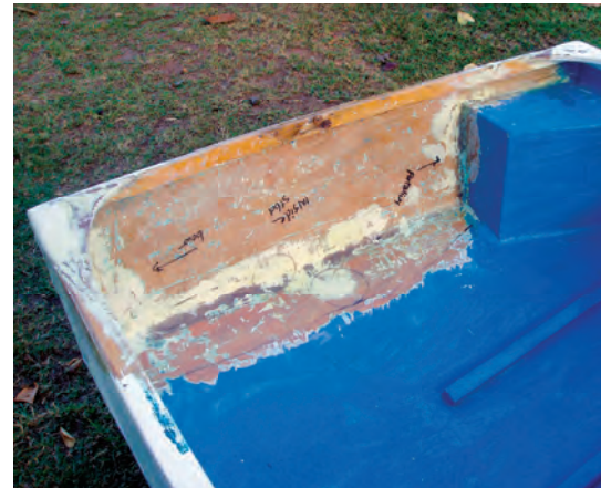
Bacio's rugged construction probably saved Philip's life when he was hit broadside by a speeding powerboat in Nuku Hiva, above. The collision stove in the starboard aft hull panel, leaving the forward half of the boat undamaged. When repairing Bacio , three photos at right, Philip and Leslie made do with the limited supplies they had on board together with what was available in their remote location. She was afloat again in a week.
