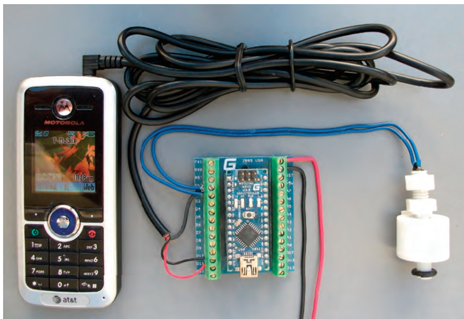
Connecting a sensor and phone to the microcontroller is easy. The software does the clever stuff.
