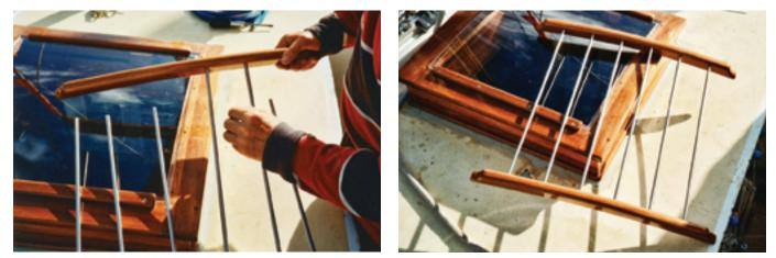
Knowing that varnishing the various parts of the hatch in situ would be difficult, Nick designed the guards to be disassembled. Here, he is fitting the bars into the combs, at left. Once the guard was assembled, at right, he fastened the combs to the hatch from beneath.
