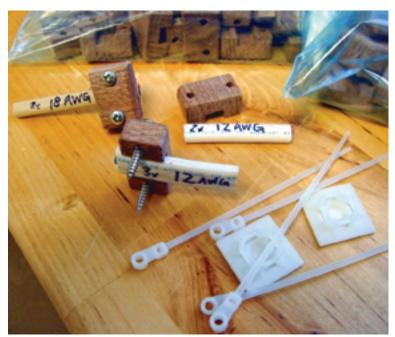
Stephen wasn't satisfied that the commercially available devices for securing electrical wiring would hold the wires firmly enough, so he made his own to fit three sizes of wire, above. When compared against a plastic cable clip, at left below, Stephen's design is more secure and more handsome, at right below.
