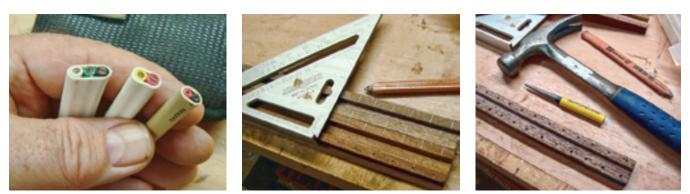
Each size of cable, at left, needed its own custom clamp. After cutting the grooves for the cables in the wood strips, Stephen marked them for fastener holes, center, then used a center punch to mark the hole centers, at right.
