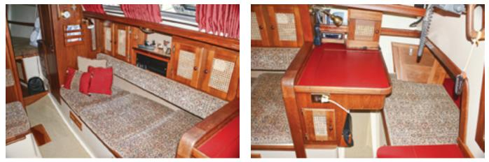
Swede built cabinets into the shelves behind the saloon settees and fitted them with cane doors for looks and ventilation, at left. Aft of the settee on the starboard side is a small navigation station, at right. Its seat is the head of the quarter berth.
