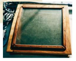
in place with wooden battens screwed down to the top of the hatch. The ends of the battens were miter cut but, instead of being joined, were left about ¼ inch apart so water could drain out at the corners.
