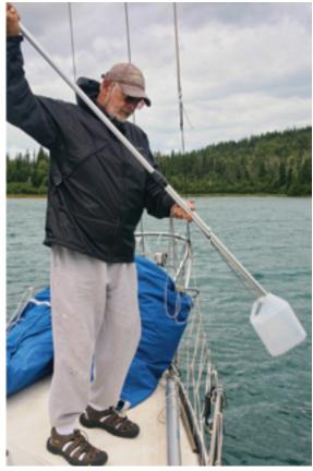
Fasten a cord to the jug's handle so you can retrieve it once you have pushed it down into the water with the boathook. Properly deployed, the container will fill with just about 1 gallon of water each time. This will be fairly easy to lift back to the deck. The same handle will be convenient for carrying the "bucket" and for pouring from it.
