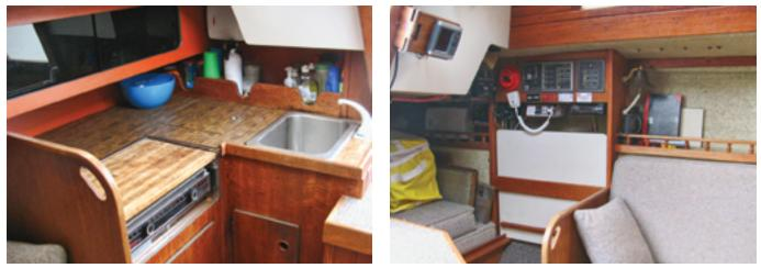
The compact galley, at left, is fitted out with an Origo alcohol stove, a small sink, and an icebox. The nav desk, at right, is cleverly designed to lift up and out for use. It is stowed against the hull and a cushion takes its place when the quarter berth is needed.
