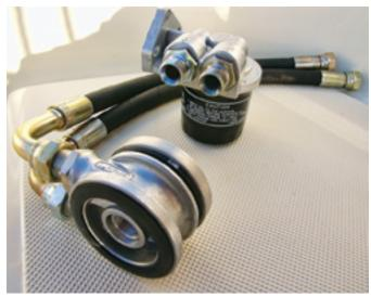
A remote oil filter kit allows the filter to be placed in a more convenient location. The piece in the foreground replaces the filter on the engine block and the other piece is the filter mounting assembly.
