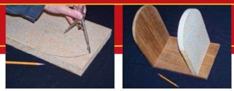
Ken made a temporary mold, at left, and attached it to the board that forms the back of his locker, center. He covered it with wax paper to prevent epoxy from adhering to it, top right. A veneer-cutting saw and a batten ensured clean straight cuts in the veneer skins. Ken clamped the veneer to the form while he glued and stapled it to the base and the back. Some of the clamps remained in place while he applied the first layer of fiberglass cloth.
