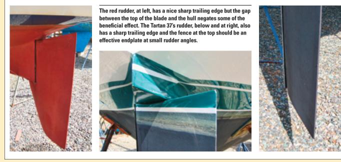
the rudder can benefit from some end-plate effect off the hull that will help keep the flow over the blade attached. We have done new rudders for a few boats that originally came with the scimitar blade and the results were always very good.
