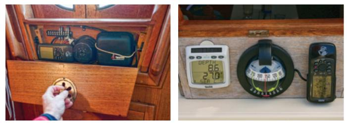
The doorframe was sufficiently deep to provide an enclosure for the backs of the compass and the depth sounder, at left. It also holds the GPS when it's not in use. Benjy's trio of instruments is convenient to view and doesn't obstruct the seating area, at right.
