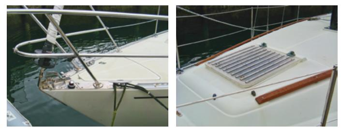
At the bow there is a small anchor locker, two cleats, and a tiny roller for handling ground tackle, at left. The forward hatch, at right, located on the coachroof above the entrance to the forward cabin, is a little too far aft to bring much breeze to crew sleeping on the V-berth.
