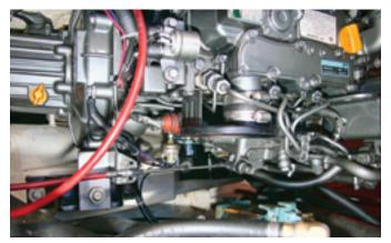
Even with the air filter removed, the oil filter was close to invisible and gaining access to change it was almost impossible.
