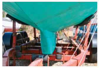
A blunt leading edge does not induce good flow over the keel. This one could benefit from an addition to give it a more parabolic shape.
