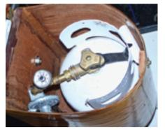
The gas regulator and pressure gauge are inside the locker, at left. The latched lid, at right, keeps out the rain but, to ensure the locker ventilates, it is not airtight.
