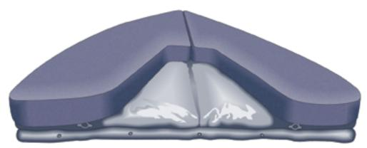
The flexible tank can fit into a space in which a hard tank would be difficult or impossible to install. An innovative idea, especially useful on small boats where space is at a premium, is a combination water tank and water bed. This illustration shows how a water bed/water tank works. The center berth cushion has been left out for clarity.
