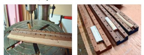
For speed and precision, Stephen used a drill press when drilling the holes, at left. The cables fit snugly in their grooves, at right. Stephen cut off the individual clamps on a band saw.
