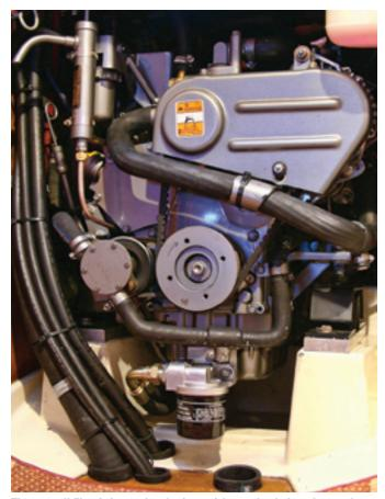
The new oil filter is located at the front of the engine below the crankshaft pulley. The oil sump pump is also visible at the top left of the photo.
