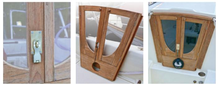
With the hasp in place, at left, the doorknob cannot be turned. It can be secured with a padlock. The entire doorframe assembly can be removed, center. The doors and their frame were built around the compass, at right, and the other instruments followed.
