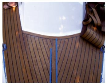
To make the synthetic deck look traditional, Eric and Kris fashioned margin pieces around the edges. Using wide masking tape let them caulk the seams without making a mess, at left. The king plank on the foredeck is a nice touch, at right. Note how flexible the material is.
