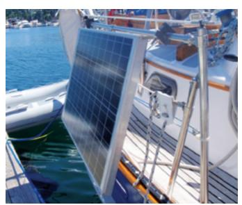
The plastic rail clamps beneath the panels are used to adjust the panels in the fore-and-aft direction and to lock them in position, at left. The panels have so far withstood 25-plus knots of wind with moderate seas. During docking maneuvers or in extreme weather, we can rotate the panels to a flat "stowed" position, at right.
