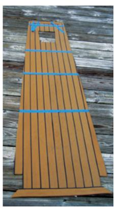
Before the TekDek could be installed, hardware had to be removed and the deck sanded smooth, at left. Kris cut sections of TekDek to the template, laid them out, and figured the joints, center. Taped together, the cockpit sole pieces await assembly on the boat, at right.
