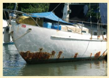
With modern coatings and TLC, a steel hull need not suffer this fate.
