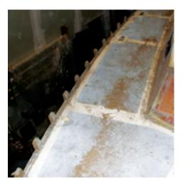
The original toerail resisted Stephen's attempts to rescue it so he cut it either side of the bolts, at top, and removed it in pieces, above.
