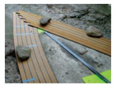
Grinding out the old deck was effective, but collateral damage to adjacent areas not covered by the new deck required additional cosmetic work. A more precise approach might have been to make shallow cuts through the top skin of the deck with a circular saw, then remove the skin to access the wet core.
