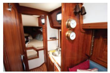
With the table stowed on the bulkhead, Sparkle Plenty's saloon, at left, is airy and spacious. The white laminate headliner replaced aging vinyl. A full-width head compartment, at right, separates the forward cabin from the saloon.
