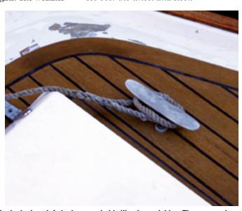
Scuffed with 100-grit sandpaper to give it a more "natural" look, the synthetic deck, at left, looks remarkably like the real thing. The preparation involved grinding the old deck surface. This left some areas damaged, at right, and they became the target of the next stage of the project.
