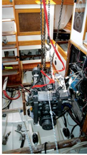
The engine in *Iron Mistress* can be extracted to allow access for inspecting and spot-blasting the bilge.
