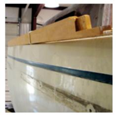
Stephen started fitting the toerails at the bow, at left. To bend the 10-foot lengths to the deck line, he used a handy billy, center and at right. After purchasing a plug cutter, Stephen used it prolifically, below, and plugged over the countersunk heads of the toerail bolts, at bottom.
