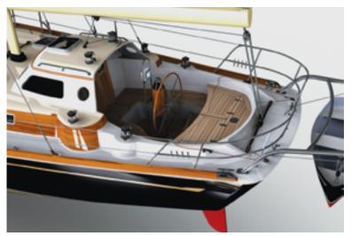
Bob used this rendering of a close-up of the cockpit to help the client understand the geometry of the house overhang on the 57-foot ketch shown above.
