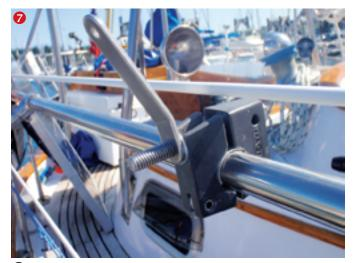
I positioned heavy-duty rail clamps, like those used on barbecue mounts, over the slots I'd cut in the 1-inch tubing. When these are tightened, they clamp the outer tube to the inner tube and hold the panel in the desired side-to-side position.
