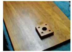
George chamfered the table's edges with a block plane, at left, mounted the hinges and clamps, center, and attached a socket for the leg, at right.
