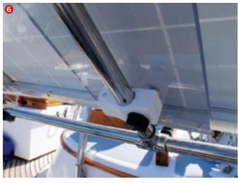
The new solar panels measured 26 x 40 inches. To mount them, I purchased two pieces of  $\frac{1}{2}$ -inch scrap acrylic sheet cut to 7 x 26 inches. I attached one to the back of each panel using machine screws with washers and nuts.
