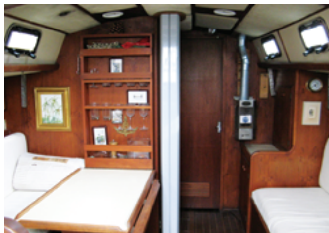
The view from the saloon looking aft, at left, shows a conventional arrangement with the chart table, quarter berth, and wet locker next to the companionway to starboard and the tight U-shaped galley to port. Forward, Duane installed a wood-burning stove to cheer up the already cozy cabin when cruising in the cool Pacific Northwest autumn, at right. The plywood bulkheads are bonded to the hull and deck for strength and stiffness.
