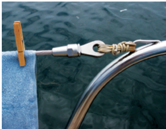
For the price of a handful of swageless rigging terminals, Dave and Connie McBride replaced Eurisko's doubtful lifelines with new ones made out of her old standing rigging.
