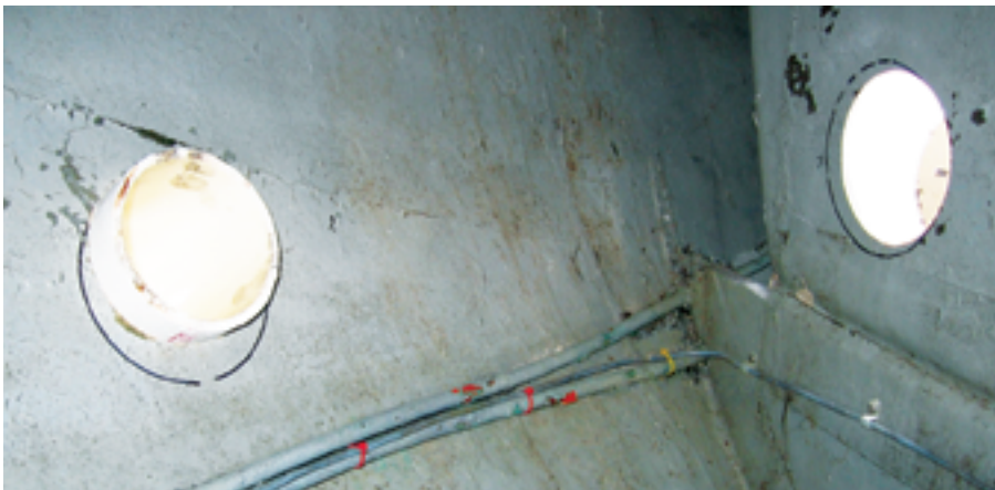
After cutting the holes in the cockpit side and the hull, John test fit the pipe that passes through the hull before marking it for cutting, at left. The trim ring on the cockpit side assures a solid installation and can be fitted with a cover if needed, at right.
