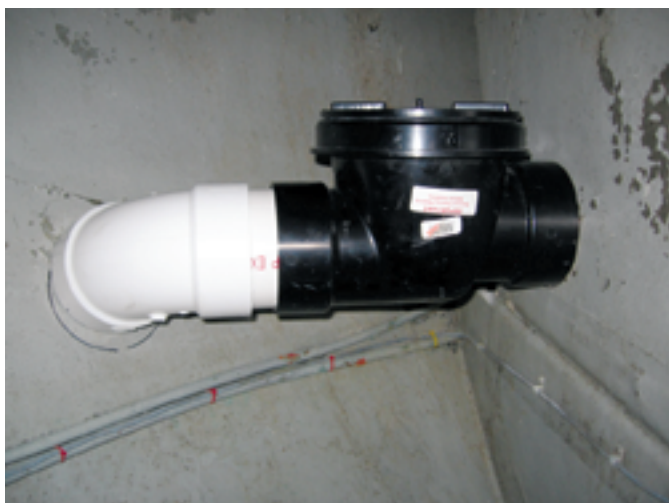
By dry-fitting all of the parts of his oversize scuppers, John ensured that they would slign properly and that he would cut the holes in the right places, at left. The new scupper cut in the cockpit side dwarfs the original cockpit drain, at right.
