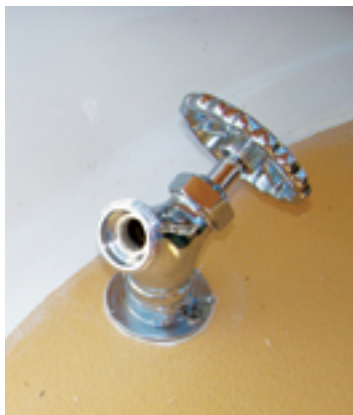
The wash-down plumbing leads to a standard hose bib under the foredeck grating, above. The pre-coiled hose is easy to stow, at right.
