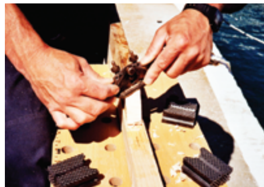
Richard used a spokeshave to round off the shoulder of the blade.
