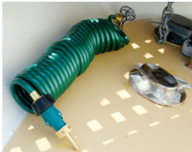
The wash-down plumbing leads to a standard hose bib under the foredeck grating, above. The pre-coiled hose is easy to stow, at right.
