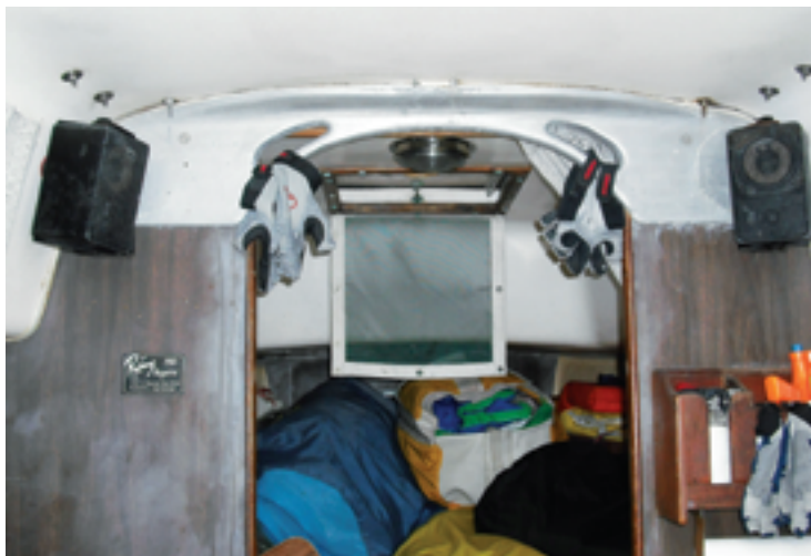
Amanda has the standard layout for a Morgan 24. A V-berth (here filled with sails) occupies the bow, at left. The galley is forward in the saloon and the settees extend under the cockpit as quarter berths, at right.
