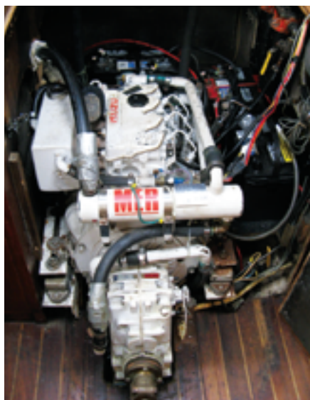
After years of fairly minor aggravations with the original engine, Duane repowered with a smaller Isuzu diesel. Removing the companionway steps provides access, at left. Fitted with lee cloths, the saloon settees make good sea berths, at right.
