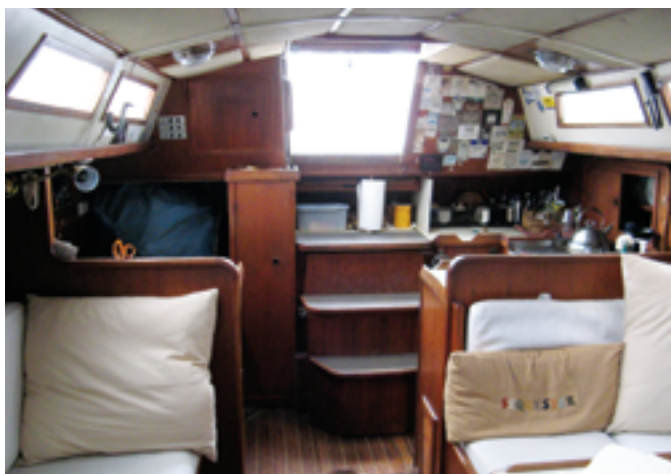
The view from the saloon looking aft, at left, shows a conventional arrangement with the chart table, quarter berth, and wet locker next to the companionway to starboard and the tight U-shaped galley to port. Forward, Duane installed a wood-burning stove to cheer up the already cozy cabin when cruising in the cool Pacific Northwest autumn, at right. The plywood bulkheads are bonded to the hull and deck for strength and stiffness.
