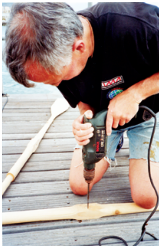
All but finished, the oars need only the means to attach them to the dinghy, above. Richard drilled holes for the bolts, at right, and cut recesses for washers with a spade bit, at top right. The shiny wooden oars lend Sigfrid's dinghy some much needed class, below.
