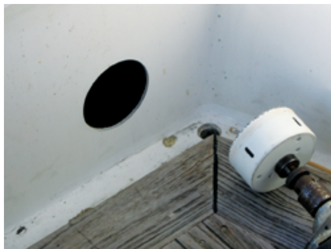
By dry-fitting all of the parts of his oversize scuppers, John ensured that they would slign properly and that he would cut the holes in the right places, at left. The new scupper cut in the cockpit side dwarfs the original cockpit drain, at right.
