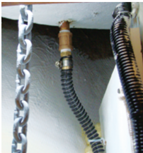
From the head intake, the wash-down supply hose passes through the bulkhead into the forward cabin, to a strainer, then to the pump, at left. The hose continues forward under the berth, at right, and into the chain locker, where it connects to the on-deck hose bib via a pipe extension, below.
