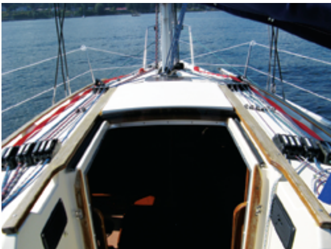
Sail-control lines are color coded, and with good reason; there are 15 rope clutches mounted on the cabintop, at left. The cast aluminum stemhead with its two bow rollers is a much-appreciated cruising feature but is unusual for a racing-oriented boat like the Arcadia, at right.
