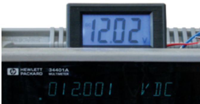
Tim tested the $10 eBay LCD voltmeter in the laboratory. It passed.
