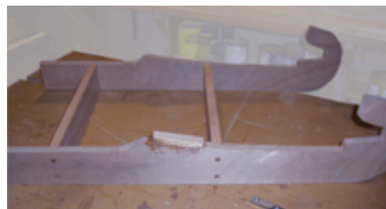
From index cards stapled together, Tony made cardboard patterns, top. Then he made the plywood upper stiles for the ladder, above.
