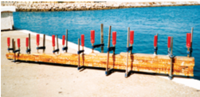
The laminating completed and the glue cured, the rough tiller awaits removal of the clamps, at left. To create the curve on the underside, Richard sprung a batten on the side of the tiller, drew along it with a marker pen, at right, then cut to the line with a jigsaw.
