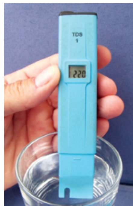
A digital TDS (total dissolved solids) meter provides a convenient means of testing the product water for purity.
