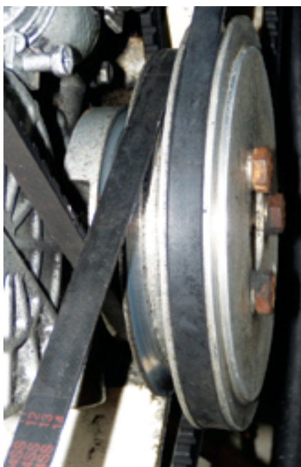
On Caribee , Randy fitted a double pulley on the engine to drive the watermaker (smaller pulley) and an alternator (larger pulley).
