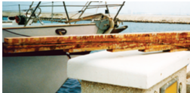
The laminating completed and the glue cured, the rough tiller awaits removal of the clamps, at left. To create the curve on the underside, Richard sprung a batten on the side of the tiller, drew along it with a marker pen, at right, then cut to the line with a jigsaw.
