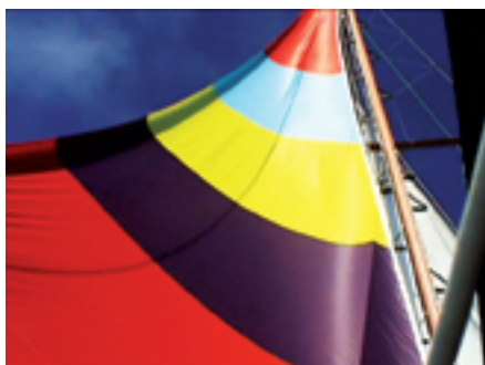
The Mainster has lines in its luff, leech, and foot with which to make the sail full or flat. Luff sag is not a problem when sailing off the wind.
