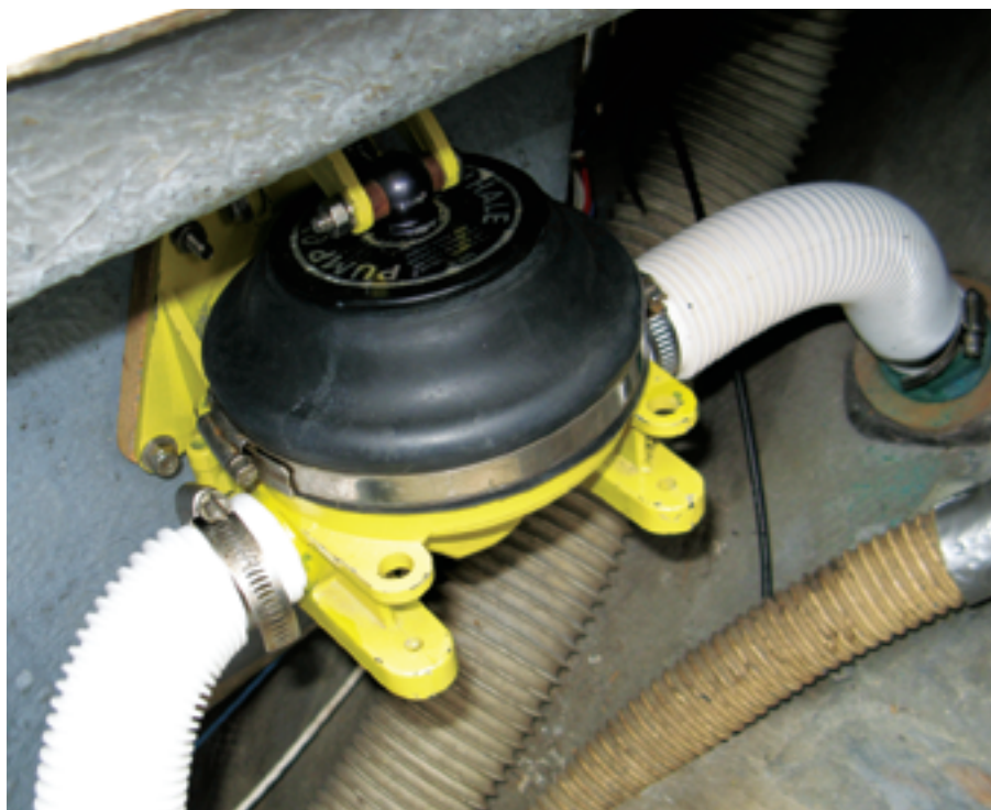
After being a notation on the "to do" list for several seasons, the bilge pump, finally refurbished, became a functioning part of Kuma's essential equipment.
