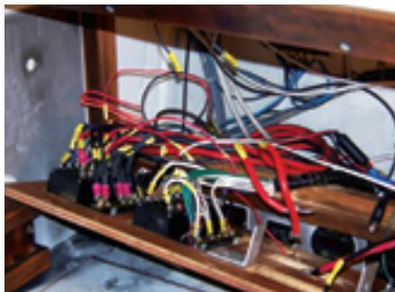
Because acidic smoke residues could cause problems down the line, the electrical panel, at left, had to be removed, cleaned, and rewired, at right.
