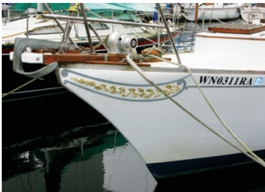
The anchor sprit Richard had installed complements the clipper bow and molded trailboards that give the Ericson Cruising 31 its characteristic appearance.
