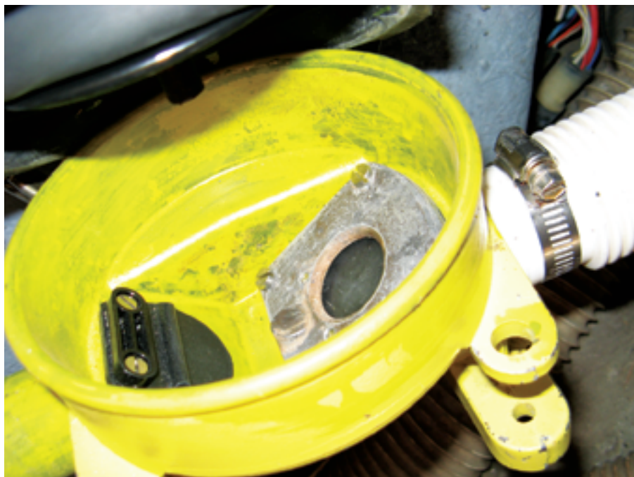
The body of the Whale Gusher bilge pump had years of life left in it but the valves had seized. Here, after reluctantly giving up its old valves, the pump's cast aluminum body has been given a coat of protective paint and the new valves are in place.
