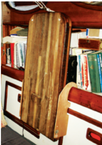
Dave can sit at his table with his back against the bulkhead. He left off the fiddle on the side of the table he faces so he can rest his arms on it as he works. When he's done, the table folds away against the settee back.
