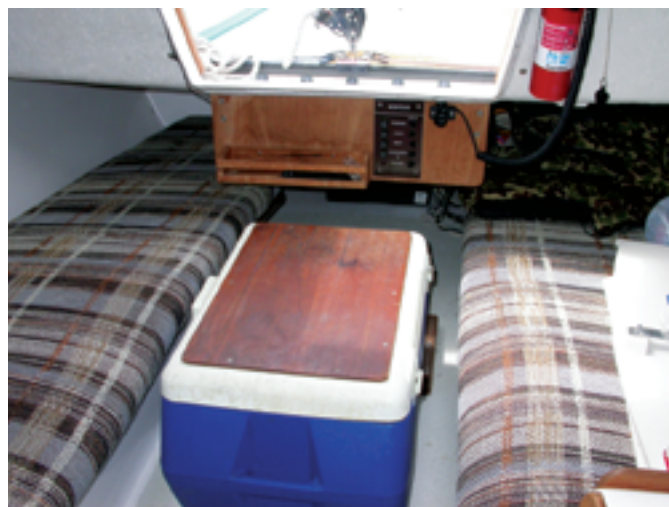
The V-berth occupies most of the area forward of the mast, which is supported by the compression post, at left. The center section of the V-berth can be removed to provide access to the portable toilet beneath. Two small countertops make up the "galley." At mealtimes, a removable tabletop fits between them to provide a larger work surface. A 50-quart cooler does double duty as a companionway step, at right.
