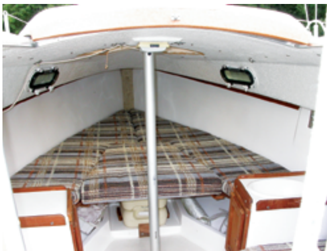
The V-berth occupies most of the area forward of the mast, which is supported by the compression post, at left. The center section of the V-berth can be removed to provide access to the portable toilet beneath. Two small countertops make up the "galley." At mealtimes, a removable tabletop fits between them to provide a larger work surface. A 50-quart cooler does double duty as a companionway step, at right.
