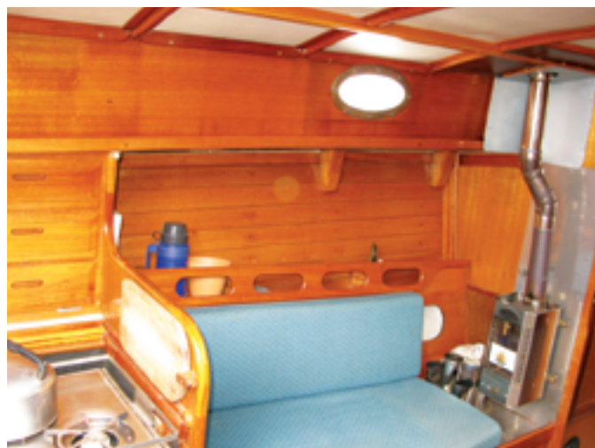
Ericson Yachts gave the interior of the Cruising 31 a cozy and classic feeling. It has abundant teak paneling and trim and a white overhead with wooden beams and grabrails. The solid-fuel heating stove is a season stretcher in Kuma's home waters.
