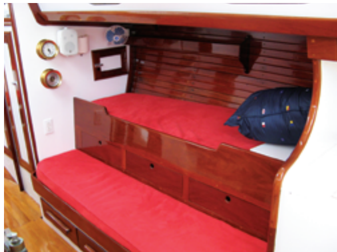
The galley is aft, and not particularly large for a 40-footer. Shortcomings include lack of counter space for food preparation and the icebox lid, which must do double duty as the chart table, at left. Pilot berths port and starboard make good sea berths or kids' berths. If there's just a couple aboard, they provide good stowage, at right.
