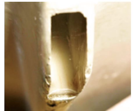
Because epoxy doesn't stick to it, the packing tape covering the foam blank left a nice finish on the inside of the wheel well.
