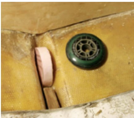
The foam blank used as a form to construct the wheel well was slightly larger in all dimensions than the wheel to be fitted.
