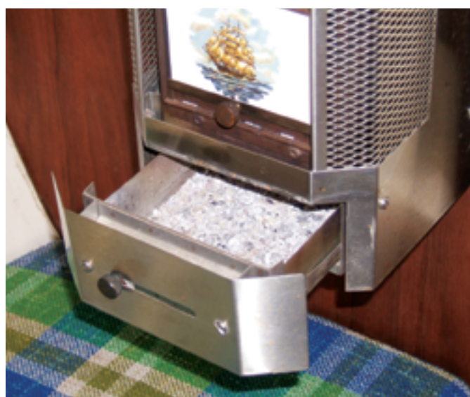
The firebox isn't very large but it puts out a lot of heat, top. Ashes collect in a convenient drawer, above.
