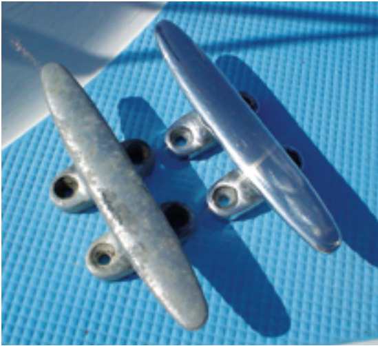
Aluminum deck cleats clean up nicely with a little judicious sanding, brushing and buffing, left and right. Stainless-steel gudgeons, below, also respond to TLC and will enhance the boat's appearance when re-installed.
