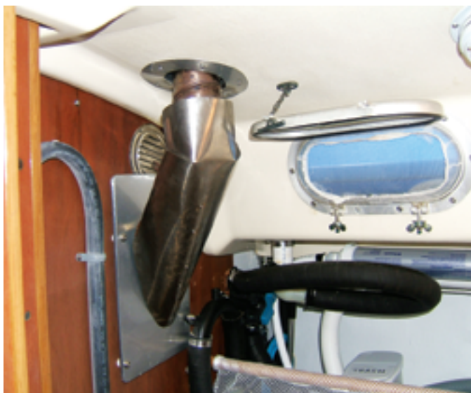
In the head, a heat shield around the flue saves scalps.
