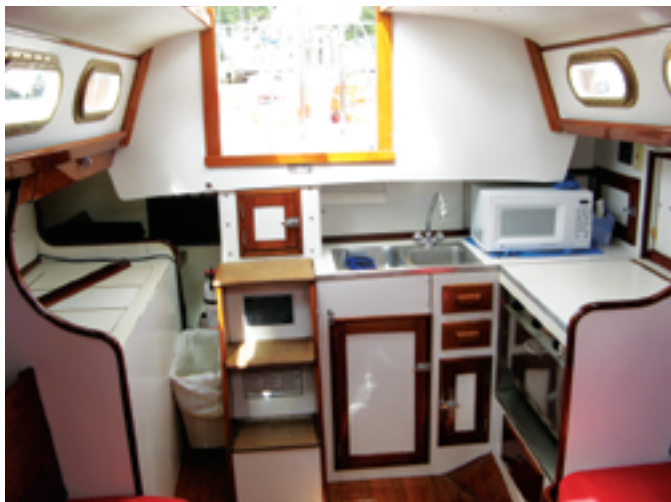
The galley is aft, and not particularly large for a 40-footer. Shortcomings include lack of counter space for food preparation and the icebox lid, which must do double duty as the chart table, at left. Pilot berths port and starboard make good sea berths or kids' berths. If there's just a couple aboard, they provide good stowage, at right.
