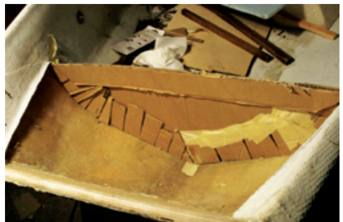
The new plywood former clamped and wedged in place during gluing, at left. The sprung wooden sticks are braced against blocks temporarily tacked in place. The foamed polyurethane glue is visible around the edge of the plywood former. The template for the seats consists of a large piece of cardboard roughly cut to shape with many little pieces attached to it to follow the interior contour, at right.
