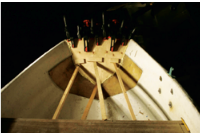
The new plywood former clamped and wedged in place during gluing, at left. The sprung wooden sticks are braced against blocks temporarily tacked in place. The foamed polyurethane glue is visible around the edge of the plywood former. The template for the seats consists of a large piece of cardboard roughly cut to shape with many little pieces attached to it to follow the interior contour, at right.
