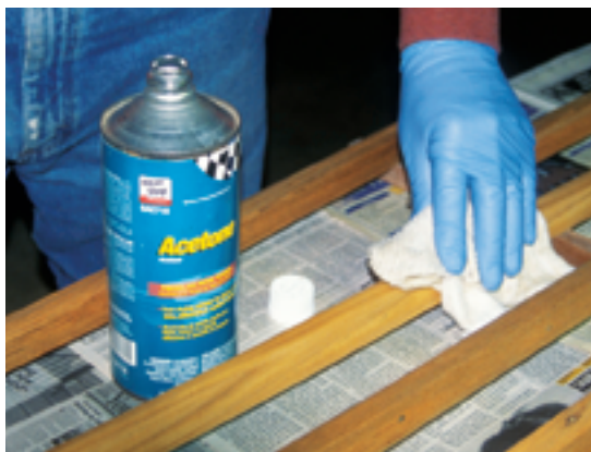
After removing the toerails from the boat, Gregg took off all traces of the old finish with a vibrating palm sander, far left. Wiping the smooth, uniform surface with acetone ensured that the parts were free of sanding dust, at left.
