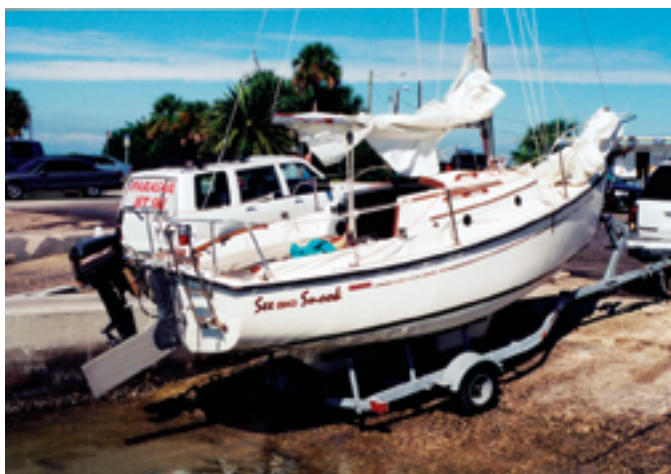
The Com-Pac 19 tows well behind most cars and is easily launched at a typical ramp, where the kick-up rudder, at left, lessens the risk of grounding. The V-berth, at right, is adequate for two adults although the compression post will come between them.
