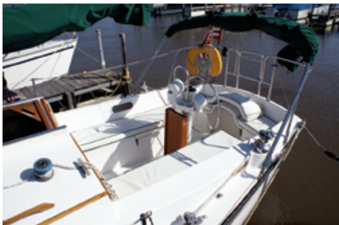
The T-shaped cockpit, at left, gives the helmsman room to move to the rail port and starboard to check sail trim, but the wheel and pedestal impede movement forward. That makes singlehanding difficult, because the mainsail sheet leads to a traveler on the cabin trunk. Charlie and Elaine Lawson, right, find their Newport 28 II well suited to their style of weekend and short-term cruising.
