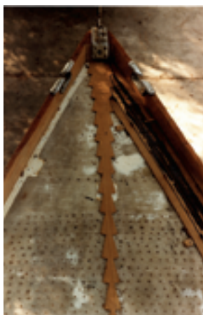
Part of Magnolia's makeover was a new teak deck, in process at left, and bronze opening ports to replace fixed windows, at right.
