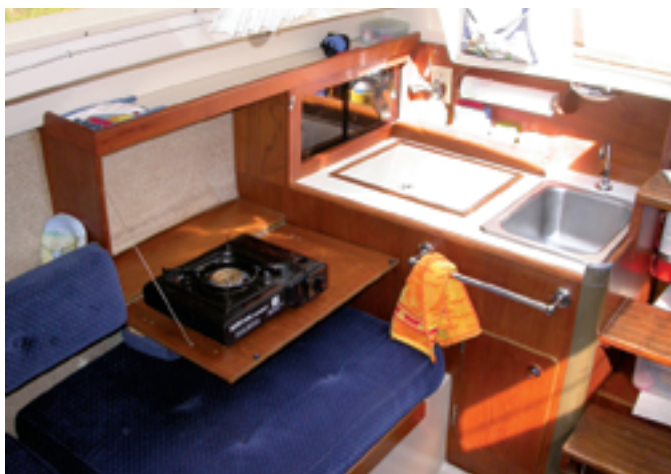
Aboard Martha J. , the cooking is done on a portable butane stove. It rests on a panel that folds down to expand the small galley work area, at left. The dinette table mounts on the main bulkhead. Fully opened, it seats four, at right. The starboard leaf folds back to allow passage forward.
