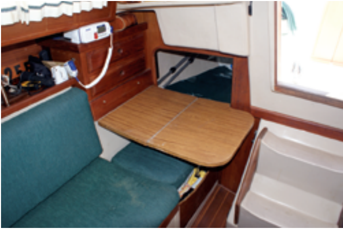
The navigator can communicate with the helm while working at the folding chart table over the head of the starboard quarter berth, at left. Access to the front of the engine is provided behind the companionway ladder, at right, and its top is exposed by a hatch in the cockpit.
