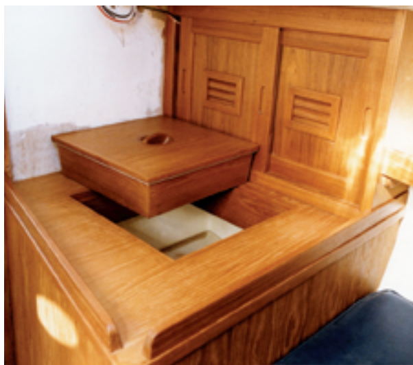
To solve the warm-beer problem, Paul built an efficient icebox (and extra lockers) where the head had been. Although it's in the forward cabin, it's conveniently adjacent to the galley counter.
