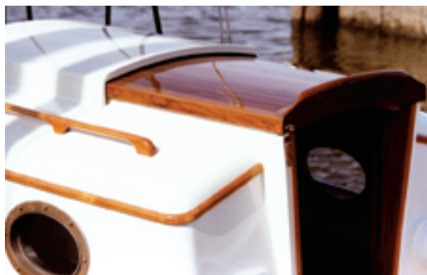
After stepping through the teak companionway hatch, Paul used its parts as patterns for constructing a new one, then built the sea hood to keep the sea on the outside.
