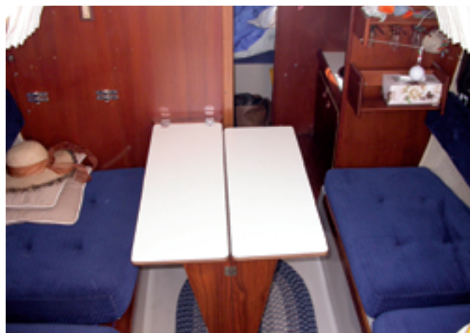
Aboard Martha J. , the cooking is done on a portable butane stove. It rests on a panel that folds down to expand the small galley work area, at left. The dinette table mounts on the main bulkhead. Fully opened, it seats four, at right. The starboard leaf folds back to allow passage forward.
