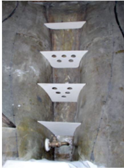
Checking the fit of the bulkheads and baffles.
