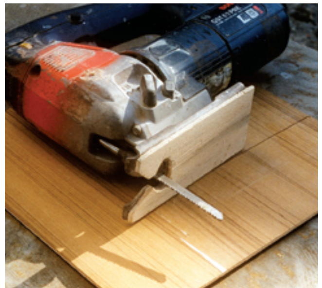
A shoe, made from a scrap of wood and glued with contact adhesive to the saw's foot, will prevent surface damage and scratching. This is particularly useful when cutting lumber that is already painted or varnished.
