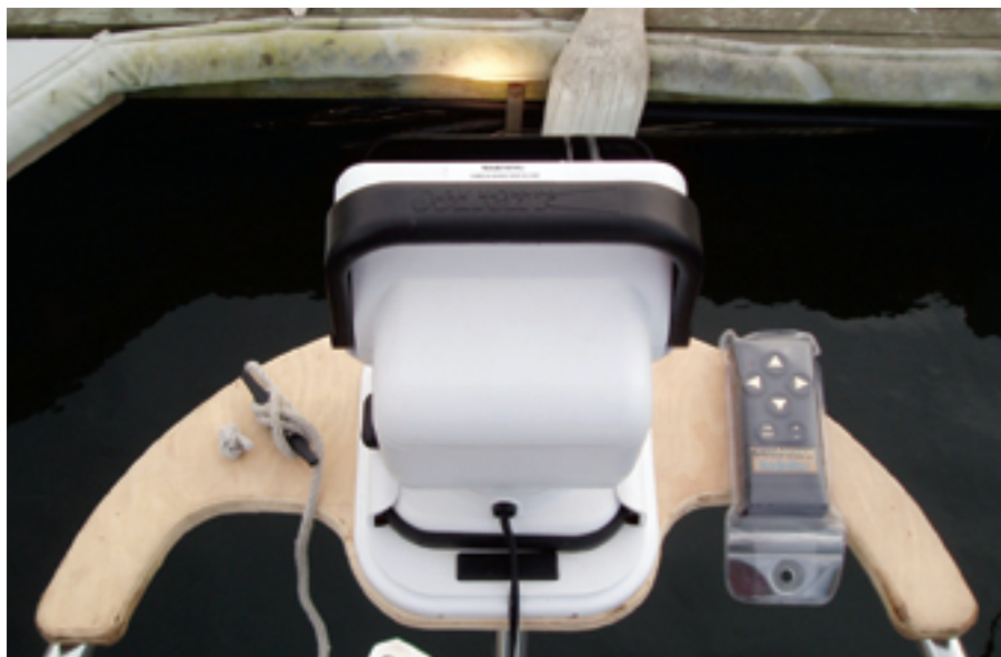
As well as swiveling through more than 360 degrees laterally, the searchlight beam rotates vertically. Depressed at this angle, it can shine on a mooring buoy.
