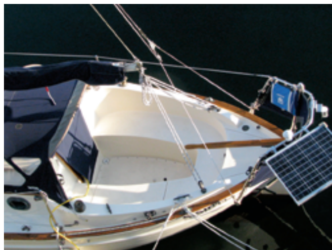
Because of the outboard rudder, the tiller takes up little room in Sisiutl's cockpit which, being compact, has seagoing potential. A solar panel helps keep the battery charged when the boat's at sea.
