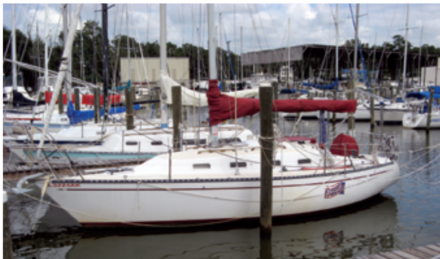
Wide sidedecks and inboard chainplates make for easy movement fore and aft. The double lifelines and pulpits are a bonus.
