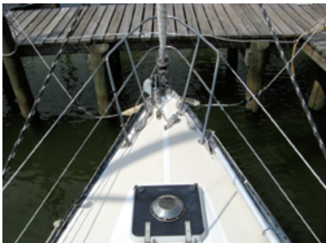
The bow has a fine entry. The ventilation hatch on the foredeck does not directly interfere with foredeck work, but the crew needs to be mindful of it, especially if the open hatch is covered by a doused sail.
