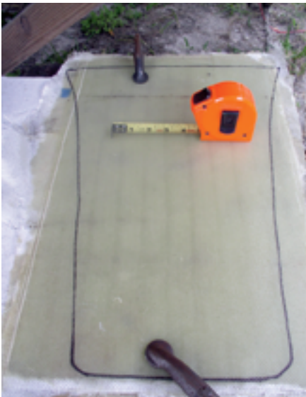
Drawing out the aft bulkhead.
