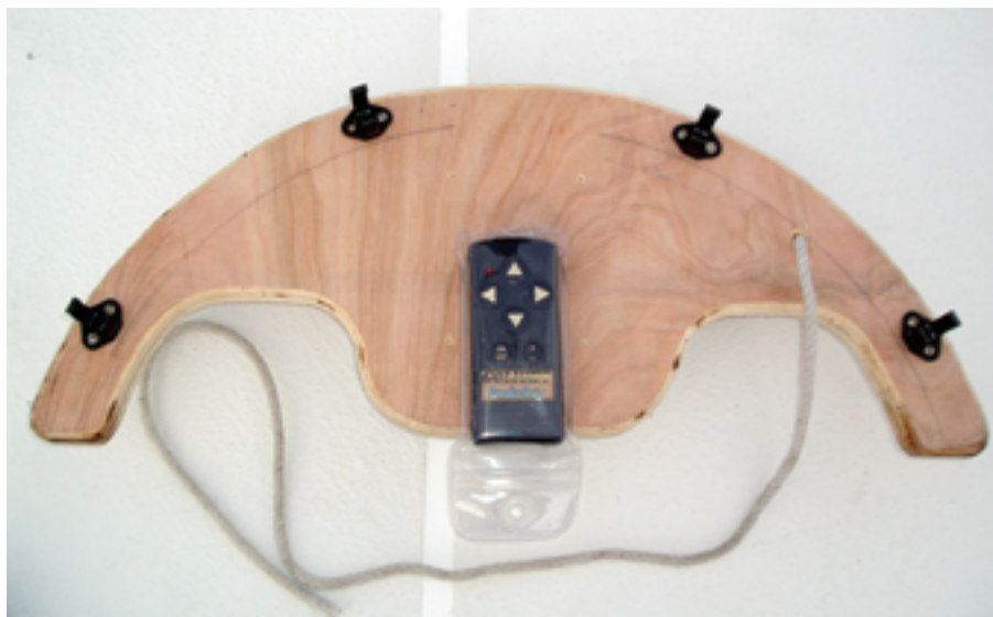
A view of the underside of the "boomerang" shows the clips with which it attaches to the bow pulpit and the "just in case" lanyard that keeps it there.
