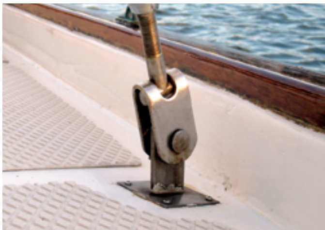
Flush with the deck, a chainplate invites leaks.
