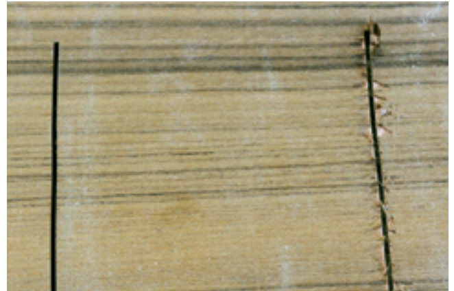
The damage to the teak veneer on the right-hand saw cut was caused by a conventional jigsaw blade cutting on the upstroke. The left-hand saw cut was made with an upside-down blade. In this case, the veneer was left intact.
