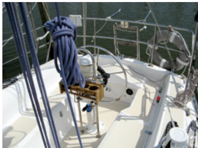
The spacious cockpit has a modified T shape, making it possible to get around the wheel without stepping up on the seats — a good safety feature. The heavy-duty mainsheet traveler is mounted on the bridge deck.
