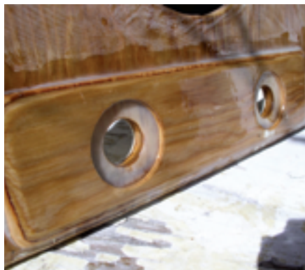
Creating a base for the plumbing fittings.
