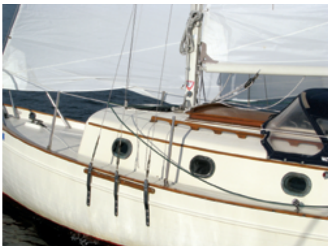
The roomy foredeck with its high bulwarks and the wide side decks contribute to crew safety, and the oversized chainplates convey an idea of the boat's ruggedness.
