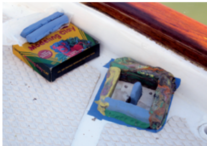
A mold of modeling clay defines the shape of an island of epoxy.
