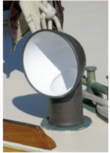
The louver vent to the cockpit locker, at left. The Nicro solar vent, above, pulls air through the spaces above and below the head door, helping to ventilate the rest of the boat as well. The chain locker in the forepeak lies just below a 4-inch cowl ventilator, at right.
