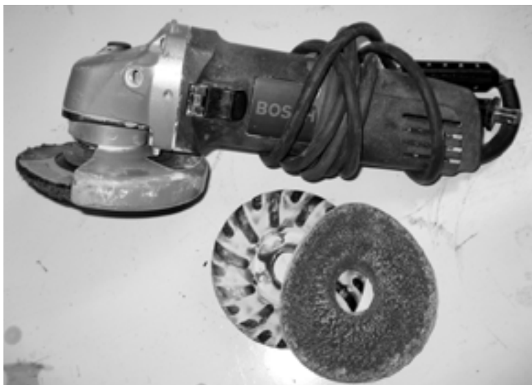
The Bosch 4½-inch grinder with sanding pad and 36-grit disc is a good choice for removing very heavy material.
