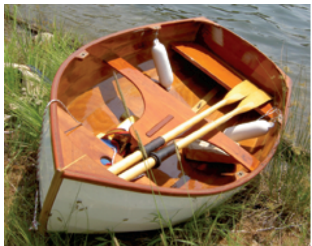
Nina's middle seat, extended to encompass the daggerboard trunk, adds both style and stiffness.
