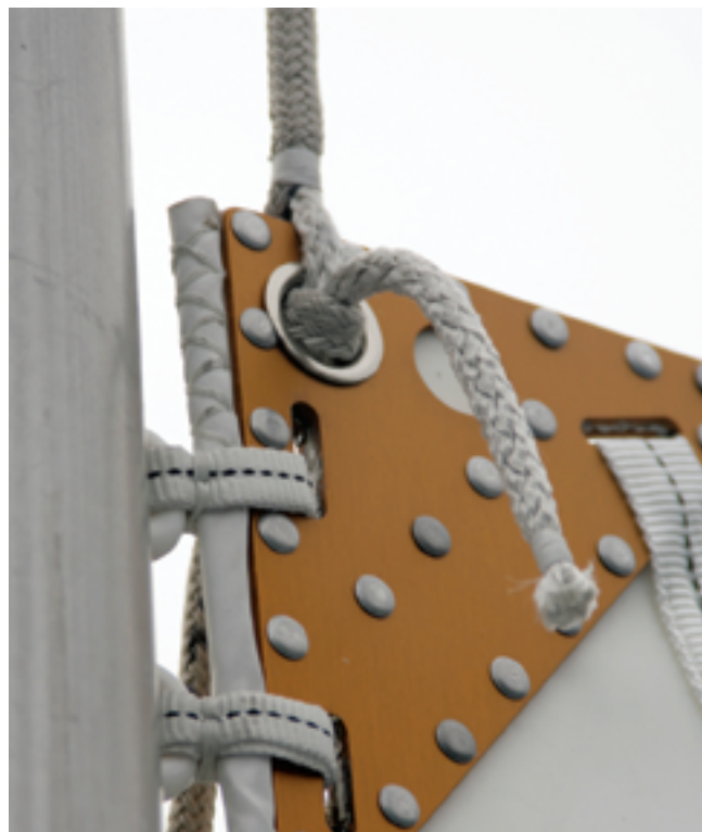
No need for a shackle at the head of this sail with the help of double-braided line and Paul's clever trick.
