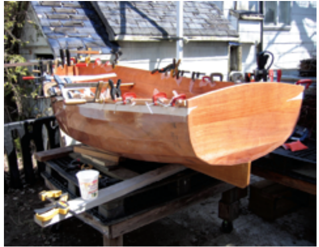
When it came time to fit the mahogany gunwale rails, Jonathon rounded up all the clamps in the neighborhood.
