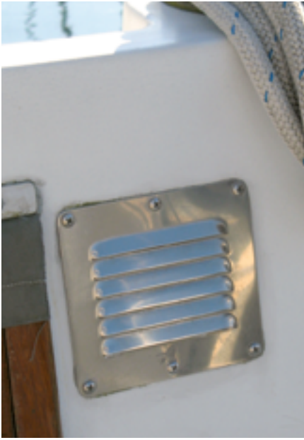
The louver vent to the cockpit locker, at left. The Nicro solar vent, above, pulls air through the spaces above and below the head door, helping to ventilate the rest of the boat as well. The chain locker in the forepeak lies just below a 4-inch cowl ventilator, at right.
