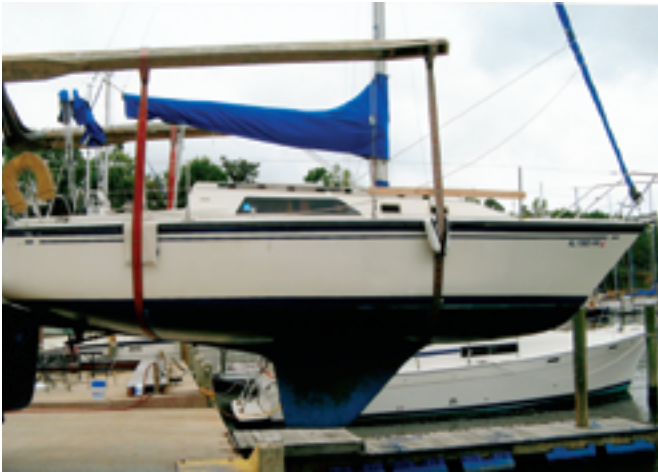
Hauled out for a scrub, the underwater profile of Liza's fin keel and spade rudder is revealed.
