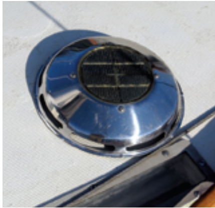
The louver vent to the cockpit locker, at left. The Nicro solar vent, above, pulls air through the spaces above and below the head door, helping to ventilate the rest of the boat as well. The chain locker in the forepeak lies just below a 4-inch cowl ventilator, at right.
