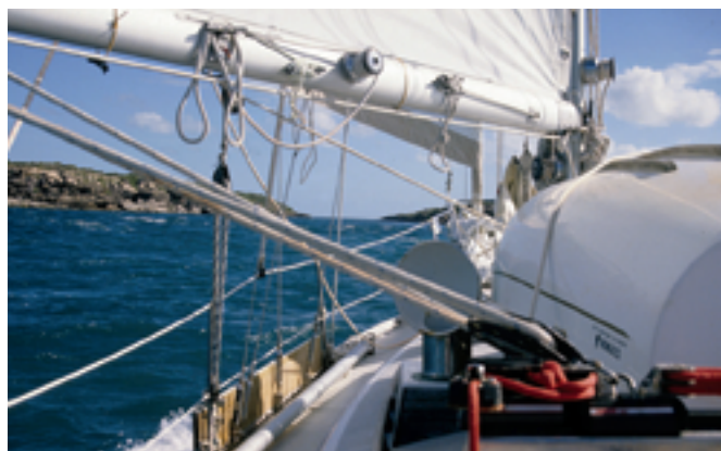
A block-and-tackle or vang strapped to the toerail makes an adequate and easy-to-use poor man's preventer.
