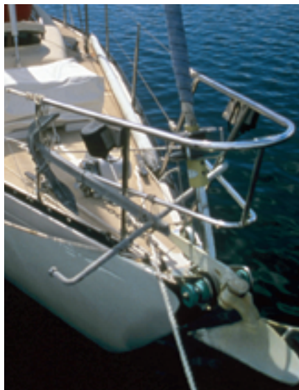
This 34-foot boat has a robust bow roller capable of holding a large anchor. Bow rollers can be retrofitted on many boats.
