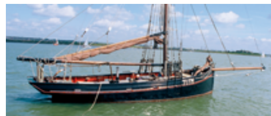
Old gaff-rigged cutters that once worked for a living are still commonly used as cruising boats in Great Britain. This well-maintained example cruises out of the River Medway in the Thames Estuary on the southeast of England.
