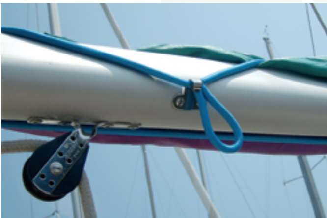
Starboard side of boom showing fender hook with the bungee hooked on.
