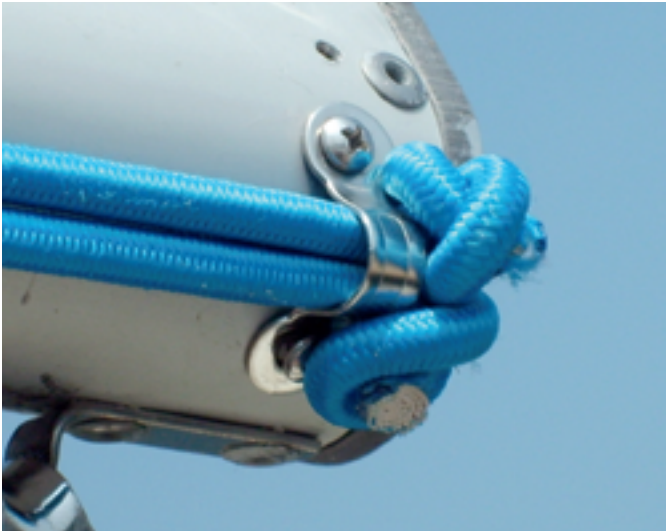
Aft end of boom showing the 5/16-inch eye strap securing two 1/4-inch bungee ends. The arrangement is the same at the other end of the boom.
