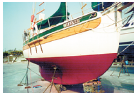
The Bristol Channel Cutter boasts a classic full-length keel characteristic of a 19th-century working boat. Many cruisers still value such keels for their directional stability and seakeeping ability.
