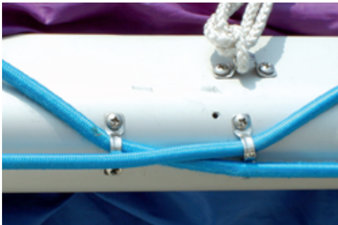
Port side of boom showing two 1/2-inch eye straps providing turning points for two bungees.
