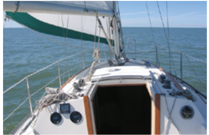
Sail controls are led aft to rope clutches and winches to either side of the companionway. Note the sea hood.
