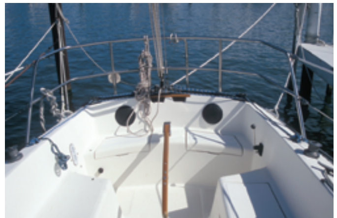
Mainsail sheeting is end-boom to a traveler across the transom.
