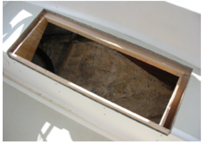
The drainage channels and framing are prepared for installation, top left. The drainage channels and framing ready for epoxy and fiberglass, top right. Looking aft from below with the drainage channels sealed in epoxy, at left. Facing page: The finished locker with the lid open, at left, and with lid closed, at right.
