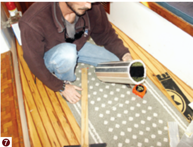
Single directional kerf cuts, above (7) for bending the Celotex. The finished aft cabin panels, (8).
