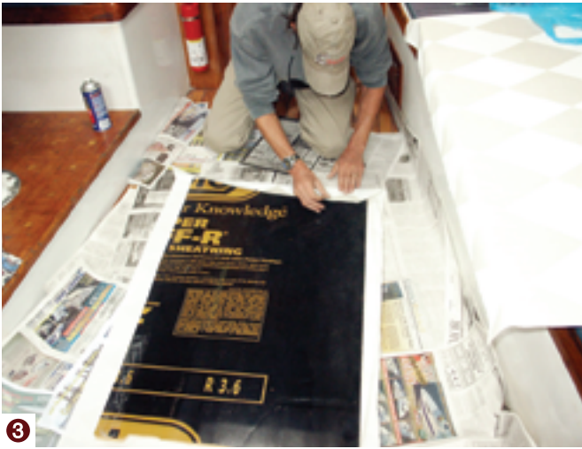
When the adhesive has set up, Dave folds the fabric covering over the Celotex, (3). The finished V-berth panels, (4).
