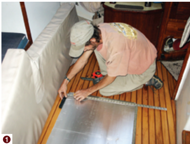
Dave cuts the Celotex to size for use in the V-berth, (1), and sprays the edges, (2), to create a tacky seal for the fabric covering.
