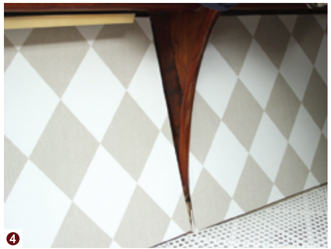
When the adhesive has set up, Dave folds the fabric covering over the Celotex, (3). The finished V-berth panels, (4).
