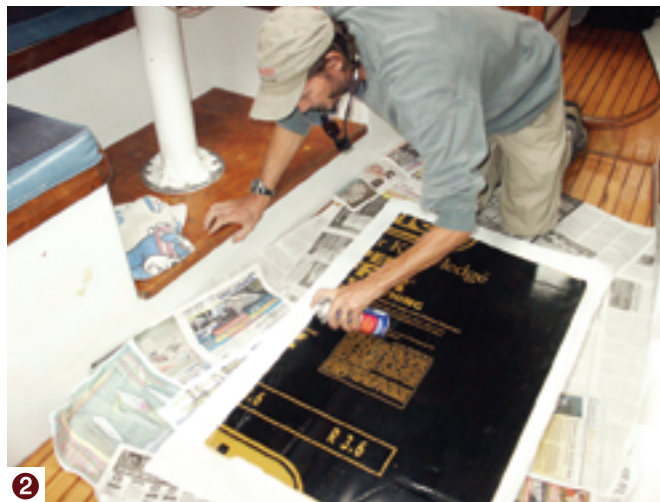
Dave cuts the Celotex to size for use in the V-berth, (1), and sprays the edges, (2), to create a tacky seal for the fabric covering.
