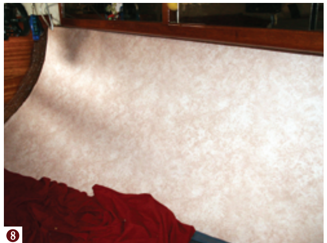
Single directional kerf cuts, above (7) for bending the Celotex. The finished aft cabin panels, (8).
