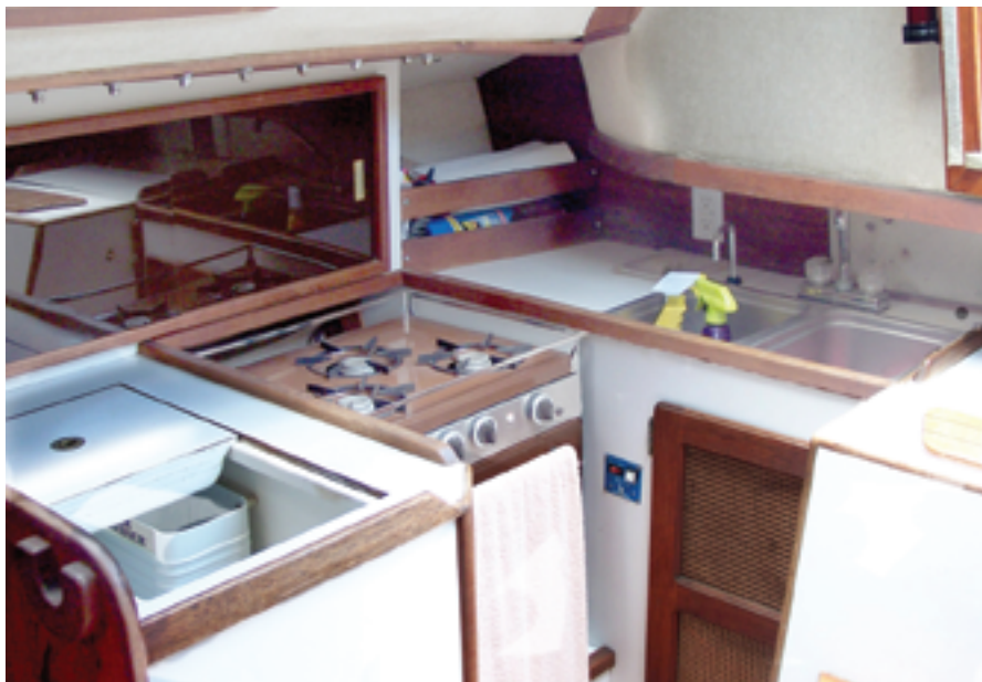
The galley is aft to starboard, with a double sink under the bridge deck, a three-burner gimbaled stove/oven, and icebox. There isn't much counter space.
