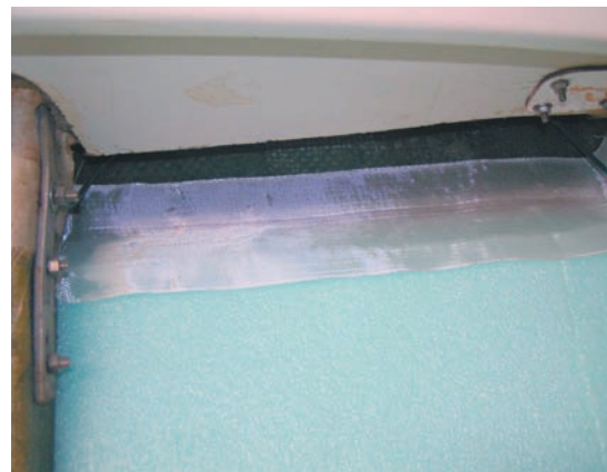
He pre-cut panels and beveled the tops to divert any leaks from the deck joint or toerail.
