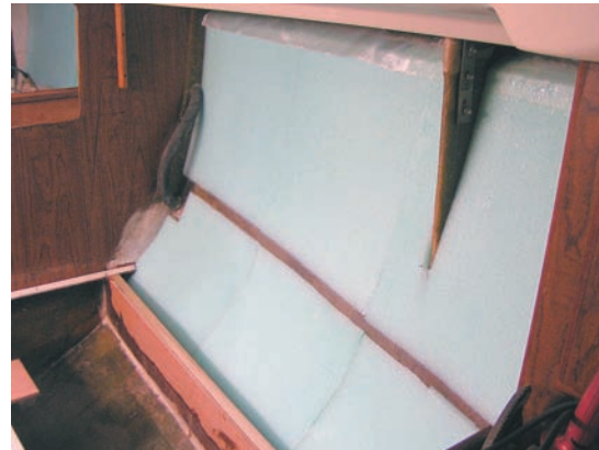
All panels were carefully fitted before Dale considered touching the contact cement can.
