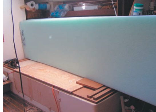
Dale chose Stratocell, easily cut with wood-working tools, as his insulation material.
