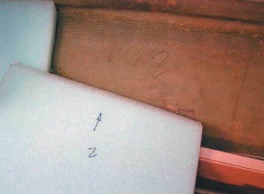
Since contact cement is unforgiving, Dale marked each piece with a name and an arrow.
