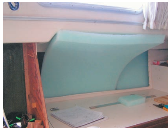
The flexibility of the material allowed it to bend to the hull and to be sprung into place.
