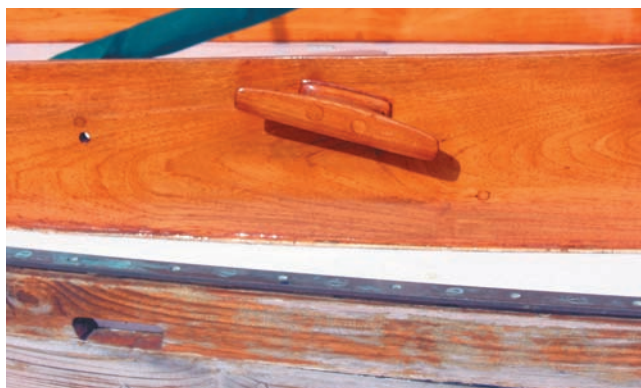
Detail of the finished coaming and the unfinished toerail.
