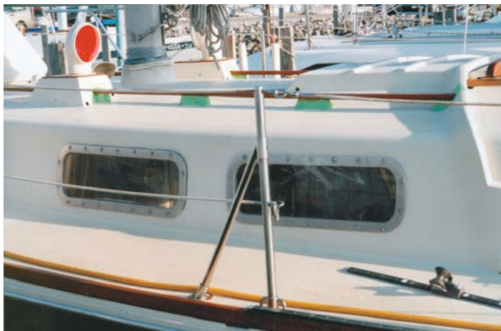
The leaking portlights on Steve's Tartan 30 were due for replacement.
