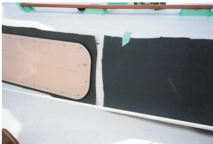
The new portlights are positioned over the gasket material and ready to be screwed down.
