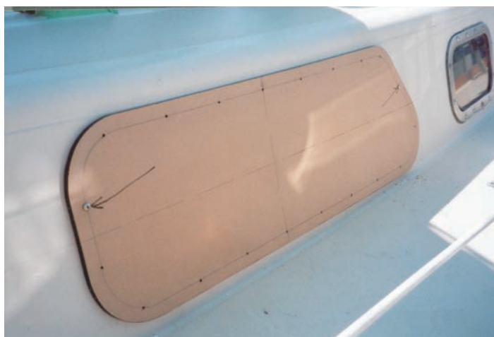
Steve used the portlight as a drill guide. Note the vertical and horizontal positioning guides. Locating screws are marked with arrows.
