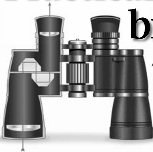
Porro prism, at left. Roof prism, at right.
