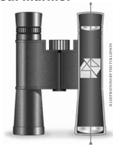
Porro prism, at left. Roof prism, at right.
