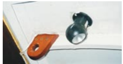
Detail of one of the mahogany blocks fastened to the cabin's rafter to hold one end.
