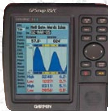
Chart plotter with graphical picture of tides, along with a listing of the times of high and low tides for the date selected
