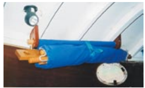
The Catnapper, rolled up and secured close to the overhead with Velcro on a nylon strap. The three H-frame pieces and the dowel for the foot are all rolled up in it. Note the reading spotlight above the right shoulder.
