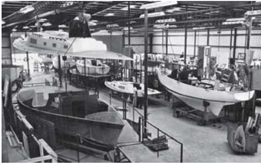
At Morgan Yachts' St. Petersburg, Florida, facility, men worked from scaffolding on boats of all sizes. Note how the decks were moved and positioned from overhead beams.
