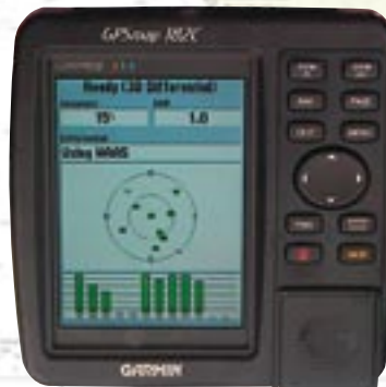
Chart plotter display, showing a sky view of the available satellites, with bar-graph of each satellite's receiving strength
