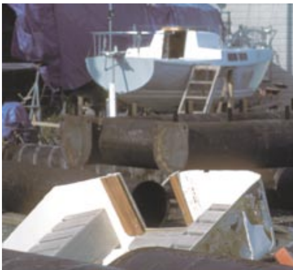
The cockpit gets cut out, above. Dave rides it to the dump, below left. The hull is gutted, below right, and gets sanded back to clean glass.
