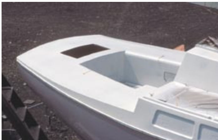
The new, aft, thwartship bulkhead, above. The cockpit getting primed for paint, at right. Note the wide gunwales and the stern deck with its hatch (not installed). Installing deck hardware, below.
