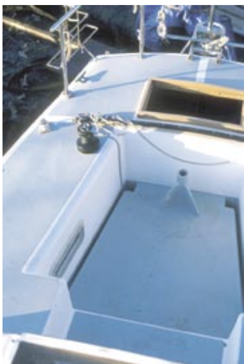
The new, aft, thwartship bulkhead, above. The cockpit getting primed for paint, at right. Note the wide gunwales and the stern deck with its hatch (not installed). Installing deck hardware, below.
