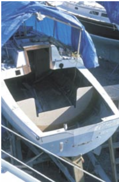
The new, aft, thwartship bulkhead, above. The cockpit getting primed for paint, at right. Note the wide gunwales and the stern deck with its hatch (not installed). Installing deck hardware, below.
