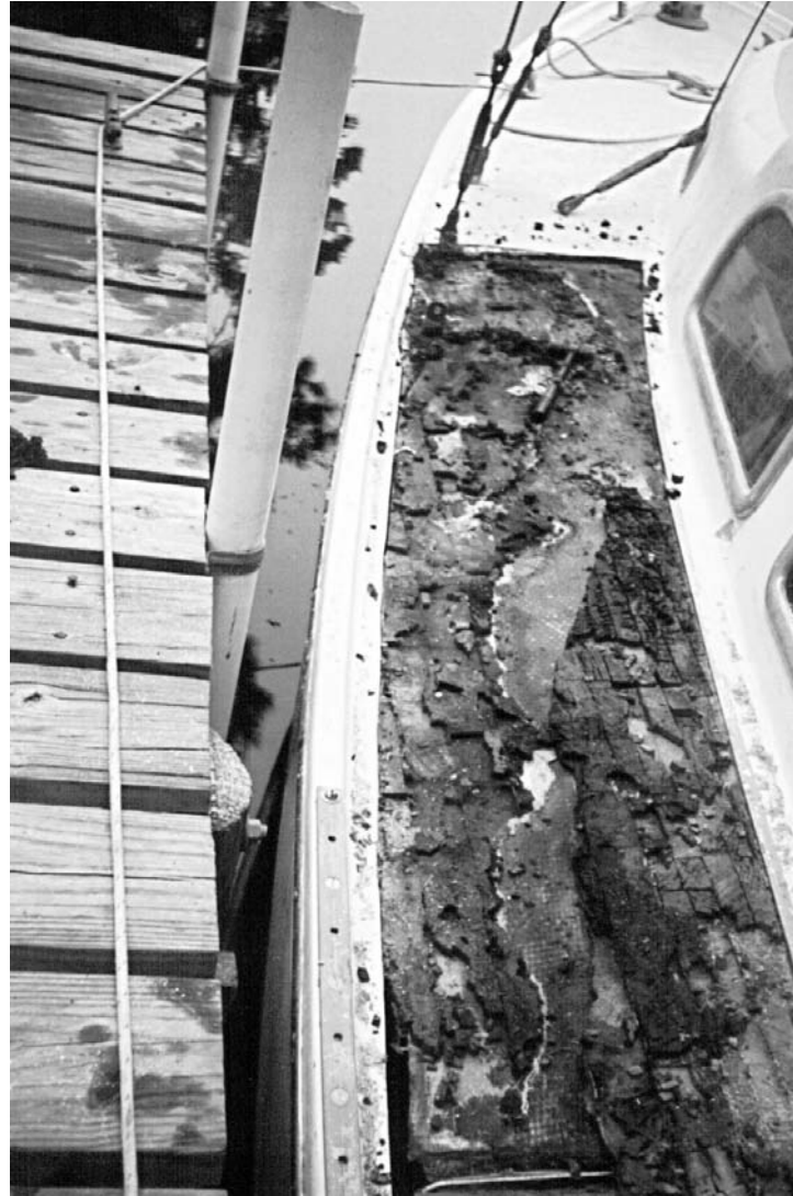
The rotted core just below the fiberglass was not a pretty sight.
