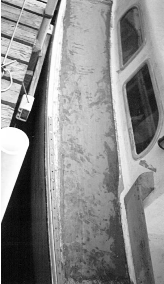
The new core was installed on the side deck.
