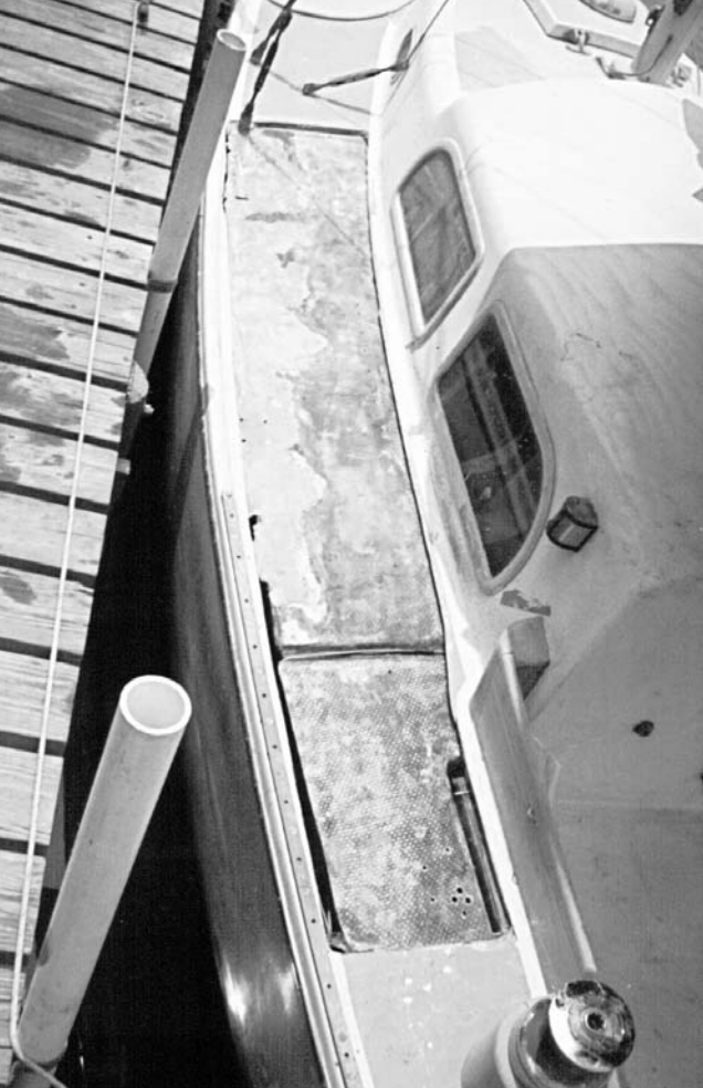
The side deck was cleaned, sanded and ready for a new core.
