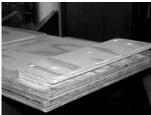
A plywood lip under the hatch crossbar holds the front of the hatch down.
