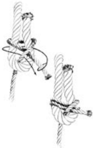
The reversed-lead sheet bend, shown above and also in the May issue, is not as reliable as the right-handed sheet bend.
