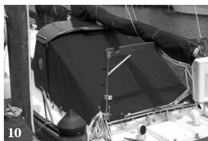
8 – The completed dodger with fabric sides. The top of the old Sunbrella dodger is cut off and the side fabric is saved as side panels. Dacron or vinyl awning rope is sewn to the edge of the fabric. The awning rope slides into an aluminum or vinyl awning track that is fastened to the underside of the hard-top.
