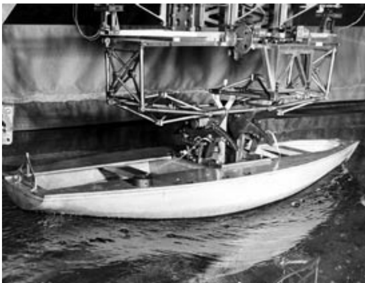
Tank testing the scale model of the Sabre 28 at the Stevens Institute of Technology in 1969.
