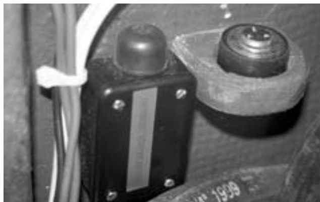
Don's emergency starter switch is located inside his engine compartment next to the runaway plug, discussed in the July 2003 issue of Good Old Boat .
