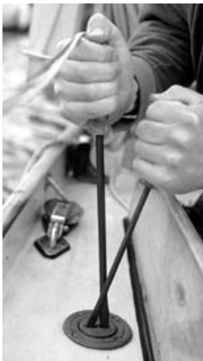
A second screwdriver increases the leverage on slotted deck-filler caps.
