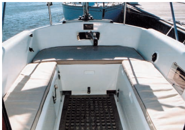
A large cockpit, at right, both isolates and protects voyagers from the elements. The floor grating protects the top of the fuel tank, immediately below it. Pagan Knight, at left, shows the Nick 31 profile.
