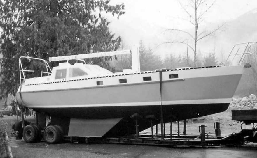
Toussaire, a 38-foot steel bilge fin motorsailer with 4-foot draft.
