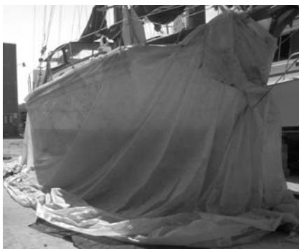
The bottom of Don's boat before the soda-blasting operation, at left. A plastic tent, center, is built around the boat's hull. At right, the hull is now down to the bare gelcoat and is slightly abraded, making it an ideal painting surface. It is now ready for a barrier coat and bottom paint or bottom paint only.
