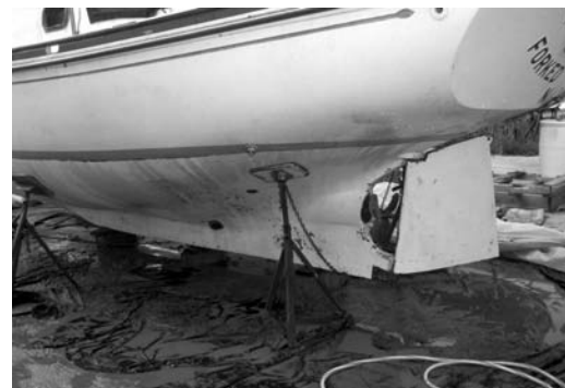
The bottom of Don's boat before the soda-blasting operation, at left. A plastic tent, center, is built around the boat's hull. At right, the hull is now down to the bare gelcoat and is slightly abraded, making it an ideal painting surface. It is now ready for a barrier coat and bottom paint or bottom paint only.
