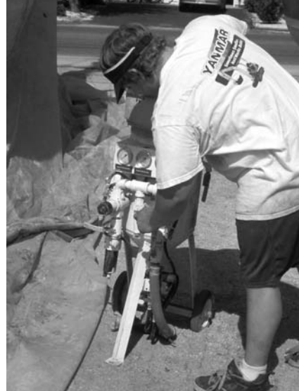
The operator connects his hoses to the soda-blasting equipment.
