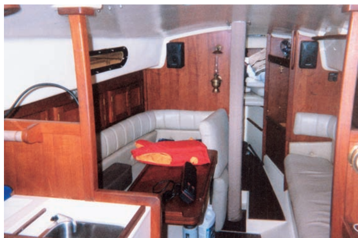
Headroom in the Contessa varies from 6 feet 1 inch to about 5 feet 10 inches. Views here are of Gerry and Allan Hodge's Contessa , at left, and Richard Whitehouse's Ceres , at right. Both are J. J. Taylor boats and show that builder's trademark fiberglass interior moldings trimmed with wood.
