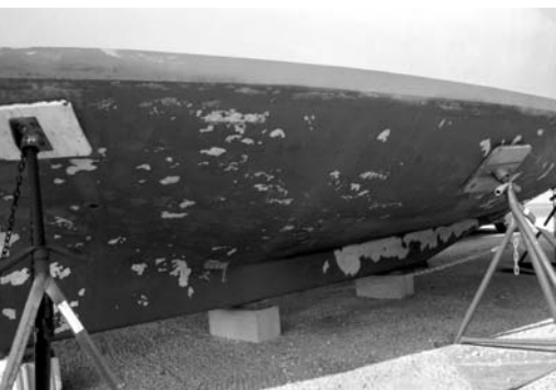
The bottom of Don's boat before the soda-blasting operation, at left. A plastic tent, center, is built around the boat's hull. At right, the hull is now down to the bare gelcoat and is slightly abraded, making it an ideal painting surface. It is now ready for a barrier coat and bottom paint or bottom paint only.
