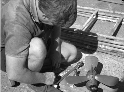
Assembling an Autostream self-feathering propeller.
