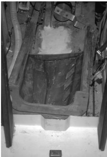
Before and after: preparations for the installation of a smaller Beta Marine engine in a C&C 30 required a new engine bed and oil drip pan to be constructed. This boat began life with an Atomic 4 which was later replaced by a Bukh and finally the Beta.
