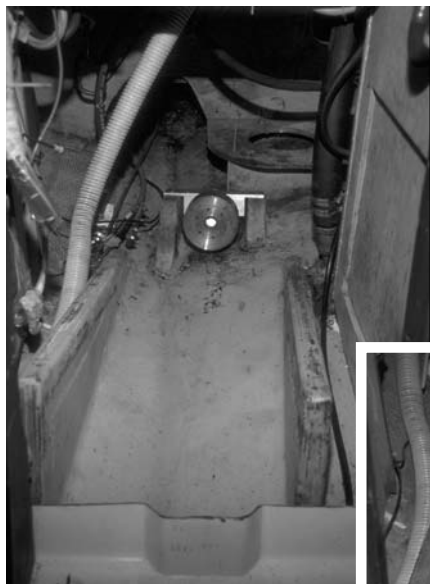
Before and after: preparations for the installation of a smaller Beta Marine engine in a C&C 30 required a new engine bed and oil drip pan to be constructed. This boat began life with an Atomic 4 which was later replaced by a Bukh and finally the Beta.
