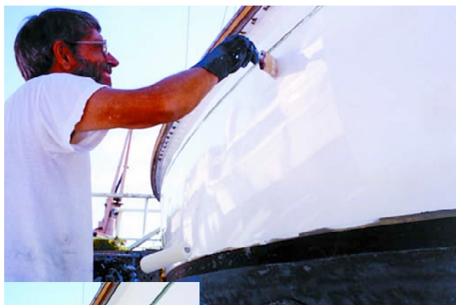
Tipping out the paint. Note the roller in the other hand. The pay-off: Don rolls out the paint.
