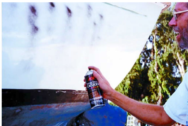
Misting the paint with contrasting lacquer aids in seeing where you have sanded.
