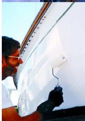
Tipping out the paint. Note the roller in the other hand. The pay-off: Don rolls out the paint.
