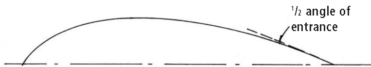
Asymmetrical Hull The modern form. Half angle of entrance is under 25 degrees, usually well under.
