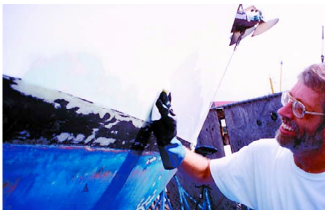
Solvent wiping in a downward sweep. The hull was wiped completely prior to sanding.
