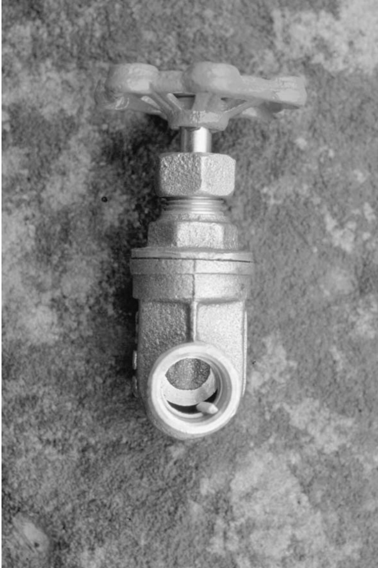
Gate valve stuck open by debris. Note that the handle does not indicate whether the valve is open or closed.
