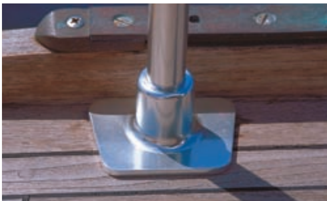
One-part base from start to finish, above, and installed on Ron's boat, at right.
