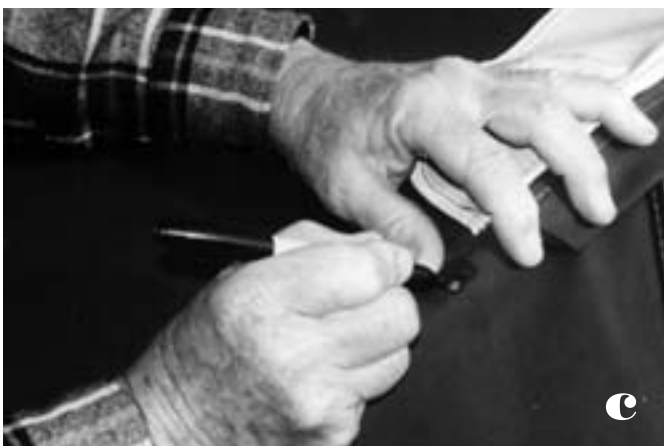
a) Marking the handle position on the fabric, b) Burning a hole through the fabric at the marked location, c) Marking the stainless steel frame through the hole in the fabric, d) With the fabric removed, drilling 1/4-inch holes through the frame, e) Mounting the handles and rubber gaskets, and f) Using wing-nuts on the inside of the dodger to make disassembly easier.
