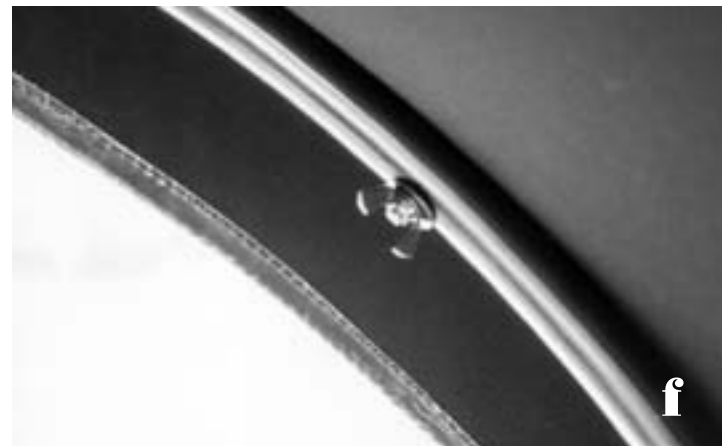
a) Marking the handle position on the fabric, b) Burning a hole through the fabric at the marked location, c) Marking the stainless steel frame through the hole in the fabric, d) With the fabric removed, drilling 1/4-inch holes through the frame, e) Mounting the handles and rubber gaskets, and f) Using wing-nuts on the inside of the dodger to make disassembly easier.
