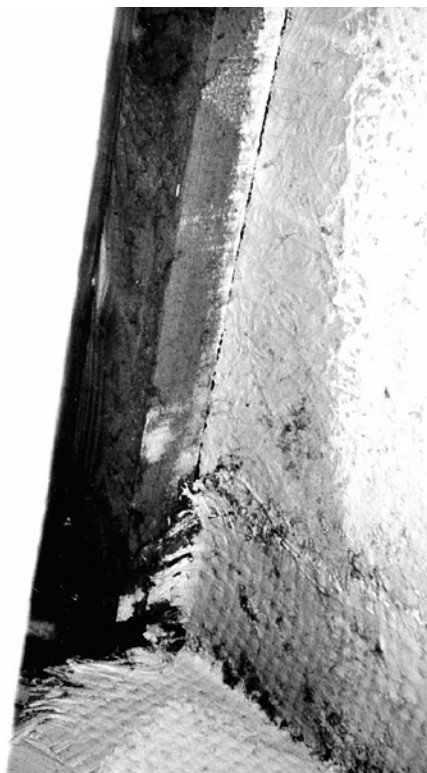
Naked structural wood next to poorly laid up roving tabbing. You can see the crack between the wood and the FRP already. It will only get worse.
