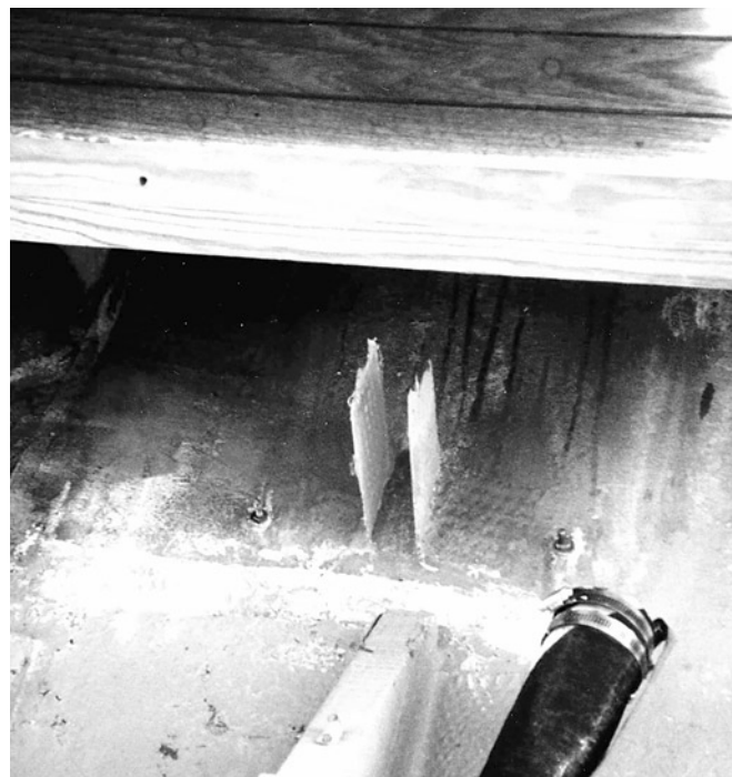
A total secondary bond failure. This builder tabbed uncoated wood beams to the hull without any prep, mechanical fasteners, or fillets.
