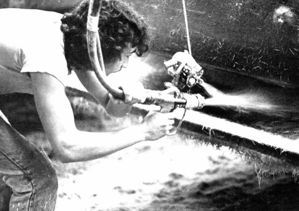
Chopper gun in use. At the very least, this worker should be wearing goggles and a respirator. Skin protection is also important. (Photo courtesy of Owens-Corning Fiberglass Corp.)
