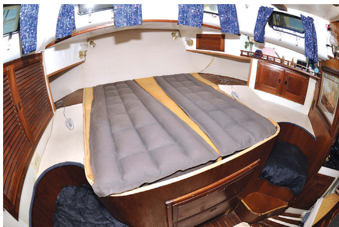
New bucket seats, above left, provide a step up to the bed, which is high to accommodate the steering gear beneath. Roger fitted pinrails to new shelves he built, above right. Foam inserts wedge individually inflatable commercial air mattresses in place, below.
