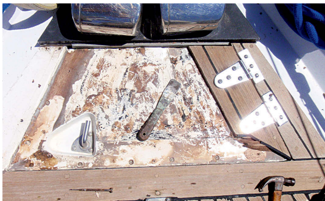
The anchor locker hatch offered an opportunity to test the feasibility of removing the teak decking, above left. The fiberglass deck under the teak was sound enough to stand alone, above right. Terry's first step in the main project was to cut around the screws, below.
