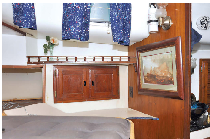
New bucket seats, above left, provide a step up to the bed, which is high to accommodate the steering gear beneath. Roger fitted pinrails to new shelves he built, above right. Foam inserts wedge individually inflatable commercial air mattresses in place, below.
