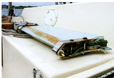
Cliff honed his shipwright skills on the dock in Newport, Rhode Island, at left, building a replacement rudder for his Sea Witch after failure #2. In event #3, Pelorus' rudder sheared off at the lower pintle, center. Event #4 was the result of a corroded pintle pin, at right.
