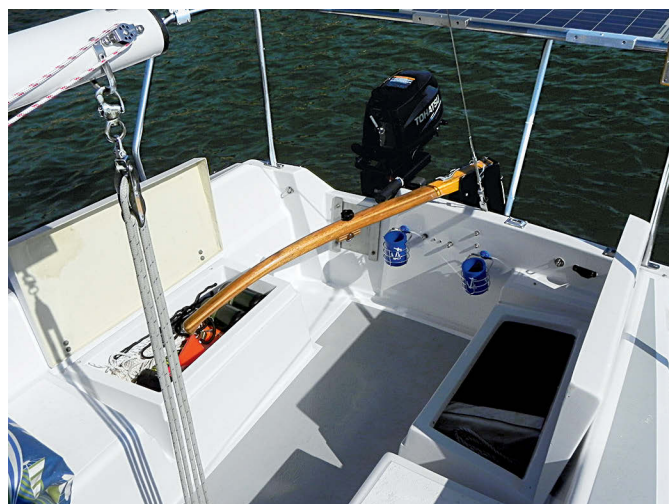
The cockpit has room for four adults on seats that are comfortable when the boat is upright but less so when heeling, at left. The aft end of the starboard seat is short to allow space for a fuel tank. Shallow lockers under both seats provide stowage for deck gear, at right.
