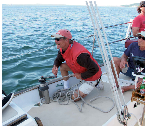
Mike fitted a bench across the stern where guests can sit comfortably away from the action yet have a good all-around view, at left. The sheet winches, mounted outboard of the wide cockpit seats, are a little awkward to use, at right, and preclude fitting a lower lifeline.
