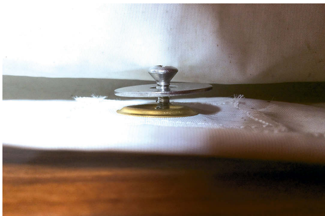
Fiona anchored the leecloth to the berth flat with wood screws, at left, sandwiching the grommets under fender washers, at right.
