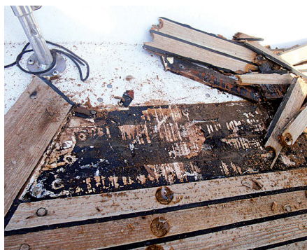
The farthest outboard teak planks were set in a white bedding compound and came up quite easily, at left. As Terry worked his way inboard, he found a tar-like compound that was much stickier, center. The teak from then on broke off in smaller pieces, at right.
