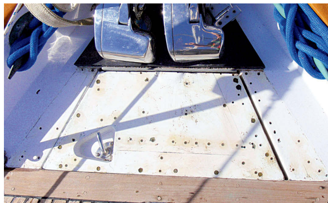
The anchor locker hatch offered an opportunity to test the feasibility of removing the teak decking, above left. The fiberglass deck under the teak was sound enough to stand alone, above right. Terry's first step in the main project was to cut around the screws, below.
