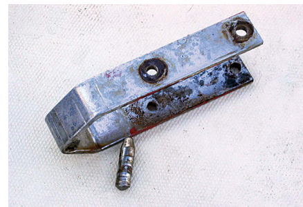
Cliff honed his shipwright skills on the dock in Newport, Rhode Island, at left, building a replacement rudder for his Sea Witch after failure #2. In event #3, Pelorus' rudder sheared off at the lower pintle, center. Event #4 was the result of a corroded pintle pin, at right.
