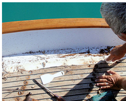
The farthest outboard teak planks were set in a white bedding compound and came up quite easily, at left. As Terry worked his way inboard, he found a tar-like compound that was much stickier, center. The teak from then on broke off in smaller pieces, at right.
