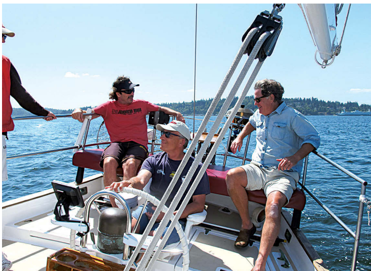
Mike fitted a bench across the stern where guests can sit comfortably away from the action yet have a good all-around view, at left. The sheet winches, mounted outboard of the wide cockpit seats, are a little awkward to use, at right, and preclude fitting a lower lifeline.
