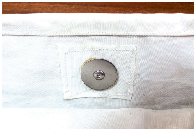
Fiona anchored the leecloth to the berth flat with wood screws, at left, sandwiching the grommets under fender washers, at right.
