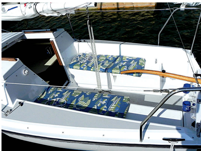
The cockpit has room for four adults on seats that are comfortable when the boat is upright but less so when heeling, at left. The aft end of the starboard seat is short to allow space for a fuel tank. Shallow lockers under both seats provide stowage for deck gear, at right.
