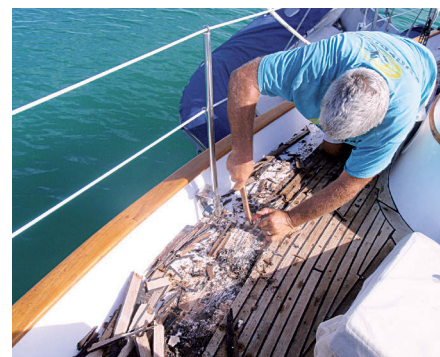
The farthest outboard teak planks were set in a white bedding compound and came up quite easily, at left. As Terry worked his way inboard, he found a tar-like compound that was much stickier, center. The teak from then on broke off in smaller pieces, at right.
