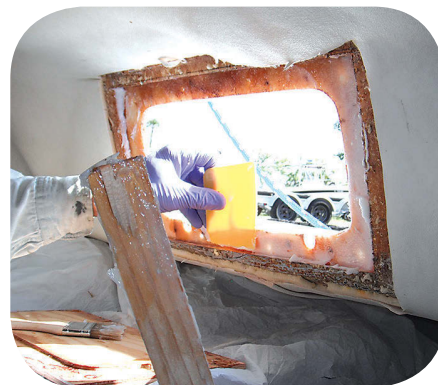
After removing a portlight and cleaning up the area, Dave cut a 1¼-inch-wide rabbet around the inside of the hole, at left, into which he would fit a plywood insert, center, with a matching rabbet to fit in the opening. He glued the plywood in place with epoxy, at right.
