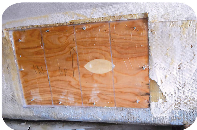
After coating the rabbets with epoxy, Dave screwed the plywood in place from the outside, using holes he’d pre-drilled for the purpose, at left. The kerfs, filled with epoxy, are visible in the plywood. The outside face of the plywood was flush with the cabin side, at right.
