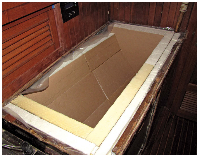
The insulation is two layers of 2.4-inch-thick polyurethane foam, at left. The inner box, at right, is lined with white laminate. David would place it inside the insulated cavern once he had fitted the divider, sealed all the inside corners, and installed the cold plate in the freezer.
