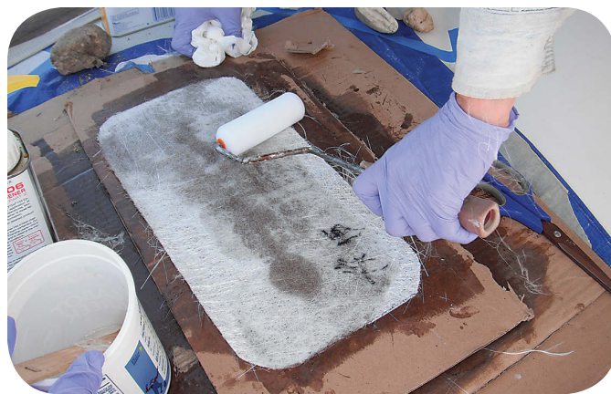
After rounding the square corners of the cut pieces, Dave laid them out so he could pick them up in the sequence — largest to smallest — in which he would use them, at left. Mat holds its shape well enough when wet that Dave could pre-wet it before placing it, at right.
