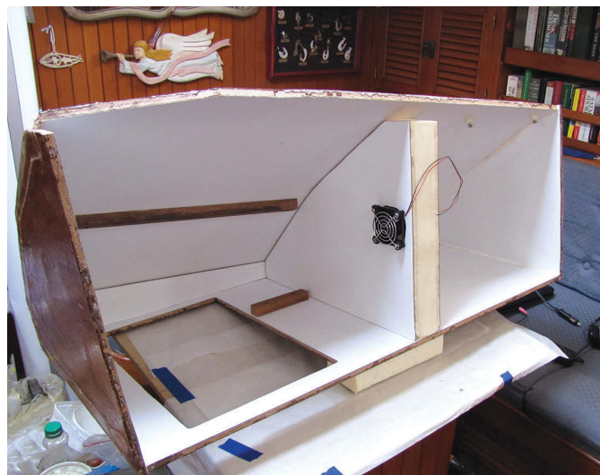
The insulation is two layers of 2.4-inch-thick polyurethane foam, at left. The inner box, at right, is lined with white laminate. David would place it inside the insulated cavern once he had fitted the divider, sealed all the inside corners, and installed the cold plate in the freezer.
