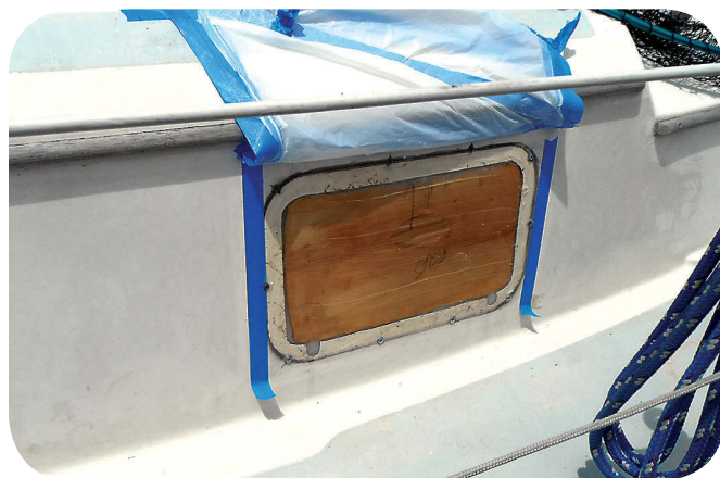
After coating the rabbets with epoxy, Dave screwed the plywood in place from the outside, using holes he’d pre-drilled for the purpose, at left. The kerfs, filled with epoxy, are visible in the plywood. The outside face of the plywood was flush with the cabin side, at right.
