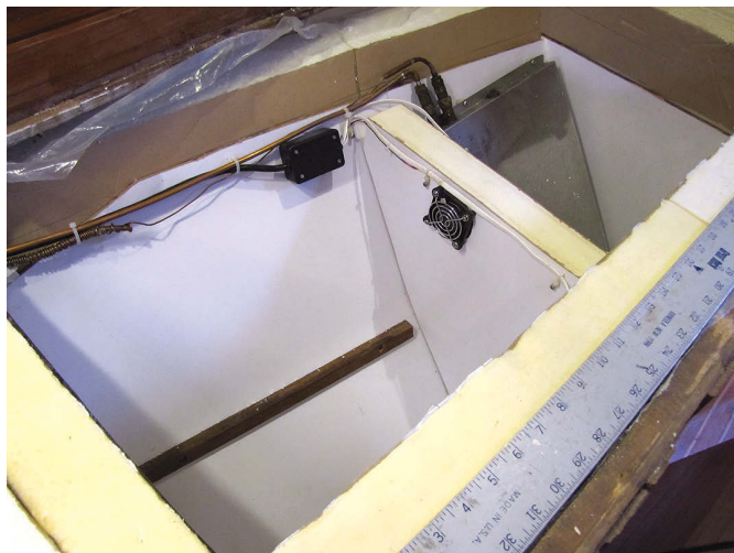
With the inner box installed, David hooked up the plumbing and wiring and performed a pressure check before adding the top.
