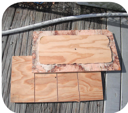
After removing a portlight and cleaning up the area, Dave cut a 1¼-inch-wide rabbet around the inside of the hole, at left, into which he would fit a plywood insert, center, with a matching rabbet to fit in the opening. He glued the plywood in place with epoxy, at right.
