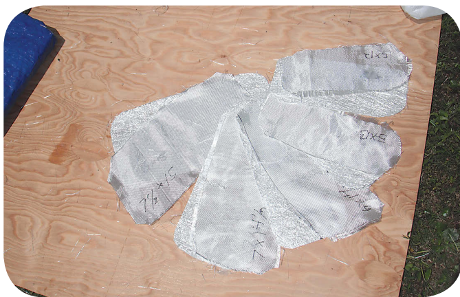
After rounding the square corners of the cut pieces, Dave laid them out so he could pick them up in the sequence — largest to smallest — in which he would use them, at left. Mat holds its shape well enough when wet that Dave could pre-wet it before placing it, at right.
