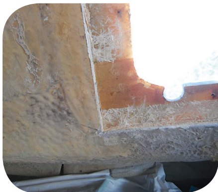
After removing a portlight and cleaning up the area, Dave cut a 1¼-inch-wide rabbet around the inside of the hole, at left, into which he would fit a plywood insert, center, with a matching rabbet to fit in the opening. He glued the plywood in place with epoxy, at right.
