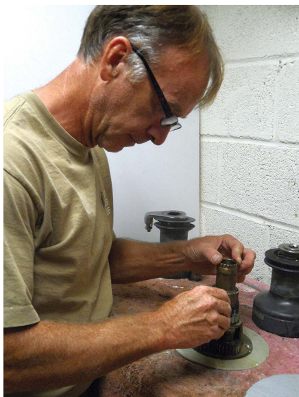
Drew cut the material for his backing plates out of a fiberglass bulkhead from a boat that was being sliced up for the dumpster, far left. Holding a Sharpie vertically, Drew made circles on the backing plate inside the holes in the winch base, near left. He drills \frac{1}{32} inch oversize to allow for alignment and measuring errors.
