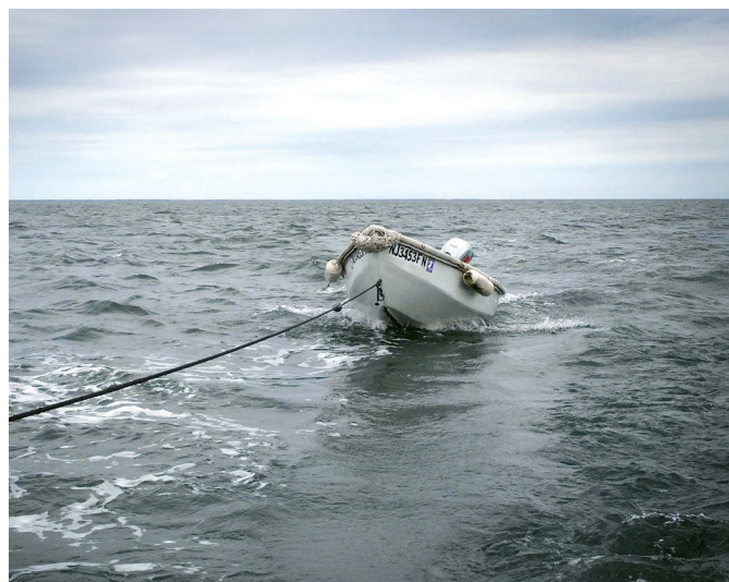
A wire strop ensures the outboard stays with the dinghy, at left. Cleats on each side serve many purposes, as does the rag. At 4 knots, the painter is entirely out of the water. At 5+ knots, at right, the dink follows as docile as a lamb with its bottom chine clear of the water.
