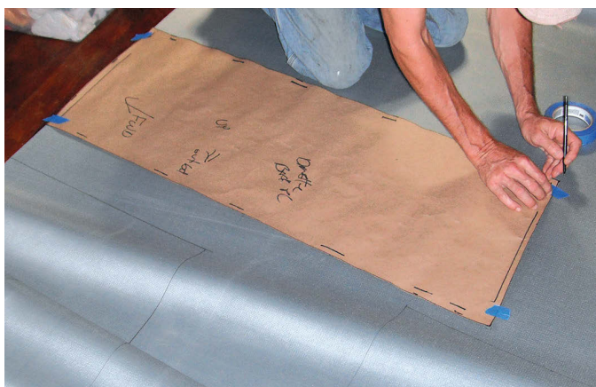
Dave and Connie laid out the patterns on the fabric in a way that left material for long lengths of boxing, above center. Dave laid the vinyl good side down so he could mark around the patterns on the back, at left, then connected the marks with a straightedge, at right,
