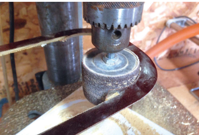
Art cut the inside edges by laying the blank on the saw table and carefully raising the saw blade, above left. He cut the inside corners with a hole saw, above right, and trimmed them with a drum sander, below left. The screen is glued in place with silicone, below right.
