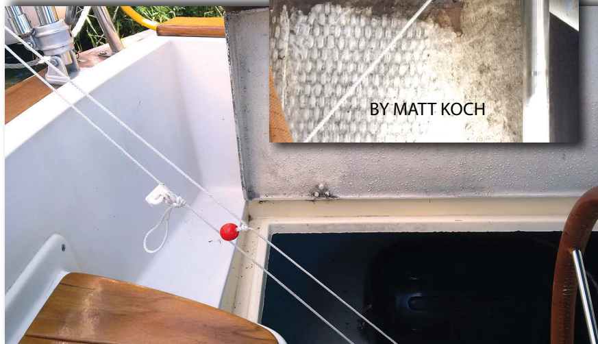
Ingenuity and a length of light line turned a broken gearshift cable into a hiccup instead of a cruise killer. Pull the sail slide for forward, the red ball for reverse.
