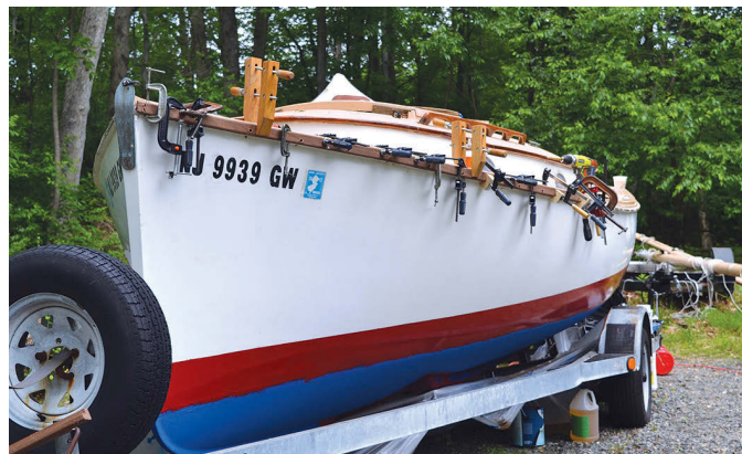
Before cutting the mast, George test-fit the tabernacle to avoid errors, above center. Joe Gerard and Bob Keppel, above left, set up the steaming tube for the mahogany strips that would become the rubrail. Installing the rubrail required the use of many clamps, above right.
