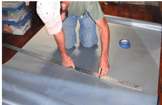
Dave and Connie laid out the patterns on the fabric in a way that left material for long lengths of boxing, above center. Dave laid the vinyl good side down so he could mark around the patterns on the back, at left, then connected the marks with a straightedge, at right,
