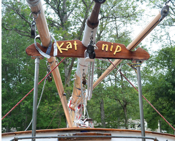
Boom gallows, decorated with the boat's name, are traditional and practical, as they stop the heavy boom from dropping into the cockpit.
