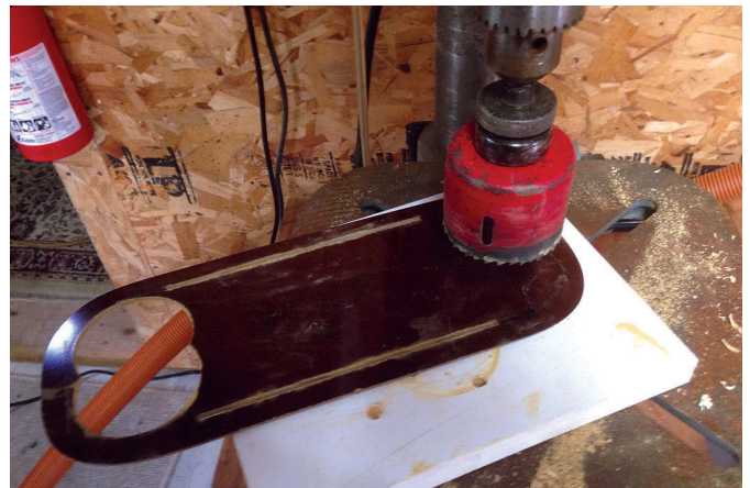
Art cut the inside edges by laying the blank on the saw table and carefully raising the saw blade, above left. He cut the inside corners with a hole saw, above right, and trimmed them with a drum sander, below left. The screen is glued in place with silicone, below right.
