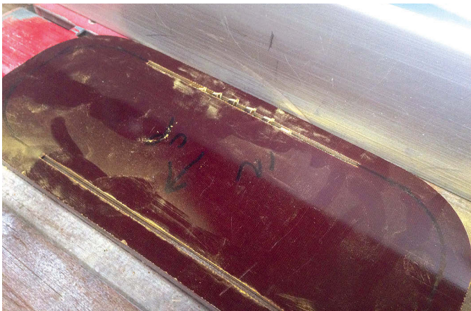
Art cut the inside edges by laying the blank on the saw table and carefully raising the saw blade, above left. He cut the inside corners with a hole saw, above right, and trimmed them with a drum sander, below left. The screen is glued in place with silicone, below right.
