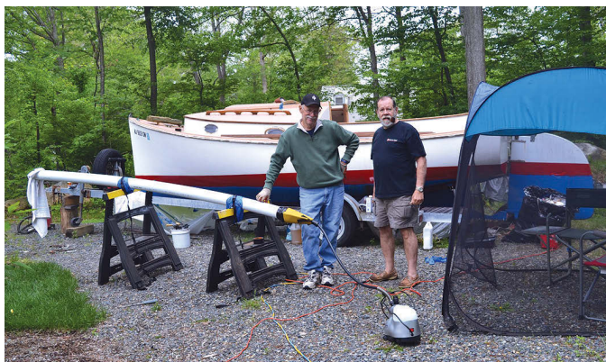
Before cutting the mast, George test-fit the tabernacle to avoid errors, above center. Joe Gerard and Bob Keppel, above left, set up the steaming tube for the mahogany strips that would become the rubrail. Installing the rubrail required the use of many clamps, above right.
