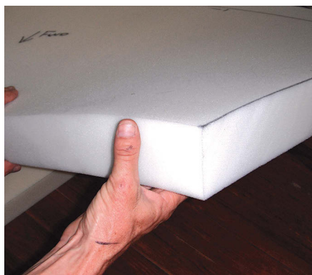
When cutting the foam, Dave was careful to hold the knife perpendicular to it, far left, and ended up with nice, crisp corners, at left.
