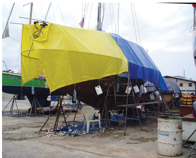
The water jugs weighing down Shirley's tarp look a bit makeshift, above, but they did their job when the wind blew. The extension created enough room for her to work on the entire hull, below.
