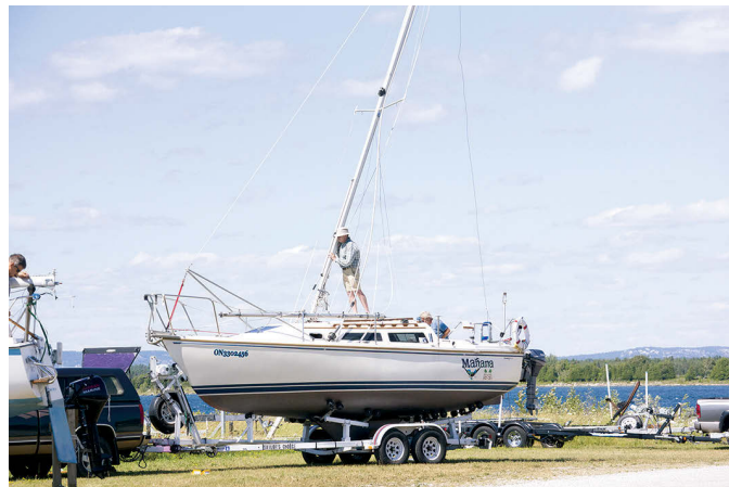
Due to its draft (2 feet 10 inches), the wing-keel version of the Catalina 25 often requires a trailer tongue extension to get the boat far enough down a typical ramp to float off the trailer, at left. Some mechanical advantage is needed when raising and lowering the mast. On Mañana , Bill Bennett uses the common arrangement of an A-frame and side-to-side bridles, at right.
