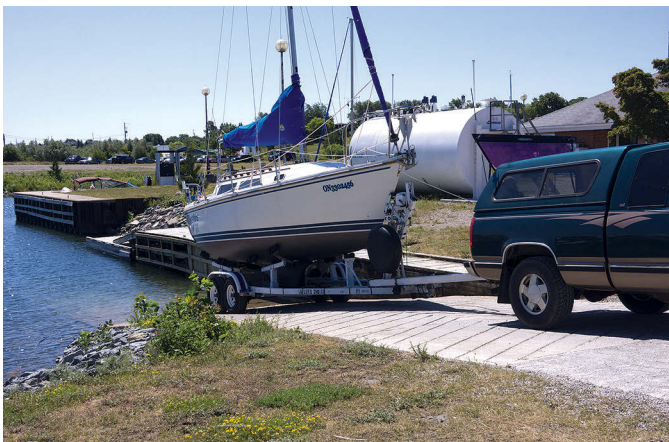
Due to its draft (2 feet 10 inches), the wing-keel version of the Catalina 25 often requires a trailer tongue extension to get the boat far enough down a typical ramp to float off the trailer, at left. Some mechanical advantage is needed when raising and lowering the mast. On Mañana , Bill Bennett uses the common arrangement of an A-frame and side-to-side bridles, at right.
