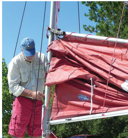
The tabernacle, at left, allows the mast to be quickly lowered, even for slipping under low bridges. Lazy-jacks tame the gaff when the sail is lowered, center. The gaff rig is easy to handle, at right, and the sail's two sets of reef points are needed when the breeze is up.
