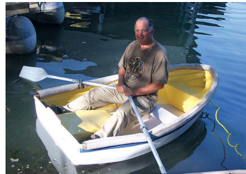
A friend made a floor for the dinghy, at left and above left, and a seat. After repairing the holes, Robert painted the boat inside and out and fitted a gunwale guard of wood, foam, and fire hose. The result is a serviceable rowboat with a new lease on life, at right.
