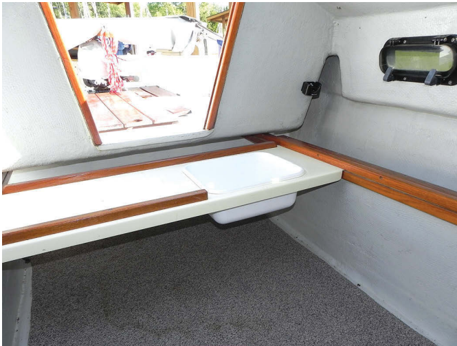
As interiors go, that in the Bay Hen 21 is spare, but the slide-out galley counter with a “sink,” at left, makes it more luxurious than the average tent. The bilgeboard trunks port and starboard define the main cabin, at right, and provide backrests for sitting athwartships.
