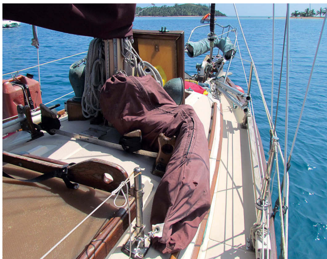
The trysail lives on deck hanked on to its own dedicated sail track and ready to hoist at a moment's notice, at left. When they need it, Ed and Ellen hoist the trysail directly from the bag, at right. The sheet is marked and pre-trimmed to prevent the sail from flogging wildly.
