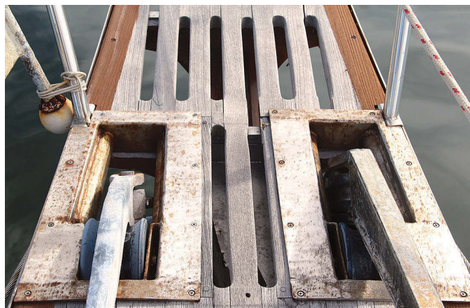
As well as making prodigious use of the sewing machine, Sandy, at left, stripped the exterior teak and recoated it with a teak oil sealer. The bowsprit housing for the anchor rollers was flawed, so Vic's friend Tom built a new, more robust one, at right, with Delrin rollers.
