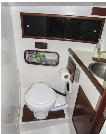
The head has room for a well-regarded Lavac manually operated vacuum toilet, sink, shower pan, and storage cubbies.
