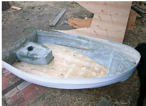
A friend made a floor for the dinghy, at left and above left, and a seat. After repairing the holes, Robert painted the boat inside and out and fitted a gunwale guard of wood, foam, and fire hose. The result is a serviceable rowboat with a new lease on life, at right.
