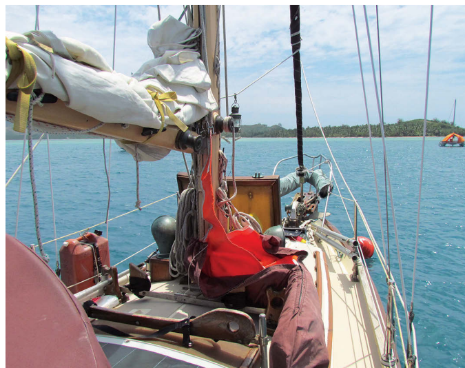
The trysail lives on deck hanked on to its own dedicated sail track and ready to hoist at a moment's notice, at left. When they need it, Ed and Ellen hoist the trysail directly from the bag, at right. The sheet is marked and pre-trimmed to prevent the sail from flogging wildly.
