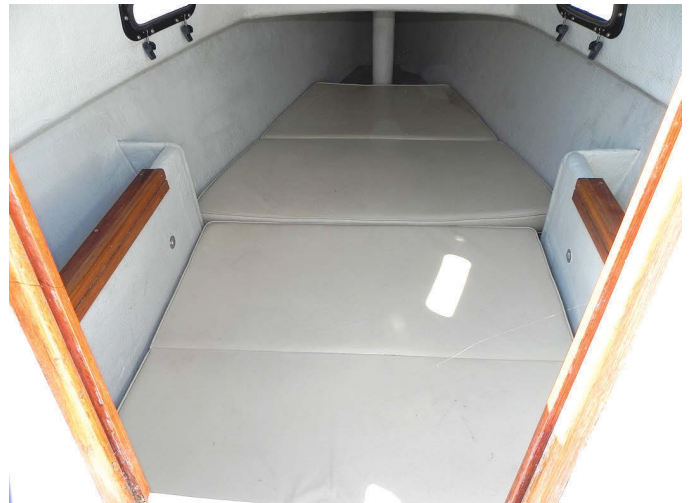
As interiors go, that in the Bay Hen 21 is spare, but the slide-out galley counter with a “sink,” at left, makes it more luxurious than the average tent. The bilgeboard trunks port and starboard define the main cabin, at right, and provide backrests for sitting athwartships.
