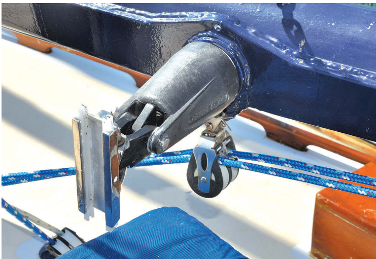
The gooseneck, at left, is a rather intricate affair as it has to allow the yard to rotate in several directions for sailing or stowing in a marina-friendly manner. Roger tested the furling system in his daughter's warehouse, at right, with a sail made from a plastic tarp.
