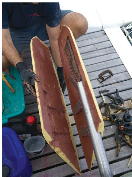
After adding a few layers of carbon fiber (to add stiffness below the stock) Evan applied glue to both halves of the core and fitted one side, at left, then the other, at right, to the stock.
