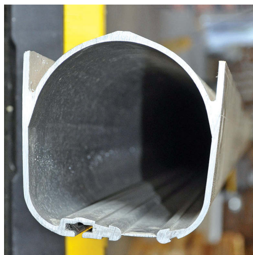
An in-yard roller-furling square sail is not a stock item at most sailmakers, so Roger had to improvise. He purchased a length of section for in-mast furling, at left, and trimmed it.
