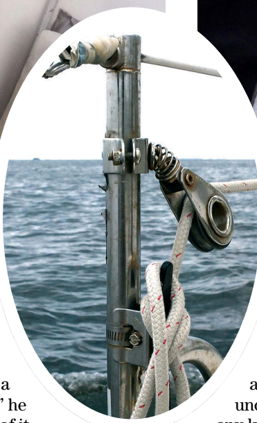
Cliff stows the downhaul line on a stanchion cleat at the cockpit, far left. The downhaul leads through stanchion blocks, inset, all the way to the bow pulpit. He clips it to the head of the sail with a snap shackle, above.
