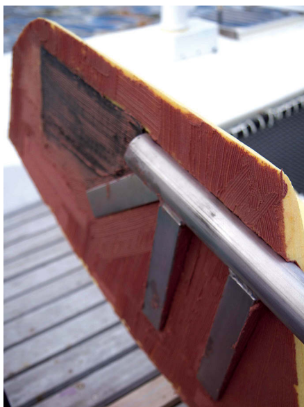
After adding a few layers of carbon fiber (to add stiffness below the stock) Evan applied glue to both halves of the core and fitted one side, at left, then the other, at right, to the stock.
