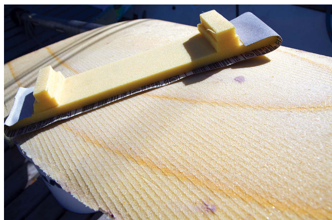
Clamping the rudder core halves together, at left, was a little delicate because the core could be crushed locally by too much pressure from the clamps. The machining process left tool marks on the rudder core, but these were easily removed with a longboard, at right.
