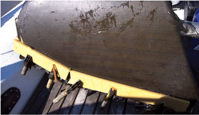
Peel ply laid over the final layer of fiberglass, at left, and removed after the resin has cured leaves the laminate with a smooth finish. Clamps and battens hold the trailing edges together helped by epoxy putty, visible as a brown line after the excess glass has been trimmed, at right.
