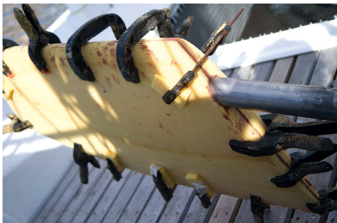
Clamping the rudder core halves together, at left, was a little delicate because the core could be crushed locally by too much pressure from the clamps. The machining process left tool marks on the rudder core, but these were easily removed with a longboard, at right.
