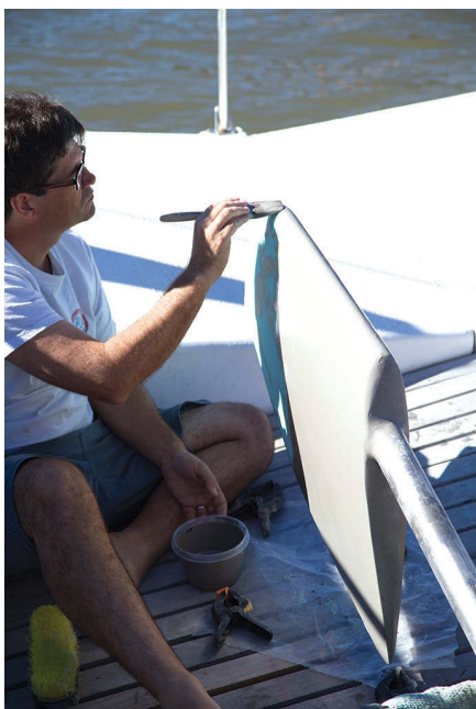
Evan gave the finished and faired rudder a coat of epoxy primer before the antifouling.
